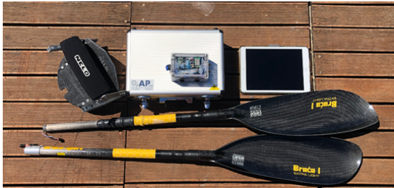
Figure 2: Shows the e-kayak system consisting of a master node, paddle, footrest and a tablet for data acquisition (APLab, Rome Italy, E-kayak).
