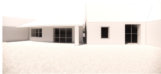
III.77. 40 cm glass gap between the Common House and the apartments
