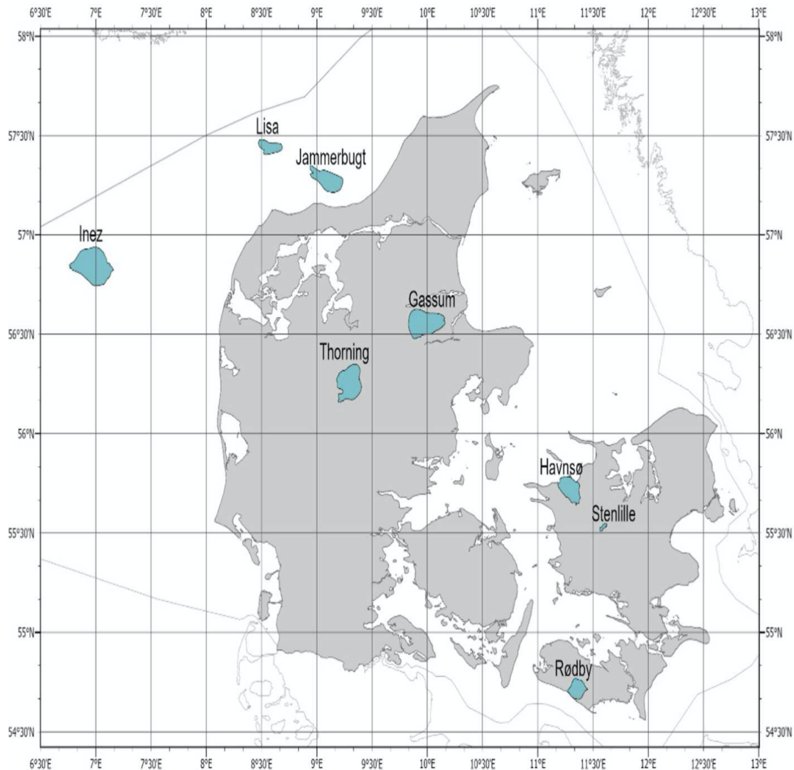
Figure 4.2. The areas where onshore and nearshore CO 2 storages possibly can be placed [Rambøll, 2022].
