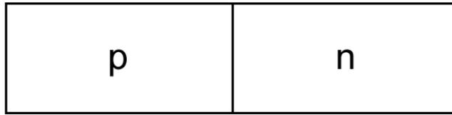
**Figure 6.1:** Illustration of a rectangular slab of a semiconductor consisting of p-type material to the left and n-type material to the right. The interface between the p- and n-type region is called a pn-junction. Inspired from [1, p. 309].
