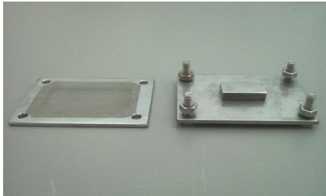
**Figure 9.2:** Illustrates the steel mesh to the left and the platform rack to the right on which the substrates are placed.
