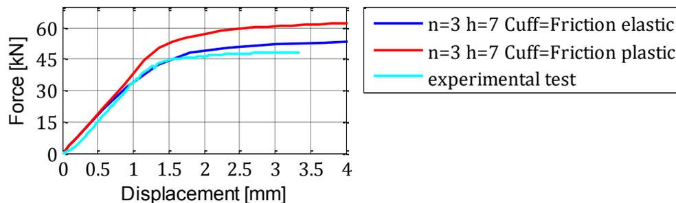
Figure 5-10: Force-displacement relation for 3 elements in the thickness and element length of 7 mm in square. The cuffs are modelled by friction with an elastic or plastic material model.
