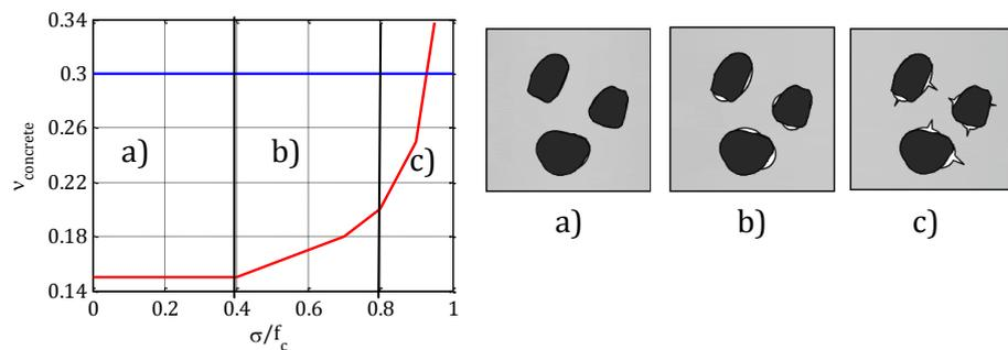
Figure 1-10: The development of Poisson's ratio for concrete vs. the normalized compressive stress and the micro-cracking: zone a) the initial pore volume, zone b) micro-cracking around the aggregates and zone c) micro-cracking in the cement paste. Source: figure 3.2-23 in [1.7]
