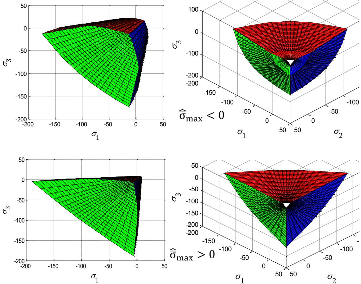
**Figure 4-8: The yield surface of the modified Lubliner in the 2D view (left) and in the deviatoric plane (right) for  $K=2/3$ . A triaxial compressive stress state ( $\nu$  is active) is shown in the upper plots, and  $\hat{\sigma}_{\max} > 0$  in the lower plots.**
