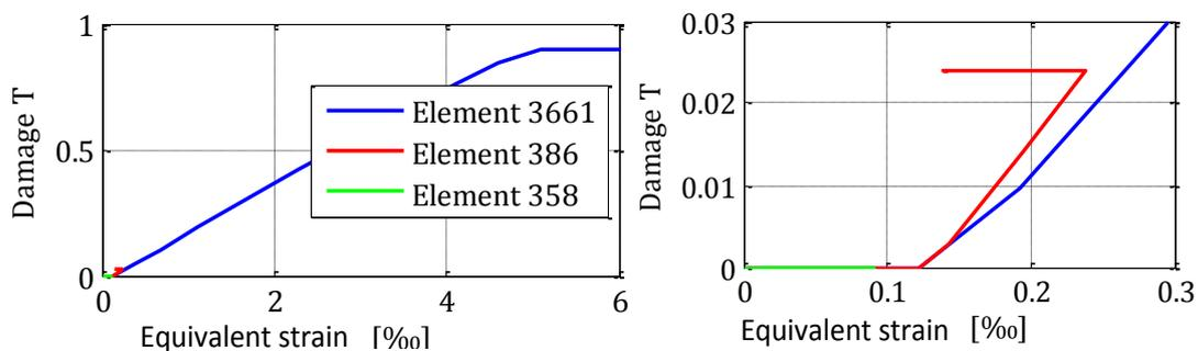
**Figure 4-16:** The corresponding tensile damage in the integration points of figure 4-15. In the zoom of the plot (right) it is seen, that the damage level is kept when the relaxation occurs.
