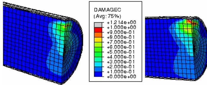
Figure 6-10: The compressive damage in the PCFT with LSC grout at the end of LS1 equal to a load level of 30 kN (left) and for a loading of 50 kN (right).
