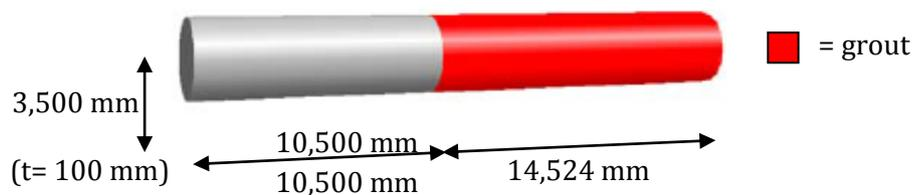
**Figure 1-29:** The geometry of the grouted leg in the Rambøll analysis. [1.16]
