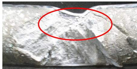
Figure 6-12: The failure in one of the PCFTs with LSC grout. The red marking illustrates the area with crushing in the grout.
