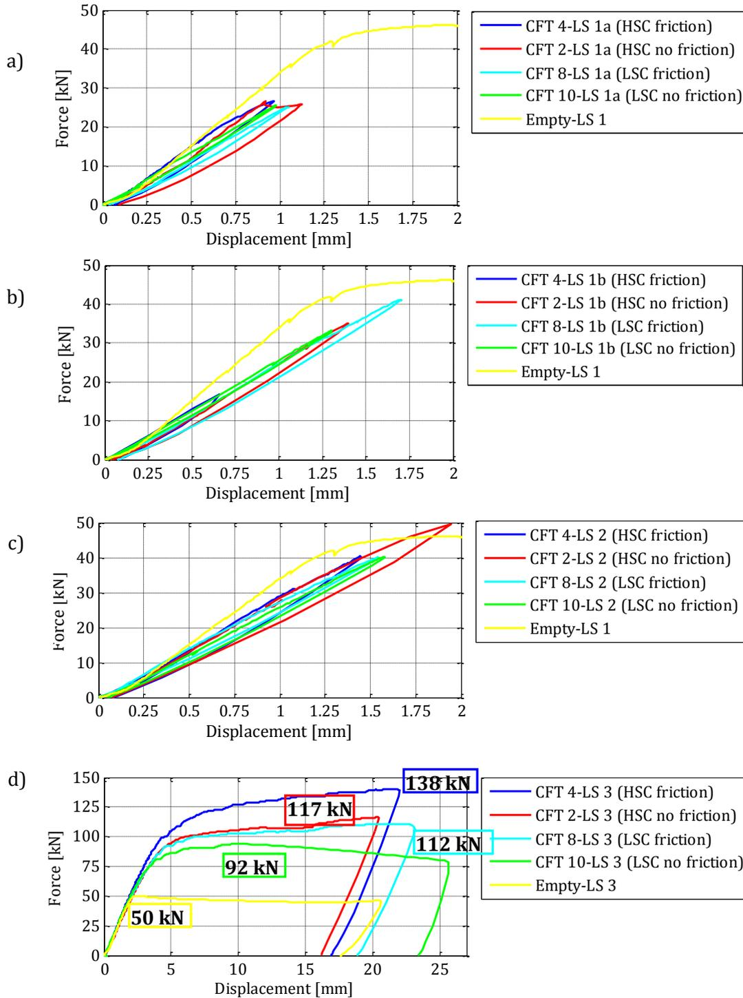
Figure 3-6: The force-displacement for CFT 2, 4, 8 and 10 in load step 1a, 1b, 2 and 3 (counted from the top). The peak loads is seen in d).
