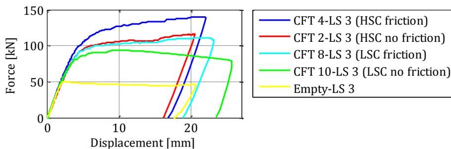
**Figure 7-7: The load deflection of the PCFTs determined by experiments.**
