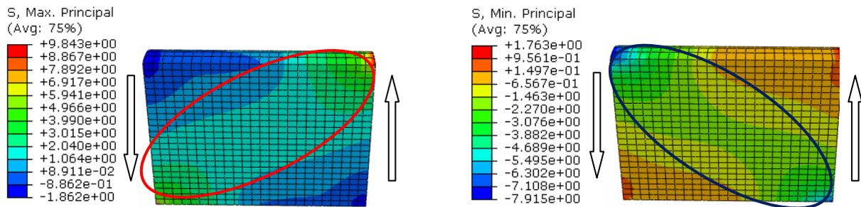
**Figure 1-23:** The maximal principal stresses (left) and the minimal principal stresses (right) in the grout core of a CFT with a shear span ratio of 1. The red marking shows the tensile stresses and the blue marking highlights the compressive stresses.
