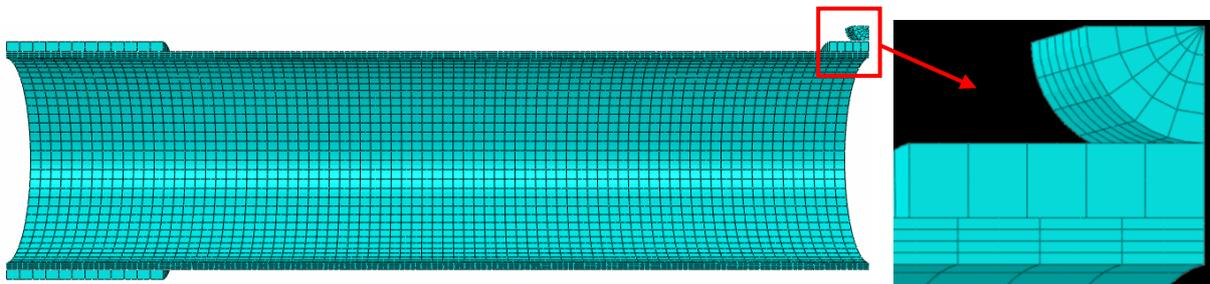
Figure 5-4: The mesh of the model (left) and a zoom of the press roll and plate (right).
