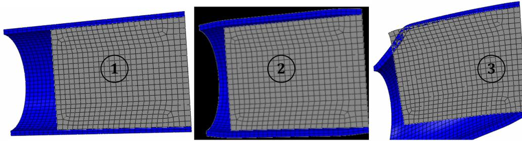
**Figure 1-28:** A composite element fixed in the end with the grout and the load applied to the steel tube in the other end. The element is subjected to (1) no load, (2) axial load on the steel section and (3) the axial load from (2) combined with a transverse load on the steel section. Contact is re-established due to transverse the loading. The deformations are scaled with a factor 25 in order to visualize the effect. The contact surface is modelled as Coulomb friction.
