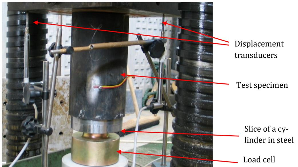
Figure 2-8: Test setup. Load cell, steel slice and test specimen in the test machine. The displacement is measured in the diagonal corners of the press plate.
