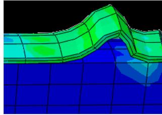
Figure 1-20: Zoom of the CFT subjected to pure bending. The steel buckles in the compressive zone.
