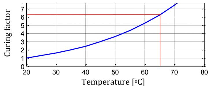
Figure 2-6: Curing factor for  $T > 20$  °C [2.2].
