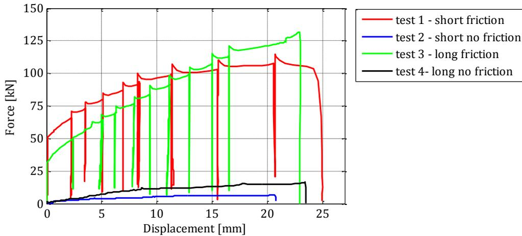
**Figure 2-9: Force-displacement for the four test specimens.**
