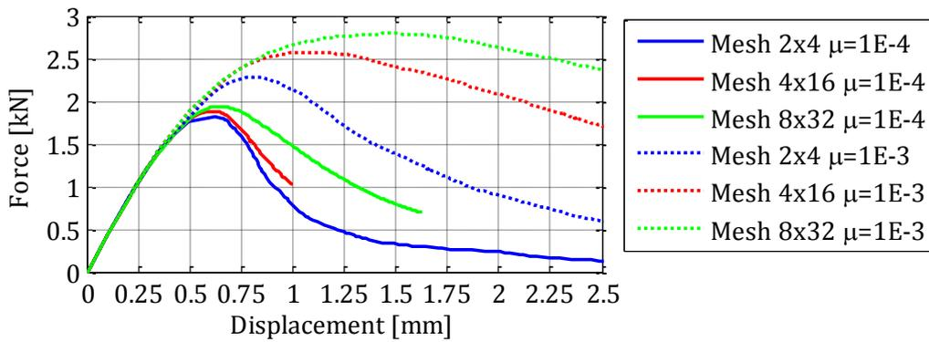
Figure 4-26: The force-displacement relation for the three meshes to  $\mu=1E-3$  and  $\mu=1E-4$ .
