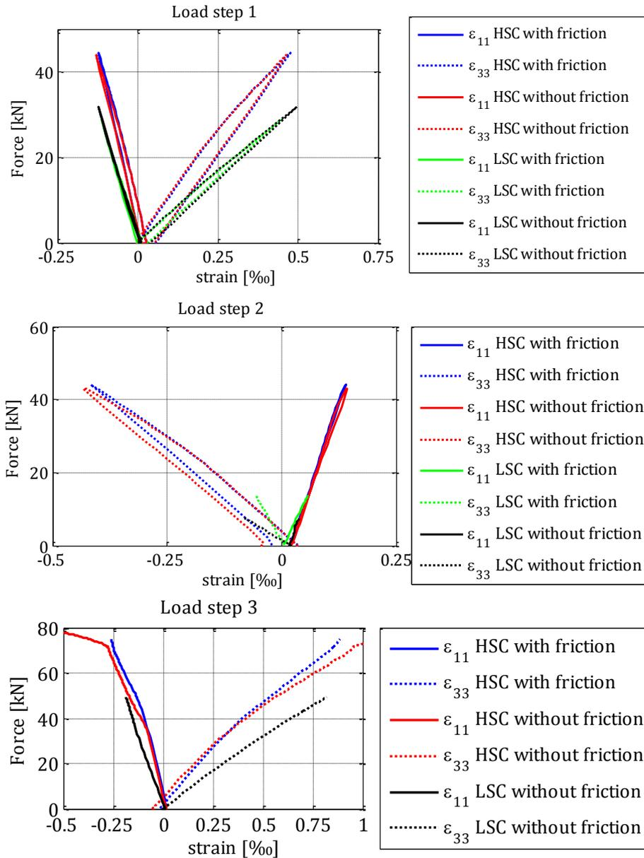
**Figure 6-6: The load-strain relations for LS 1-3 counted from the top.**
