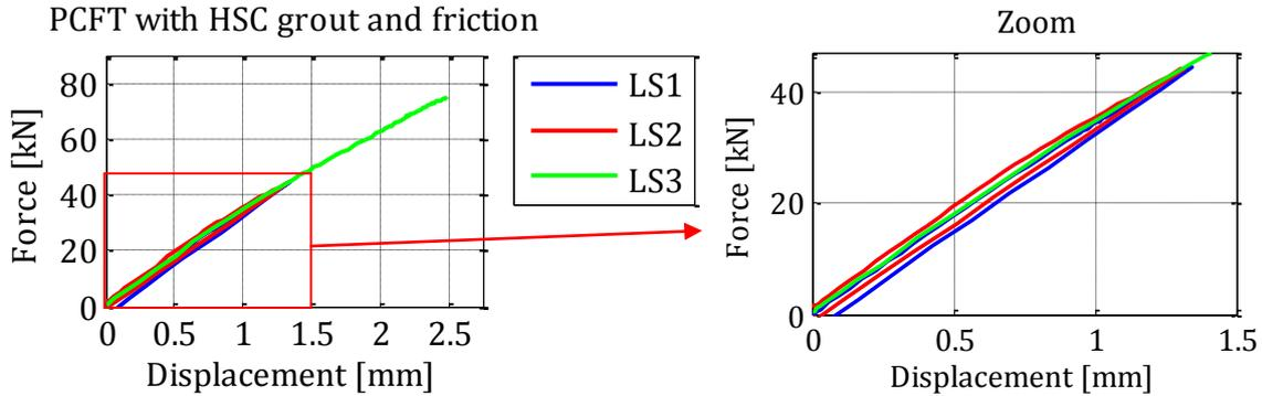
**Figure 5-20:** The force displacement relation for load step 1-3 for the PCFT with HSC grout and friction (left) and a zoom in the range of LS1 and LS2 (right),
