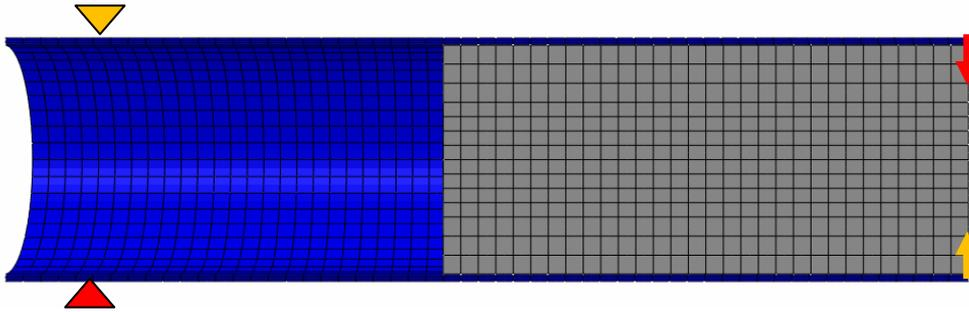
Figure 5-17: The load and support location in LS 1-3. The red pair is for LS 1 and LS 3, the orange pair is for LS 2.
