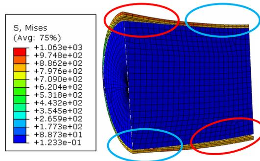
**Figure 1-6:** The binding mechanism for a CFT exposed to pure bending. Red circles indicate areas with slip between the contact surfaces and blue circles area where the contact surfaces are pressed together. The deformation is up-scaled by a factor 100.
