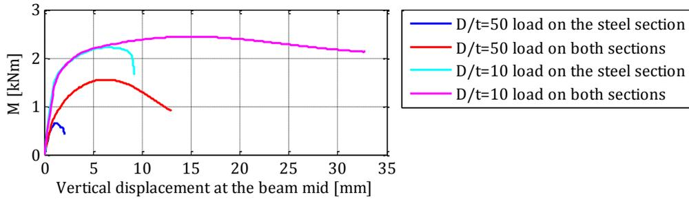
Figure 1-19: The bending moment as a function of the vertical deflection at the middle of the CFT.
