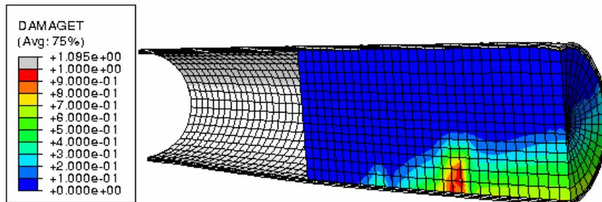
Figure 6-11: The tensile damage in the PCFT with LSC grout and no friction.
