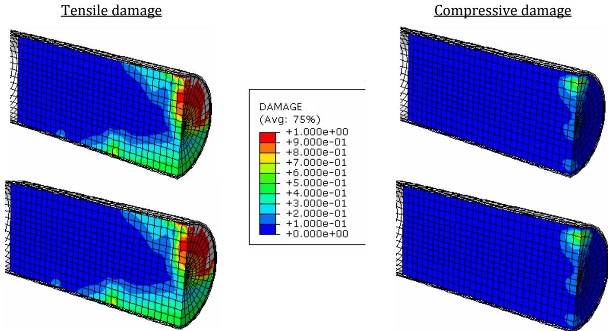
Figure 5-25: The tensile (left) and compressive (right) damage distribution in the grout core of PCFT with LSC grout without friction at the end of load step 1 (top) and when the analysis is aborted in LS 2 (bottom).
