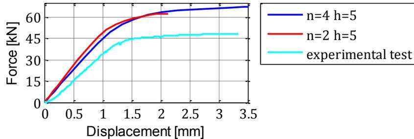
Figure 5-8: Force-displacement relation for 2 and 4 elements in the thickness and element length of 5 mm in square.
