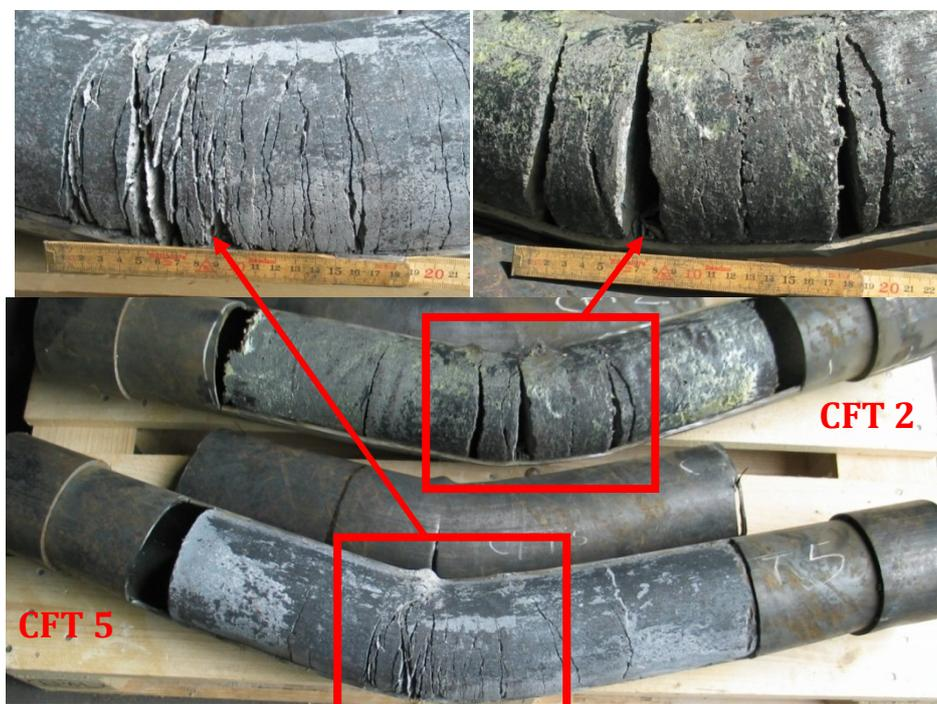
Figure 3-19: The crack in the grout for CFT 2 and CFT 5. A part of the steel tubes has been cut off in order to inspect the grout core.
