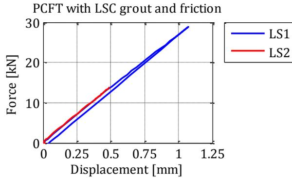
Figure 5-24: The force displacement of LS1 and 2 for the PCFT with LSC grout and friction.
