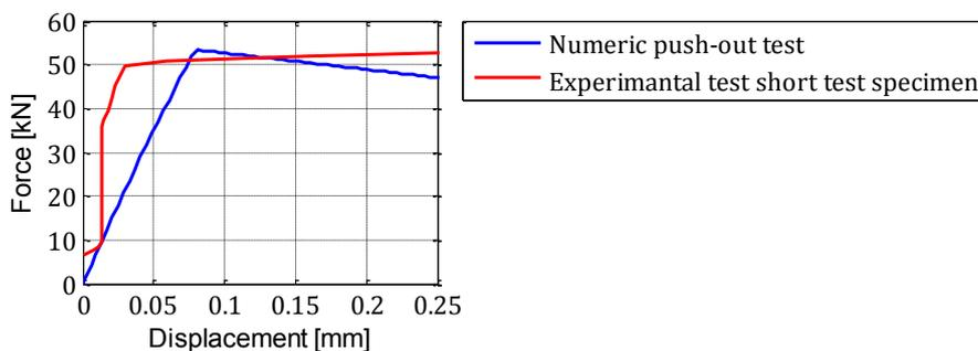
Figure 5-19: The results of the push-out tests. The experimental test is a part of the force-displacement relation for the short test specimen described in section 2.4
