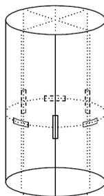
**Figure 2-5: The setup for determination of  $E_c$  and  $\nu_c$ .**
