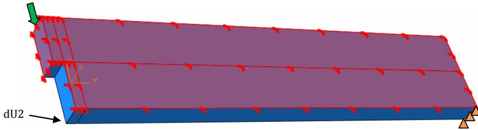
Figure 4-25: The boundary conditions. The red surfaces indicates plane of symmetry. The beam end is restricted in displacements in the Y-direction visualized by the triangles. The load is applied as a displacement of the mid beam on the line in the top of the cut face.
