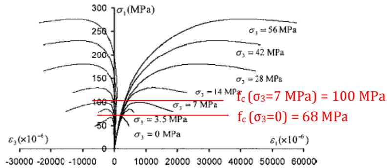
**Figure 1-11: The axial stress vs. axial strain (positive part of the axis) and hoop strain (left part of the axis) for various confining stresses on a concrete cylinder. The results are from experimental tests. The concrete used has a uniaxial compressive strength,  $f_{c0}$ , = 68 MPa. [1.8]**
