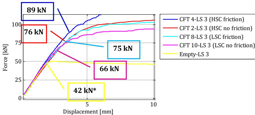
**Figure 3-11: Zoom of figure 4 15 d), and the load where the linear force-displacement relations (elastic range) ends. \*= in load step 1 yielding in the empty steel tube was reached at 42 kN according to figure 3-6 d), and by reloading the yielding force is 49 kN.**
