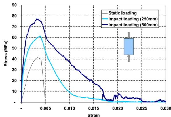
**Figure 4-5:** The influence of loading rate on the stress-strain relation in plain concrete. The impact loading is caused by a load hammer dropped at 250 mm (light blue curve) or 500 mm (dark blue curve). The static load was applied as a displacement controlled loading (12.7 mm pr. minute) [4.3].
