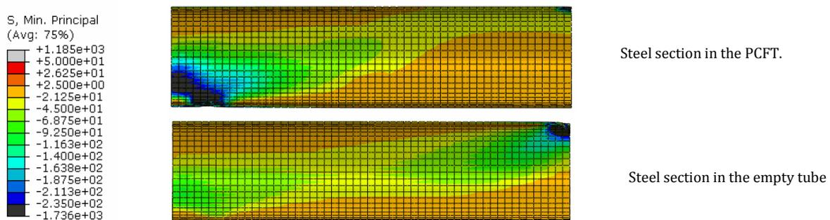
**Figure 3-9: The min. principal stress distribution in the steel section of the empty tube (lower) and the PCFT (upper). The load is applied at the stress concentration in upper right corner.**
