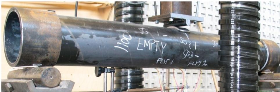
Figure 5-1: The empty steel tube in the test setup
