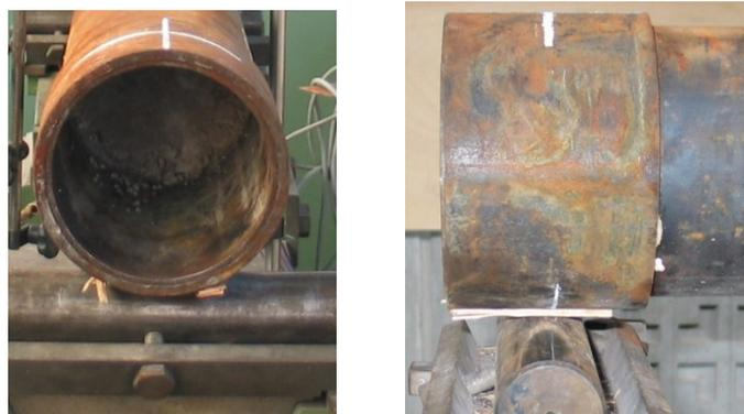
Figure 3-4: Strips of plywood placed on each side of the reinforcement cuff to prevent the tube from rolling during the test.
