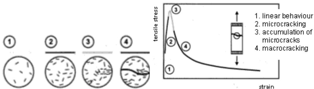
Figure 4-2: The crack evolution in relation to the tensile stress-strain relations. [4.1]
