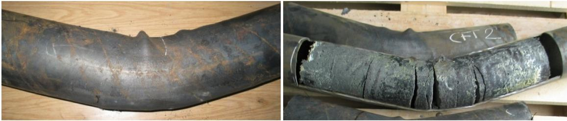
**Figure 1-30: Failure mechanism in the steel section (left) and the grout section (right) of a PCFT test specimen.**
