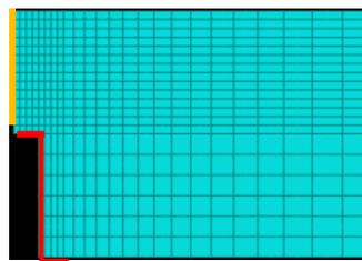
**Figure 4-24: The mesh is controlled by the marked lines.**
