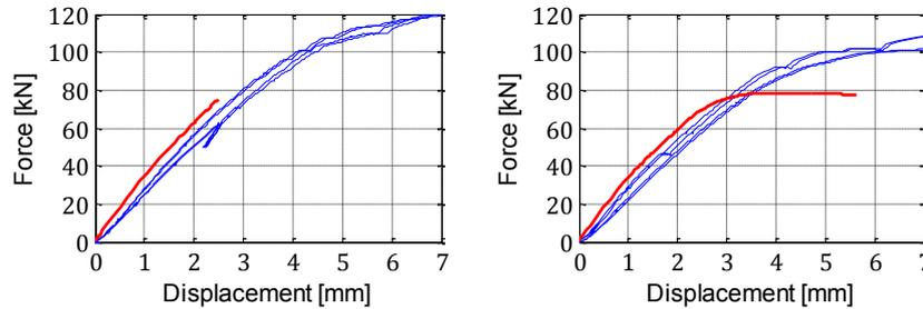
**Figure 7-6: The load-deflection relations for a PCFT with HSC grout with (left) and without (right) friction. The red curve is the numeric result; the blue curves are the experimental results.**
