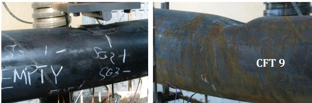
Figure 3-16: The plastic deformation where the load is applied. Left: Empty. Right: CFT 9 (LSC).
