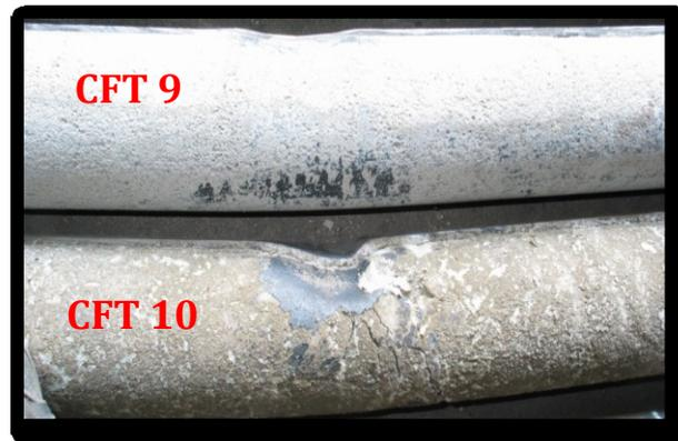
Figure 3-18: The grout core in CFT 9 (LSC non-greased) and CFT10 (greased). No visible cracks.
