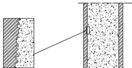
**Figure 1-5: Micro interlocking due to surface irregularities.**
