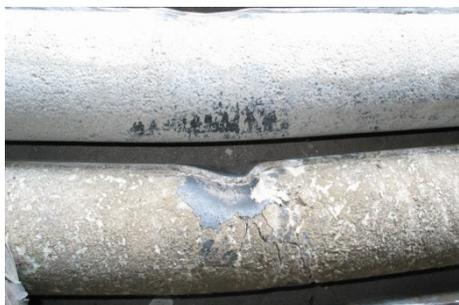
Figure 6-13: the grout cores of two PCFT's with LSC grout one non-greased (top) and one greased (bottom).
