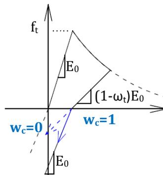
**Figure 4-14: The influence of the weights in the uniaxial load directions (blue vectors). The unbroken vector is the default directions meaning that a crack does not influence the ability to transfer compressive stresses.**
