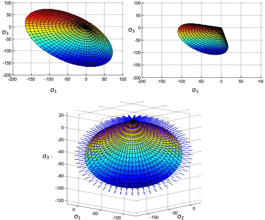
**Figure 4-11:** The plastic potential plotted in the principal stress space. The influence of the angle of dilatation is shown for the plastic potential in the  $\sigma_1$ -  $\sigma_2$  plane for  $\psi=15^\circ$  (top, left) and  $\psi=45^\circ$  (top right and bottom). The vectors in the lower plot indicate  $dg/d\sigma$ .
