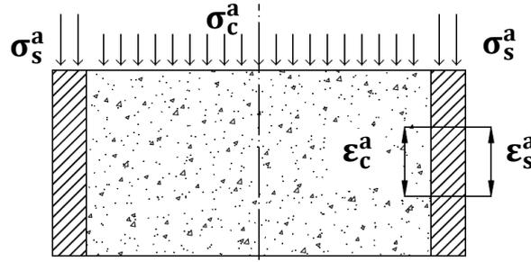
Figure 1-8: The axial strains in steel and grout are of equal size, when the load is applied to the entire CFT section.
