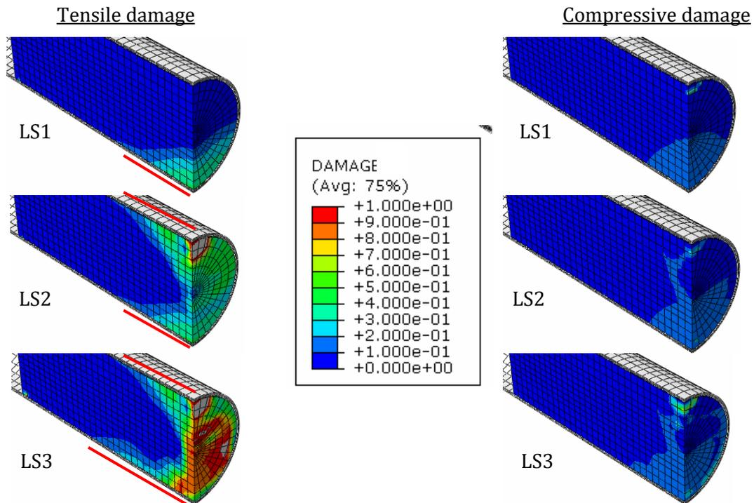
**Figure 5-21:** The tensile (left) and compressive (right) damage in the grout of the PCFT with HSC grout with friction at the end of load step 1 (top) to 3 (bottom). The red lines indicate the area the damage is smeared to.
