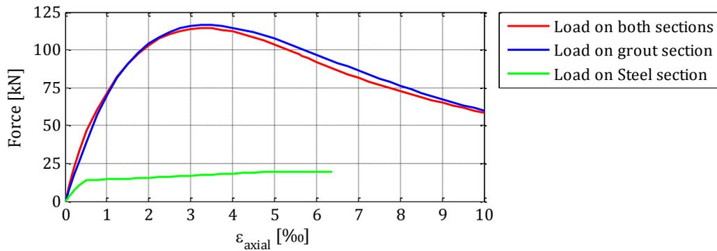
**Figure 1-3: The influence of the loading. Force as function of axial strain. [1.17]**
