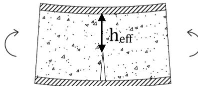
**Figure 1-16: Cracking in the grout reduces the effective height of the grout section.**
