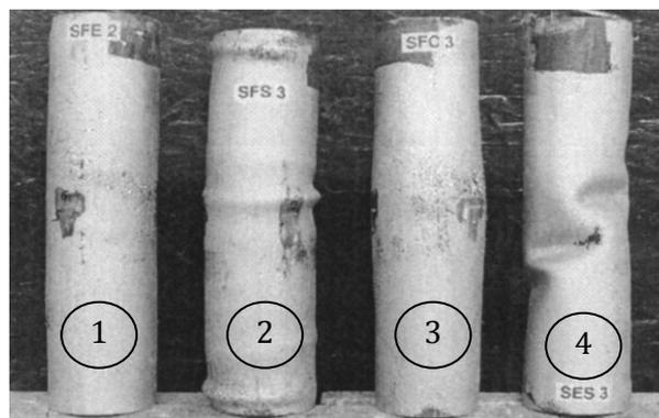
**Figure 1-24:** Failure mode in CFT's exposed to an axial concentric compressive load. The load has been applied to (1) the entire composite cross section, (2) the steel section and (3) the grout section. An empty reference tube (4) is seen to the right in the figure [1.10].
