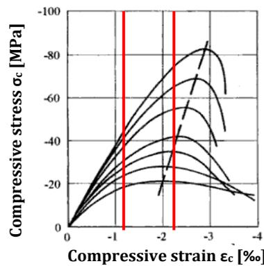
Figure 1-9: The compressive stress-strain relation. The evolution of the uniaxial compressive strength as a function of the ultimate strain,  $f_{c0}(\epsilon_u)$ , is visualized with the dashed line. The red lines marks the yield strain for normal structural steel S235-S460 [1.6].
