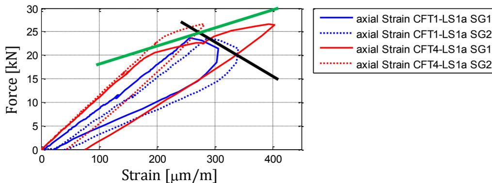
**Figure 3-14:** Force vs. Strain for CFT 1 and CFT 4 in load step 1a. The black and green lines (average of strain gauge 1 and 2) indicate the development of the stiffness after the grout is cracked. In CFT 1 =blue (greased tubes) the slope is descending while the slope in CFT4 (non-greased) increases.
