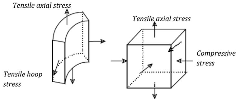
**Figure 1-15: Stress distribution in the steel tube and the grout core in the CFT axially loaded in tension.**
