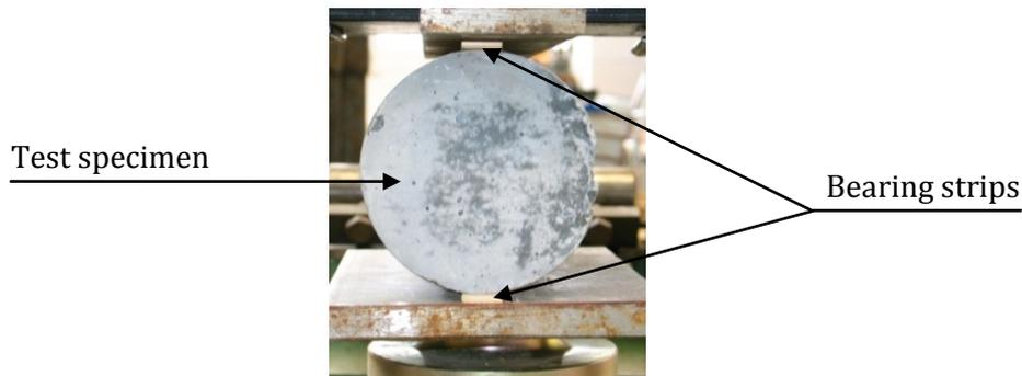
**Figure 2-2: The setup for the Brazilian test.**
