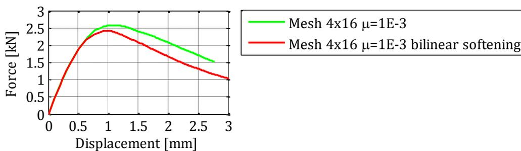
**Figure 4-29: The force-displacement relation for mesh 4x16 with the linear and the bi-linear softening**
