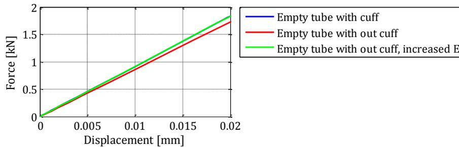
Figure 7-2: The force-displacement relations for numeric models with and without the reinforcement cuff.
