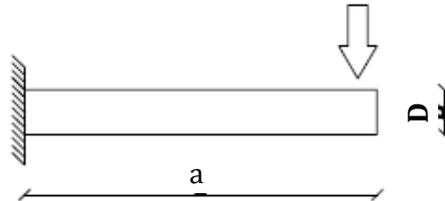
Figure 1-21: The shear span for a cantilever CFT beam subjected to a transverse loading.
