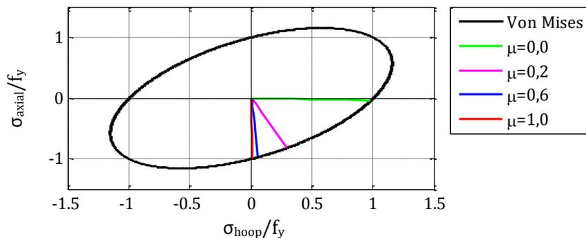
**Figure 1-13: The distribution of normalized hoop - and axial stress for various coefficients of friction. Load applied to the grout section [1.17].**
