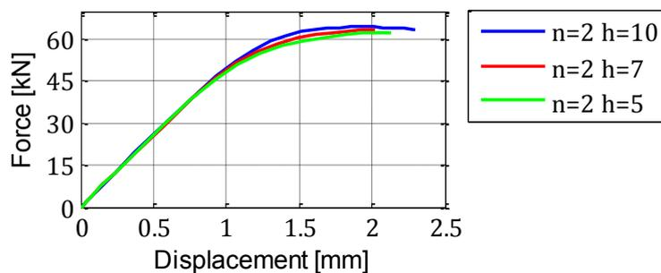
Figure 5-7: Force-displacement relation for 2 elements in the thickness and element length of 5, 7 and 10 mm in square.
