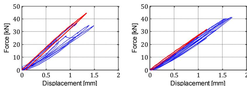
**Figure 7-5: The load-deflection relations for a PCFT with HSC grout (left) and with LSC grout (right). The red curve is the numeric result; the blue curves are the experimental results.**
