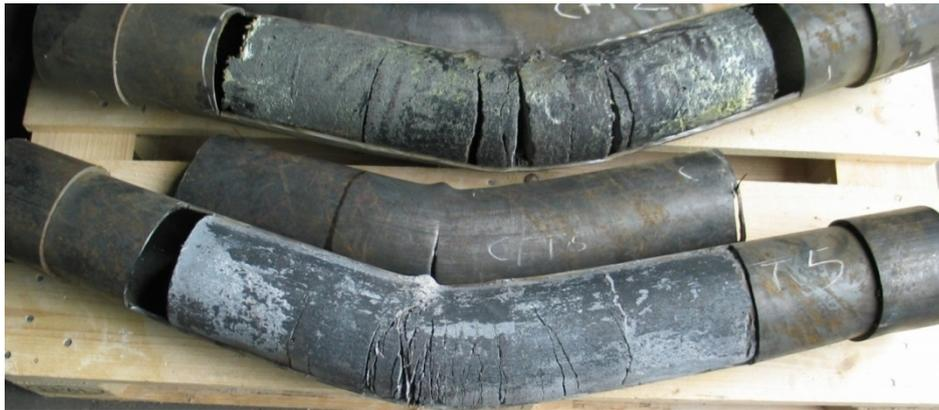
Figure 6-9: The crack pattern in the PCFT with HSC grout with (bottom) and without (top) friction determined by experiments.
