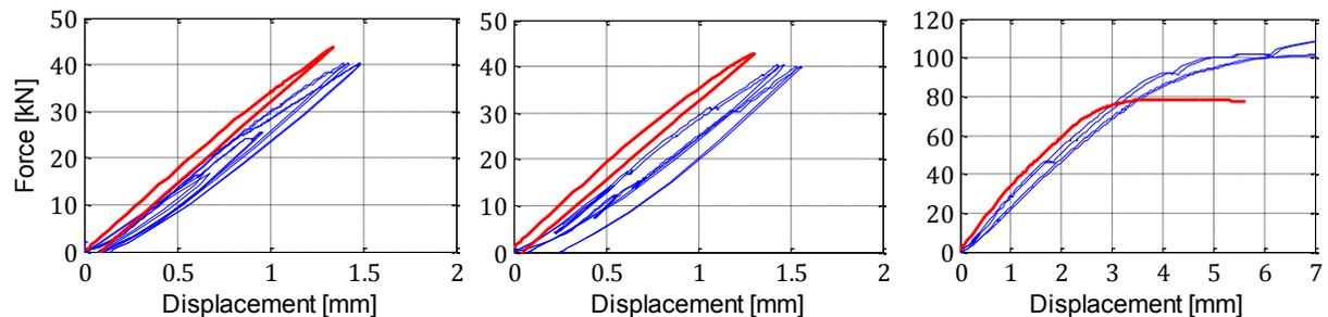
Figure 6-3: LS 1-3 for PCFT with LSC grout friction. The blue curves are the force-displacement of CFT 7-9.
