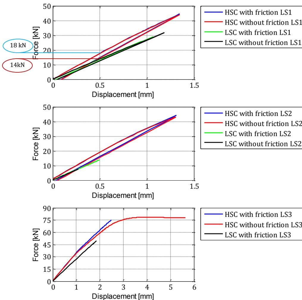
Figure 6-1: The load displacement relation of the numeric tests in LS 1-3 counted from the top.
