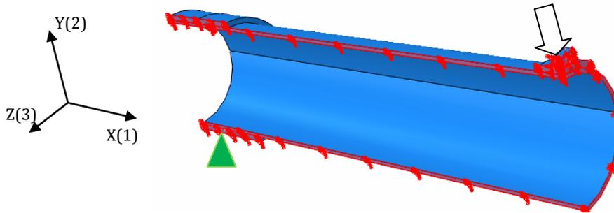
**Figure 5-5: The boundary conditions. The symmetry planes are marked with red. The green triangle visualizes the support - the node is restricted in displacements in the Y-direction. The load is applied the top cut face of the press roll as a displacement in Y.**
