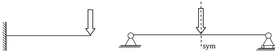
Figure 3-1: The reduced static system for the legs of the platform.
