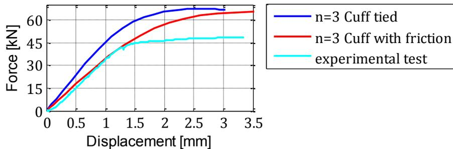
Figure 5-9: Force-displacement relation for 3 elements in the thickness and element length of 10 mm in square with the cuff tied or modelled by friction.
