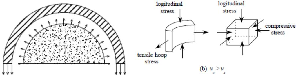
**Figure 1-12: Hoop stresses in the steel tube caused by the transverse contraction for an axial load on the grout section (left). This situation occurs if no shear stress can be transferred in the contact surface (frictionless) or if Poisson's ratio for the grout exceeds the one for steel (right). The source for the figure to the right: [1.9].**
