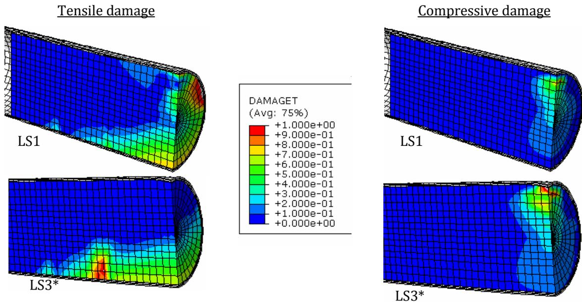
Figure 5-27: The tensile (left) and compressive (right) damage distribution in the grout core of PCFT with LSC grout without friction. The upper plots are at the end of load step 1, the lower plots are for LS3\* equal to the extended LS1.
