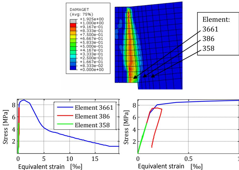
**Figure 4-15:** The stress-strain relation in a integration point of three elements in or near the crack. Element 3661 is located in the notch, 386 just outside the notch. Element 358 is neighbouring 386. A zoom (right) shows how element 358 relaxes when the damage is gathered in 3661.  $f_t$  in the model is 7.9 MPa.
