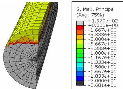
**Figure 1-14: The maximal principal stress visualizes the zone of confinement in the grout core subjected to pure bending.**
