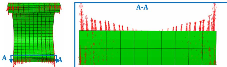
Figure 1-22: The hoop stress in the steel tube over the shear span.
