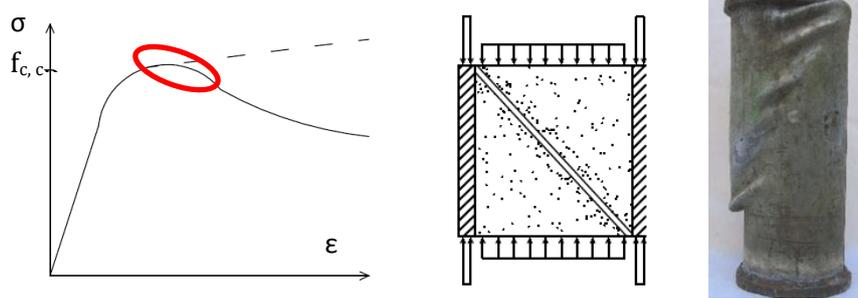
Figure 1-25: The shear failure in the grout core. When the confined compressive strength  $f_{c,c}$  has been reached- the red area on the stress-strain relation (left) and the steel is yielding, the shear failure evolves as visualized in the principle sketch (middle). The shear failure is obvious in the CFT (right).
