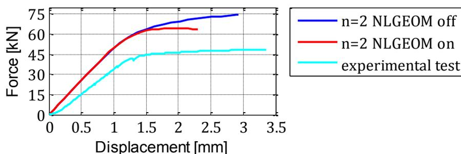
Figure 5-11: Force-displacement relation for 2 elements in the thickness and element length of 10 mm in square with and without nonlinear geometry activated. The analysis is carried out with tied cuffs.
