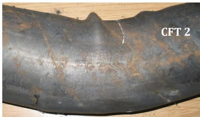
Figure 3-17: The outward buckling of CFT 2.
