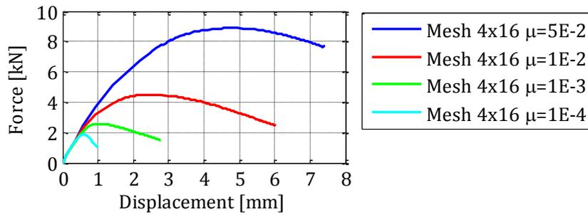
**Figure 4-27: The force displacement relation for different values of the viscosity parameter**
