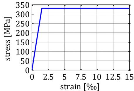
Figure 5-3: The stress-strain relation. The modulus of elasticity is 210 GPa, and  $f_y = 328$  MPa.
