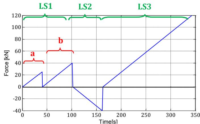
**Figure 3-5: The force amplitude in the load case used for the main test program. Negative amplitude means that the test specimen has been rolled 180 degrees about the axial axis.**
