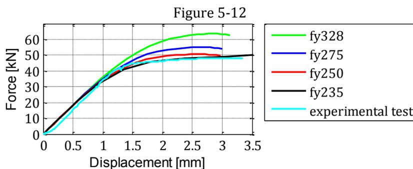
Figure 5-12: Force-displacement relation for 3 elements in the thickness and element length of 10 mm in square for different yield stresses. In the analysis for  $f_y = 235$  MPa is NLGEOM deactivated, and the cuff is modelled with friction.
