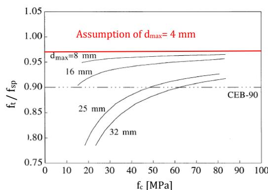
Figure 2-3: Ratio of the tensile strength to the splitting tensile strength compared to the proposal of [2.5] (the line CEB-90) for different maximum aggregate size,  $d_{max}$  [2.6]. The red line is an assumption for  $d_{max}=4$  mm.
