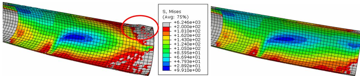
**Figure 6-14:** The steel tube of the PCFT with HSC grout without friction. The deformation is scaled by a factor 10. The red marking indicated the area with buckling. The deflection is 5.5 mm to the left and 2.5 mm to the right. The grey areas indicate yielding in the steel.<sup>7</sup>
