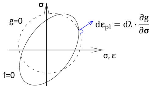
Figure 4-10: The plastic strain increment normal to the plastic potential,  $g=0$ , and the yield surface,  $f=0$ .
