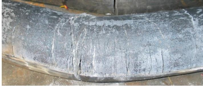
**Figure 4-3:** The cracking of concrete in the tensile zone of a PCFT. The PCFT is tested in 3-point bending with a shear span close to 4 resulting in a failure mechanism as in pure bending.
