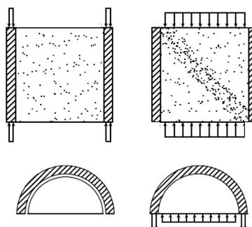
**Figure 1-7:** On top: Load applied to the steel section (left) and the grout section (right). Below: The consequences a) separation b) passive confinement of the grout core.
