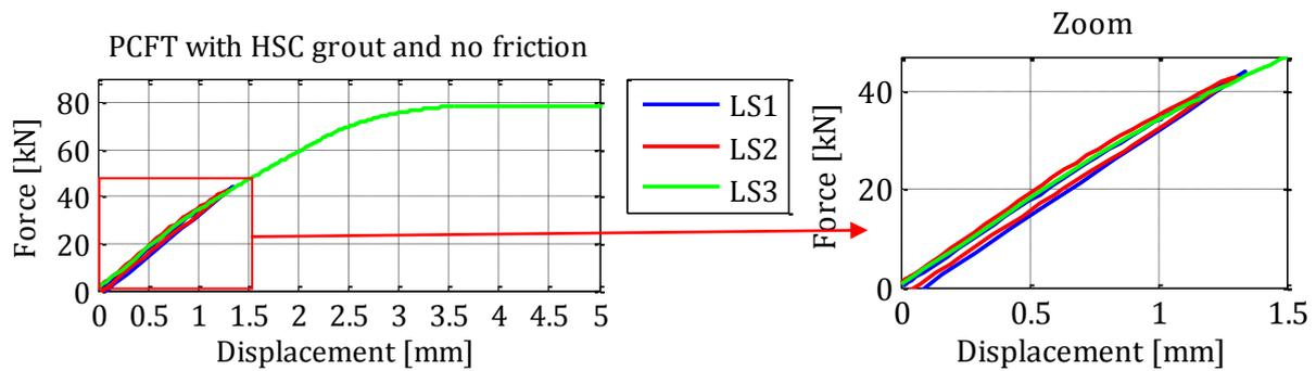
Figure 5-22: The force displacement relation for load step 1-3 for the PCFT with HSC grout and without friction (left) and a zoom in the range of LS1 and LS2 (right).
