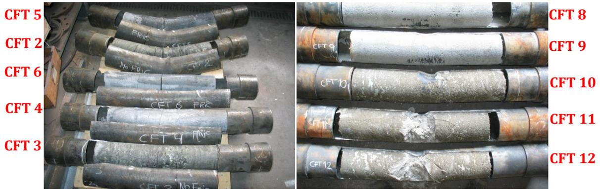
Figure 3-15: The PCFT prepared for inspection of the grout core. Left: CFT 2-6. Right: CFT 8-12.
