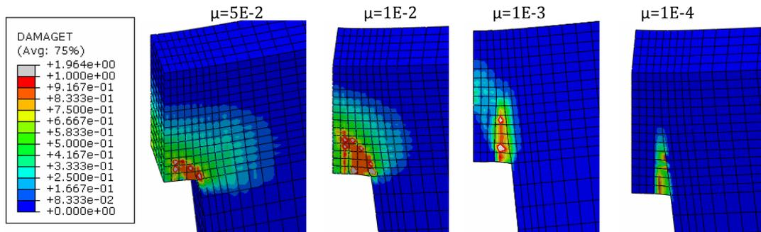
**Figure 4-28: The tensile damage in the notch for mesh 4x16 for  $\mu=5E-2$  to  $\mu=1E-4$  counted from left.**
