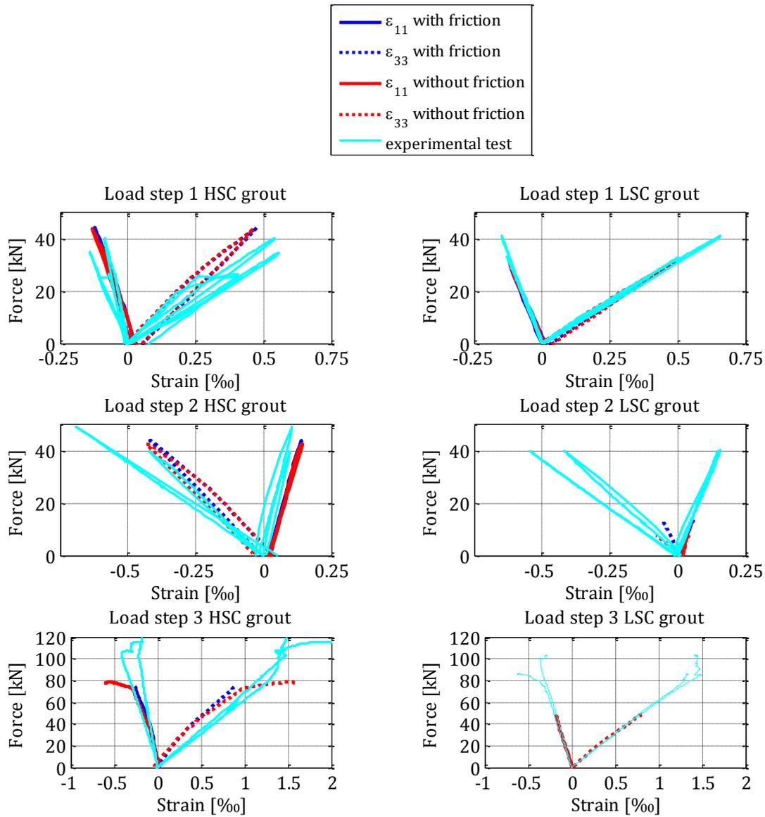
Figure 6-7: The force-strain relations for the numeric and experimental tests for PCFT with HSC grout (left) and LSC grout (right) at LS 1-3 counted from the top. The blue lines are for test specimens with friction, and the red lines for test specimens without friction. Dotted lines are hoop strains and unbroken lines are axial strains. The cyan curves are representative samples of the experimental test results.
