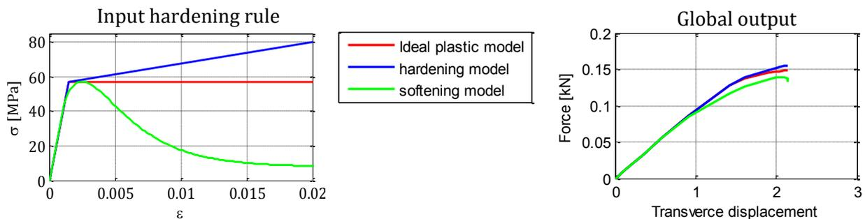
Figure 4-13: Three different hardening models, an linear elastic-ideal plastic model, a bi-linear plastic hardening model and a softening model (left) . The influence on the global load-displacement relation at the tip of the beam is seen to the right.
