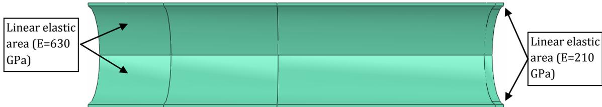
**Figure 5-13: The simplified model with areas modelled linear elastic materials.**
