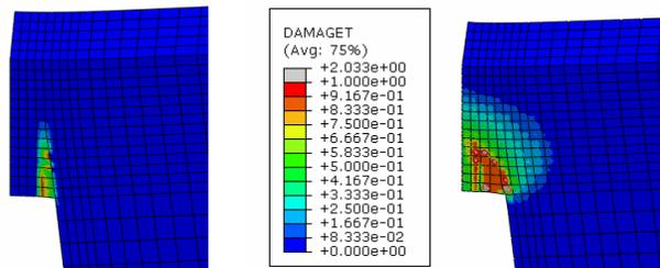
**Figure 4-17: The influence of  $\mu$  on the damage distribution in a notched beam in 3-point bending.**
