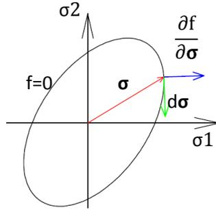
Figure 4-9: The principle plastic flow in 2D. The stress state must maintain on the yield surface. The green vector is the stress increment and the blue vector is normal to the stress increment.
