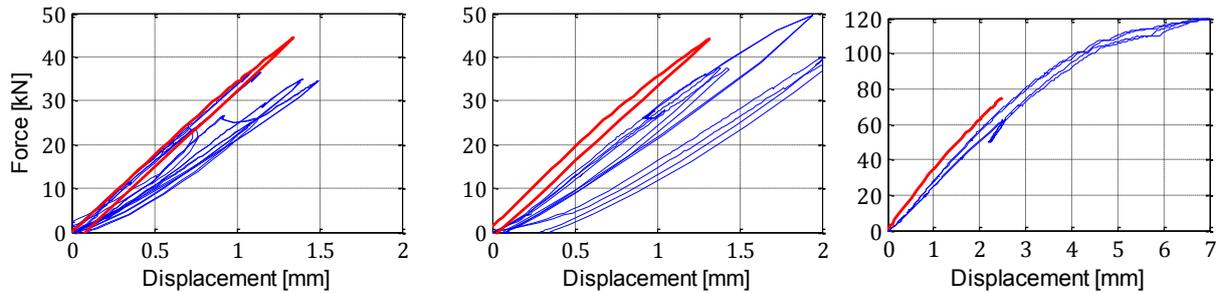
Figure 6-2: The numeric (red) and the experimental (blue) results for PCFT with HSC grout and friction in LS 1-3 counted from left. The blue curves are the force-displacement of CFT 1-3.
