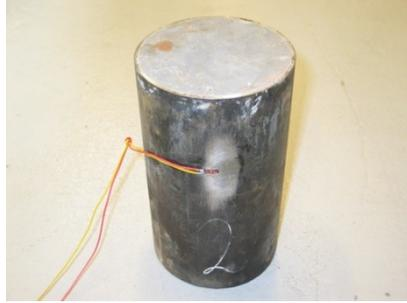
Figure 2-7: Test specimen 2. Length of steel tube is 250 mm; length of grout is 200 mm. The steel tube is greased before trial in order to remove contact between steel and grout.
