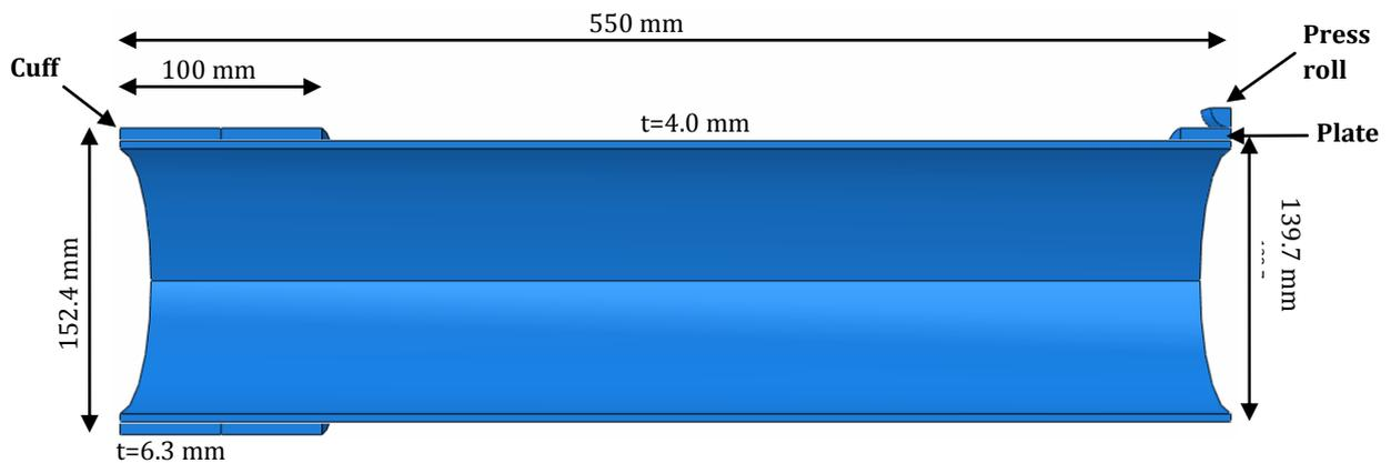
Figure 5-2: The geometry of the numeric model of the empty steel tube and the naming of setup parts.
