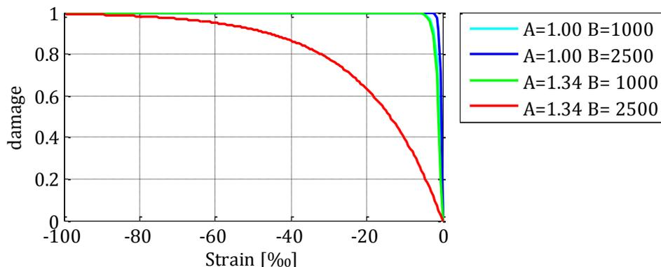
**Figure 4-20:** The influence of A and B on the damage development.
