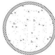
Figure 1-2: The section of a circular concrete-filled steel tube.
