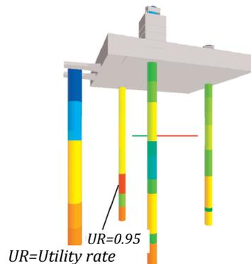
**Figure 1-27: Model of a platform. The colours indicate the utility rate of the elements, red is high and blue is low [1.12].**
