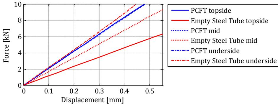
**Figure 3-10: The difference in the transversal displacement of the PCFT and the empty steel tube (numeric test). The stiffness of the empty steel tube seem higher when the displacement is measured at the underside of the beam as in the experimental tests.**
