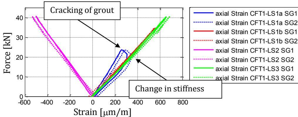
**Figure 3-13:** Force as function of axial strain in all load steps measured at strain gauge (SG) 1 and 2 for CFT 1. CFT1 was the initial test specimen and in LS 3 only loaded to 40 kN in order to inspect the grout core for cracks.
