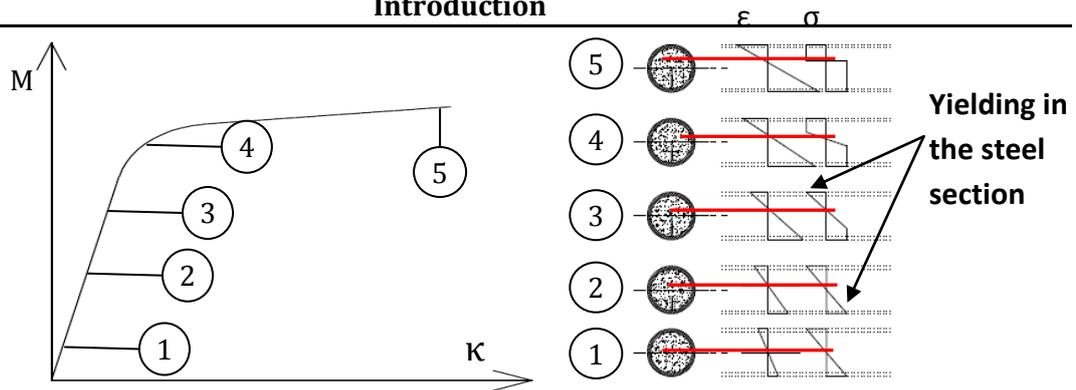
Figure 1-17: The principle progress of the bending moment,  $M$ , as a function of the curvature,  $\kappa$ , for the load situation in figure 1-16. To the right the strain- stress distribution in the section is shown at the numbered spots. The neutral axis is marked with the red lines [1.17].
