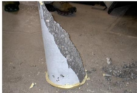
**Figure 4-4:** The shear failure in a concrete cylinder in uniaxial compression. [4.2]
