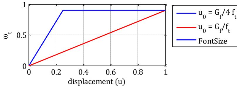
**Figure 4-21: The development of the tensile damage variable.**
