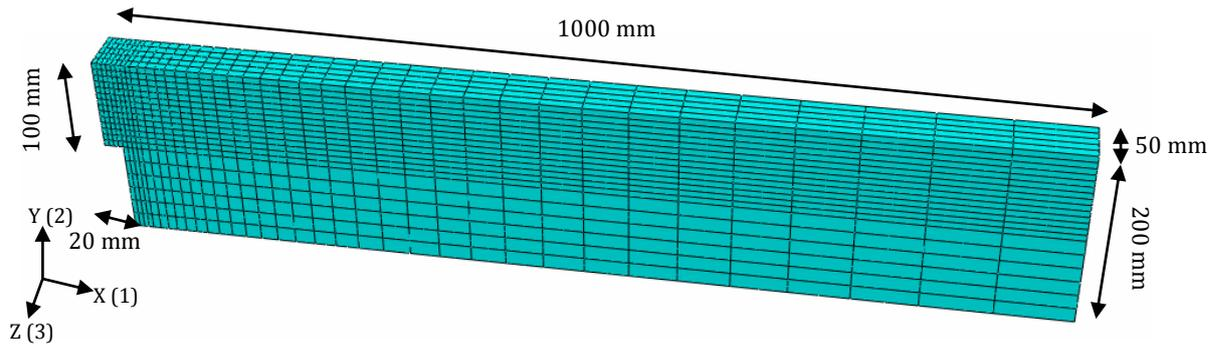
**Figure 4-23: The geometry of the concrete beam. Symmetry consideration has been made. The depth=50 mm.**
