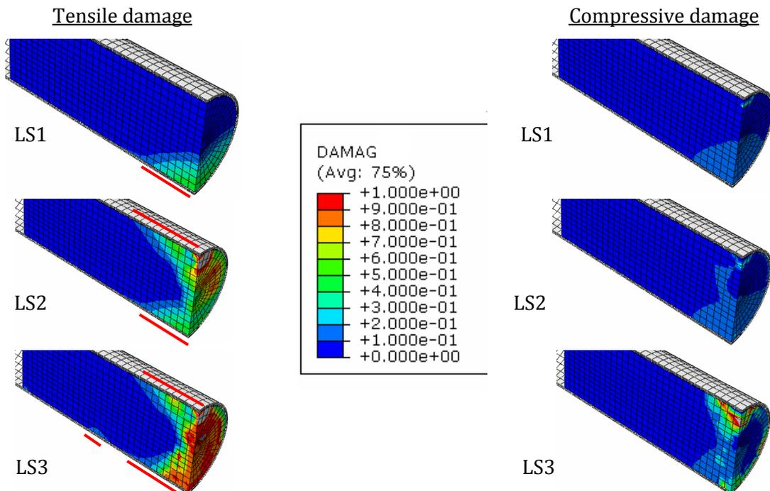
Figure 5-23: The tensile (left) and compressive (right) damage in the grout of the PCFT with HSC grout and no friction at the end of load step 1 (top) to 3 (bottom). The red lines indicate the area the damage is smeared to.
