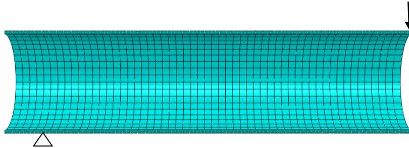
Figure 5-15: The mesh and boundary conditions. Planes of symmetry according to
