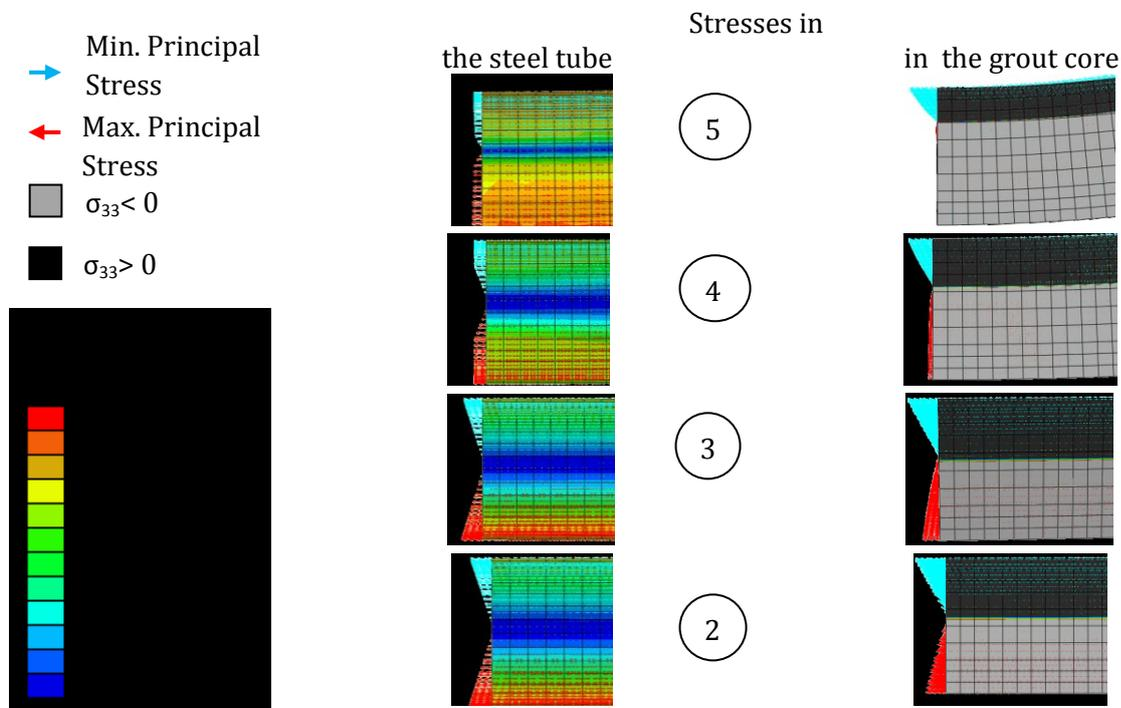
Figure 1-18: The Von Mises stresses in the steel tube (middle) and the axial stress,  $\sigma_{33}$ , in the grout core (right). The vectors= max and min principal stress. Legends are to the left. Numbers refers to figure 1-17.
