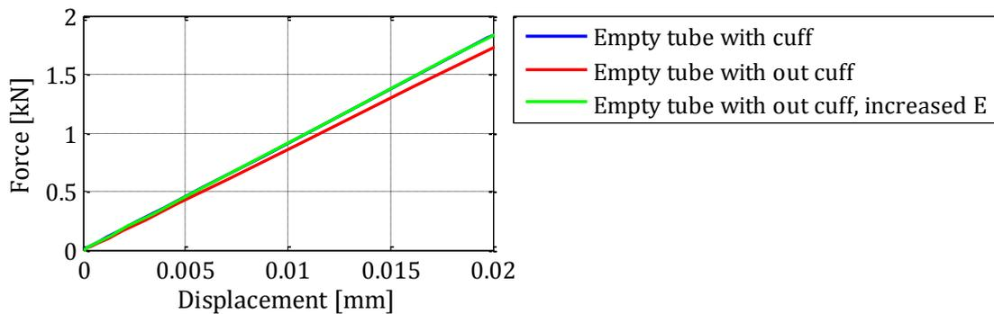
**Figure 5-14: The force as function of the difference in the displacement at mid-height of the steel tube.**
