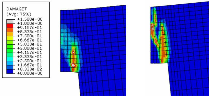
**Figure 4-30: The damage distribution for the linear softening (left) and the bilinear softening (right).  $\mu=1E-3$ .**
