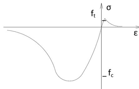
Figure 4-1: Principal stress – strain relation in concrete
