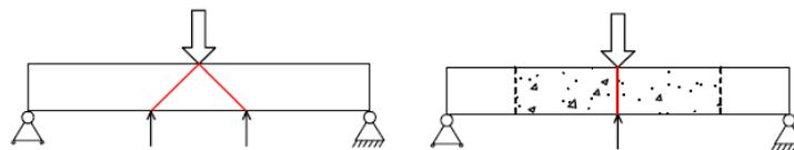
**Figure 3-8: Principal distribution of the transversal force in the empty steel tube (left) and the PCFT (right).**
