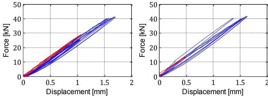
Figure 6-4: LS 1-2 for PCFT with LSC grout friction. The blue curves are the force-displacement of CFT 7-9.
