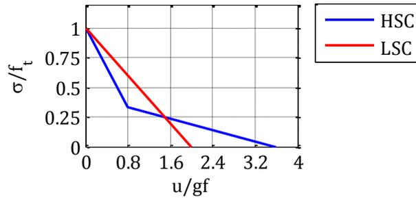
**Figure 4-19:** The softening expressed in a linear and a bi-linear stress-displacement relation – normalized with  $f_t$  and  $G$  respectively.
