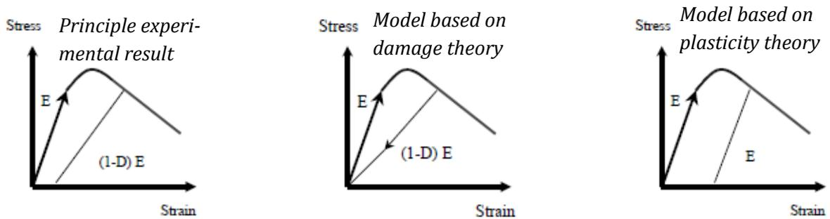
Figure 4-6: Basic differences of the damage theory and the plasticity theory. Experimental test results are found as a combination of the two models. [4.4]
