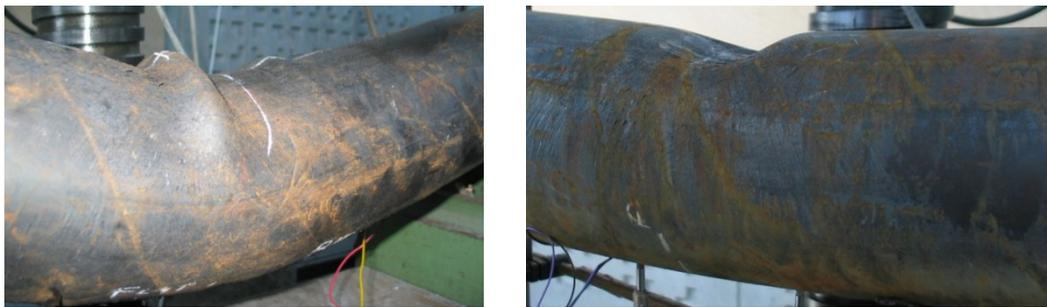
**Figure 6-15:** The outward buckling in steel tube with HSC grout (left) and the inward buckling in the steel tube with LSC grout. The inward buckling is located where the load is applied.
