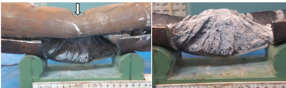
Figure 1-26: The shear failure of a CFT  $\text{Ø}88/4$  with high strength concrete (masterflow® 9500;  $f_c=115$  MPa). The test is made by the author in autumn/2010. The steel tube was cut open (left) and the inclined cracks of the shear failure in the grout was made visible (right).
