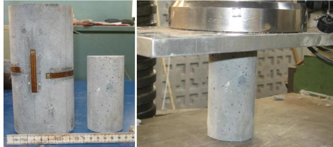
**Figure 2-1: The sizes of the cylinders for testing the compressive strength (right) and the test setup (left)**
