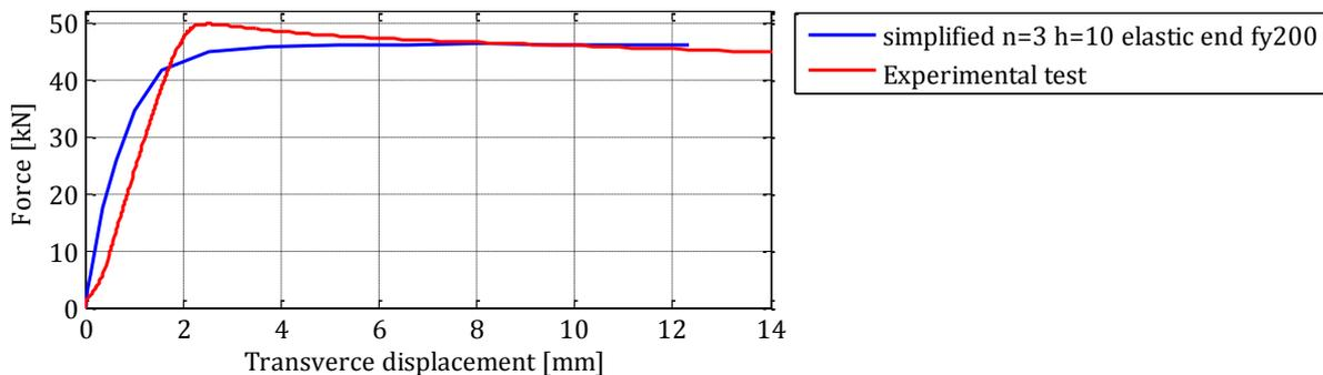
Figure 7-3: The fitting of the simplified model to the experimental result of the empty steel tube.
