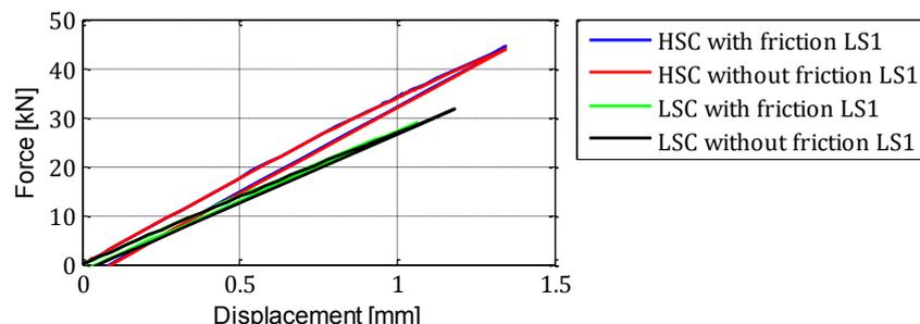
**Figure 7-4: The flexural stiffness is visualized as the slope of the load deflection curves. The PCFTs with HSC grout have an increased flexural stiffness compared to the LSC grouted PCFTs.**
