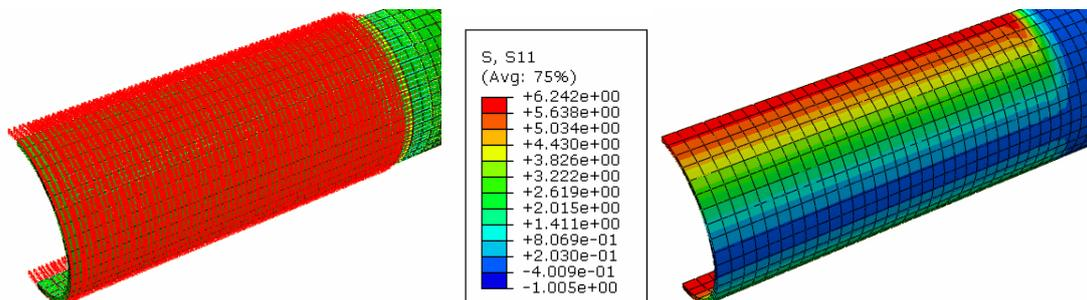
Figure 7-1: The hoop stresses in the numeric model caused by heating the grout.
