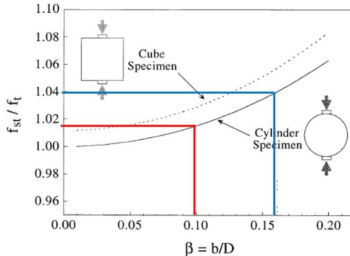
**Figure 2-4: Variation of the splitting tensile strength with the relative width of the load bearing strips,  $b$ . [Rocco] The red line is  $\beta$  for the  $\varnothing 100$  cylinders (LSC), the blue line for  $\varnothing 60$  cylinders (HSC).**
