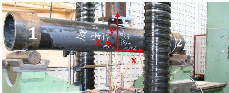
Figure 3-3: Test setup for the empty tube. The local Cartesian coordinate system is defined with origo according to the figure. "1" and "2" identifies the tube halves, which describes the measuring points.
