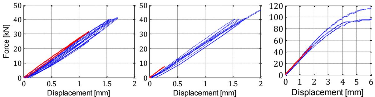
Figure 6-5: LS1-2 for PCFT with LSC grout without friction. The analysis in the lower plot was conducted without changing the load direction. The blue curves are the force-displacement of CFT 10-12.
