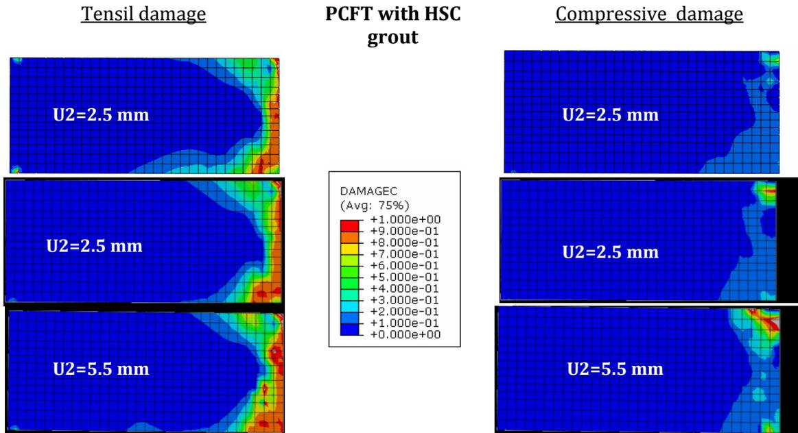
Figure 6-8: Comparison of the damage pattern in the grout for PCFT with HSC grout and with friction (top) and without friction (mid and bottom). The displacement in the PCFT is 2.5 mm in the plot in the top and middle and 5.5 mm in the plots at the bottom.
