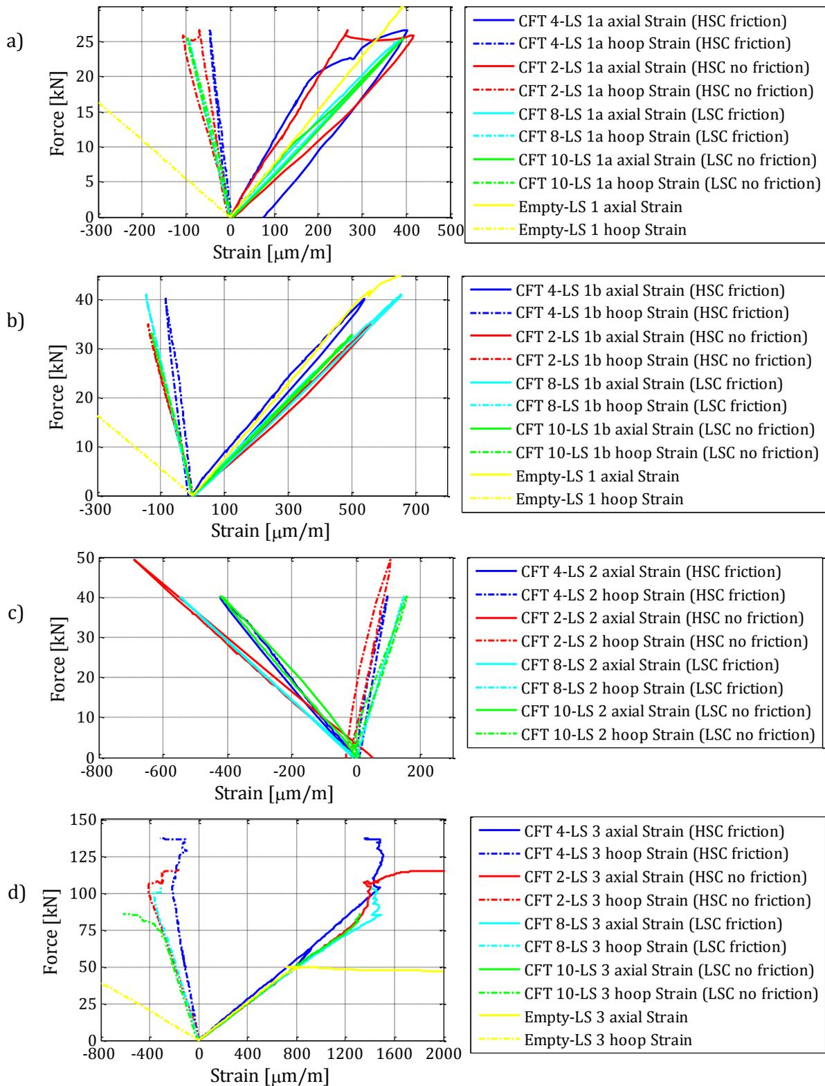
Figure 3-12: The force-strain relation for CFT 2, 4, 8 and 10 in load step 1a, 1b, 2 and 3 counted from the top.
