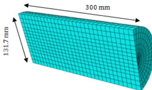
Figure 5-16: The geometry and the mesh of the grout core.
