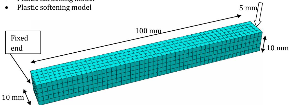
Figure 4-12: A cantilever beam 100x10x10 mm exposed to a transverse loading is tested. Three material models are used: a plastic model, a plastic hardening and a plastic softening model.
