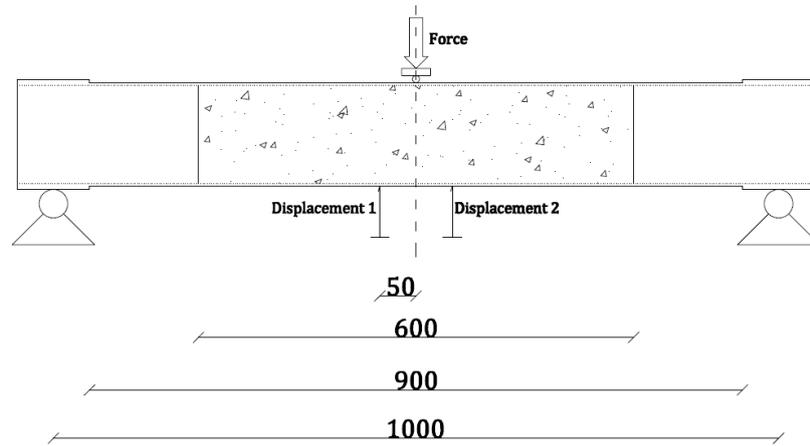
Figure 3-2: The geometry of the test specimens. Displacements are measured 50 mm on each side of the axial line of symmetry.
