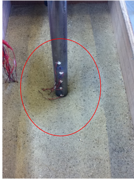
Figure 5.16: Picture of the crater in sand around the pile after cyclic loading in dry sand. The boundaries of the crater are marked with a red line.
