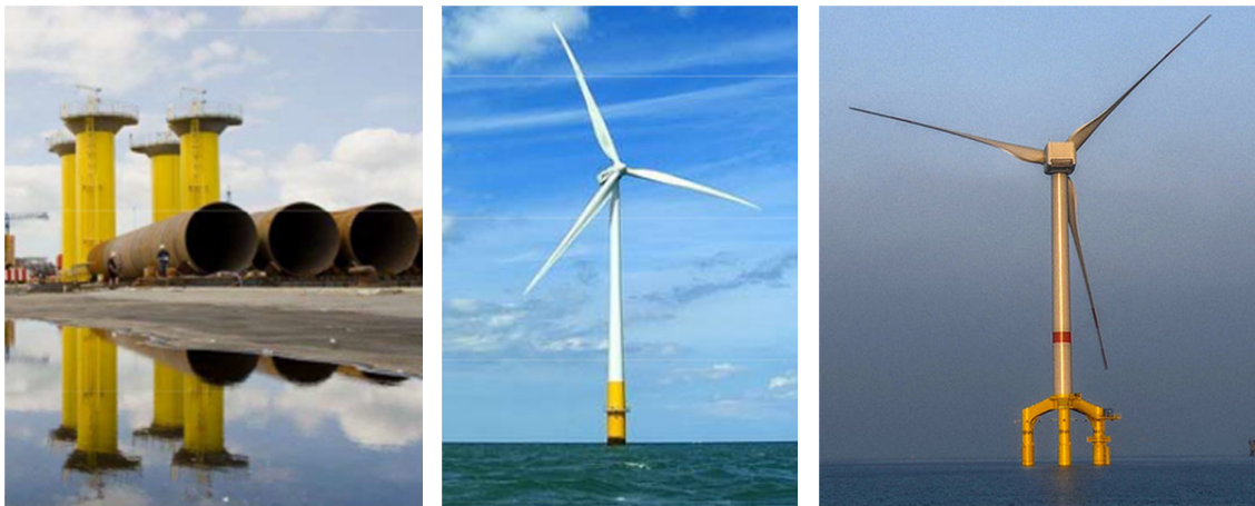
Figure 1.1: To the left: Monopile foundations and transition piece ready for shipping. The piles have diameters of about 4 m [W.4]. In the middle: 2.3 MW wind turbine from Horns Rev, founded on a monopile foundation [W.4]. To the right: 5 MW turbine from Hooksiel offshore windfarm in Germany. The turbine is founded on a tripod foundation with three monopiles [W.5].
