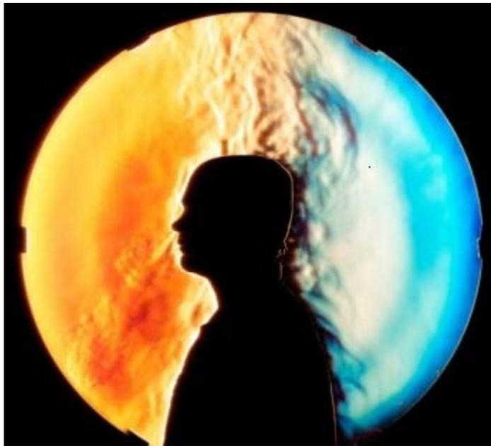
Figure 2.1: Schlieren photograph illustrates the thermal plume around a person.
