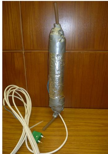
Figure 2.13: Heating unit used to heat up exhalation air.
