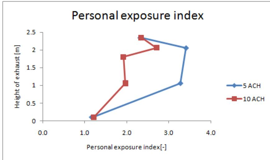
Figure 7.6: Personal exposure index dependent on the height of the exhaust and the ACH.
