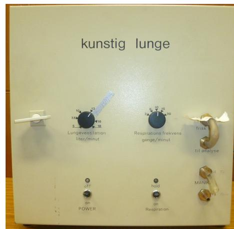
Figure 2.12: Respiration helped along with a compressor inside the shell.
