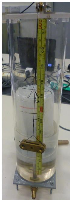
Figure 10.17: Equipment for calibrating the minute volume of the artificial lung.
