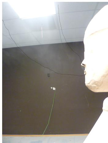
Figure 10.9: Upward flow around the maninikin.
