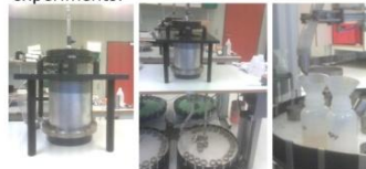
The leaching set up. The columns were irrigated with artificial rain water applied uniformly from the irrigation head.
