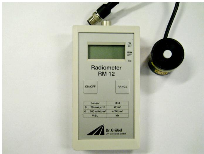
The radiometer should ideally measure the same intensity as showed in the Multiteser display "set dose". An interactive excel sheet can be used for calculation of the radiometer output measured in watt (W).
