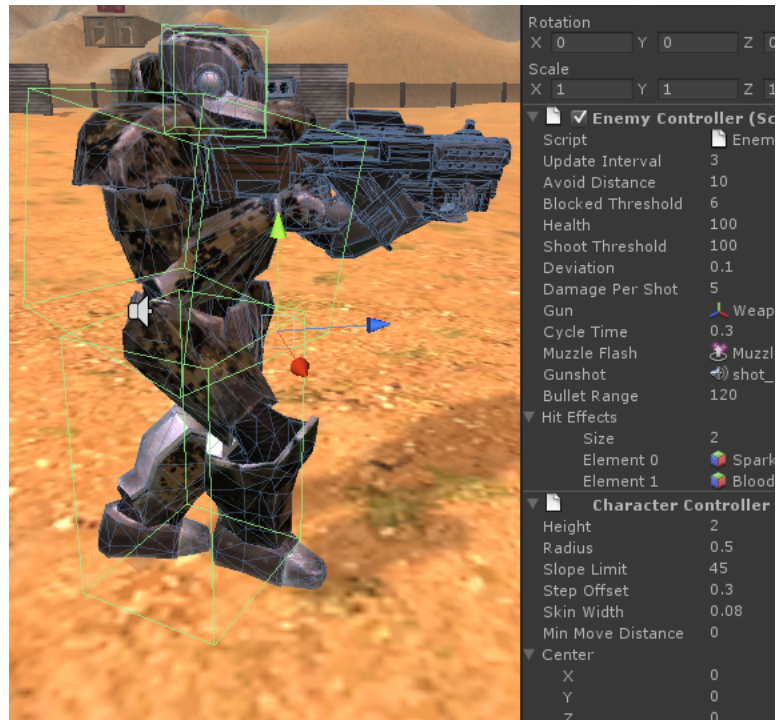
Figure 12: Shows the build up of a bot inside of the Unity editor.
