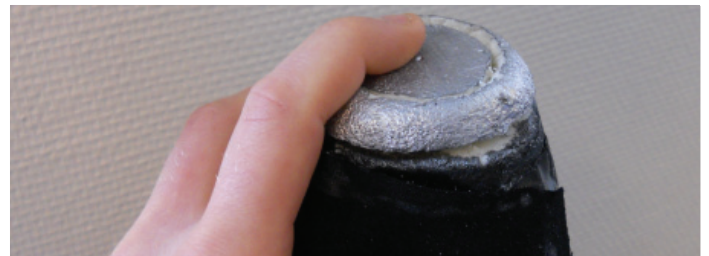
Figure 57: Merging of volume adjustment (wheel), power on/off (button), and source selection (buttons) into one end of the product
