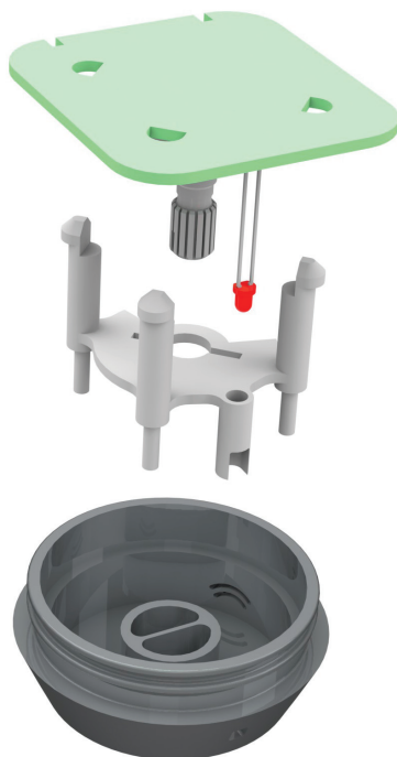
Figure 85: Exploded view of the source wheel with reuse of the PCB board bracket.
