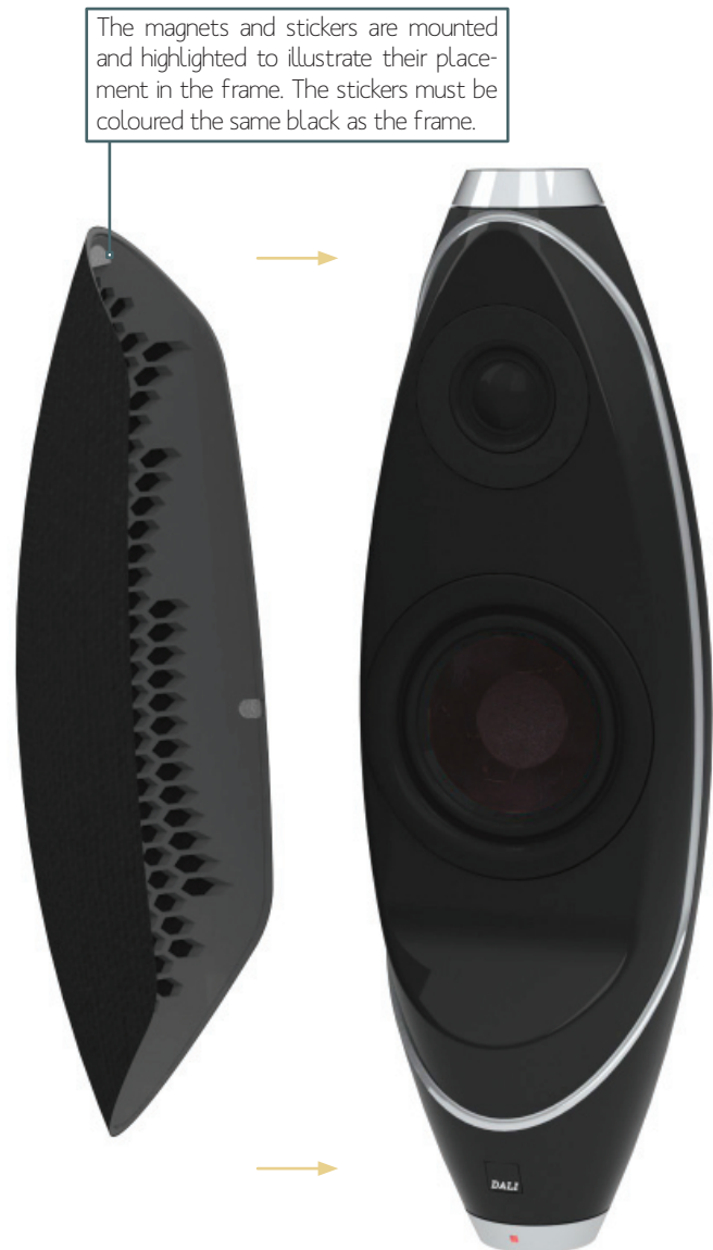
Figure 72: The cloth frame is attached to the loudspeaker by 3 magnets in the frame, and additionally 3 magnets inside the loudspeaker's front body part.
