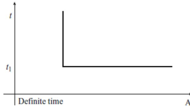
**Fig. 3.2 Definite time/current or definite time characteristic of over-current relays**
