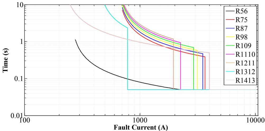
**Fig. 4.14 Time over-current characteristics plot of relays R56, R75, R87, R98, R109, R1110, R1211, R1312 and R1413 for the case where the WTGs have been replaced by GTGs**
