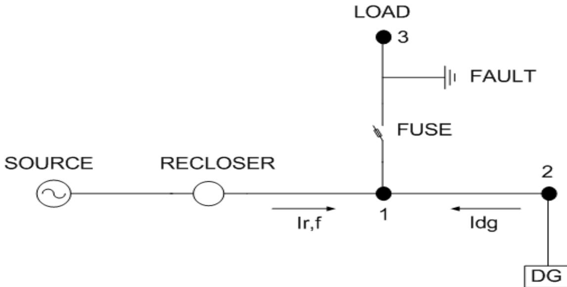
**Fig. 2.14 Network example with embedded generation**
