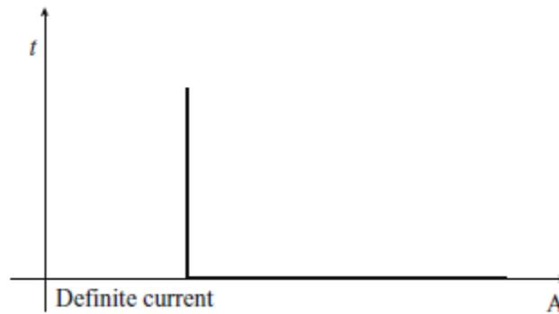
**Fig. 3.1 Definite current characteristic of over-current relays [7]**
