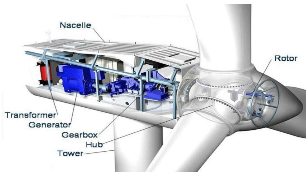
**Fig. 2.2 Schematic operation diagram of a wind turbine [12]**
