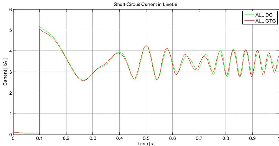
**Fig. 4.31 Short circuit current comparison in Line56 for the condition in which all the DG are connected and with all the GTG**
