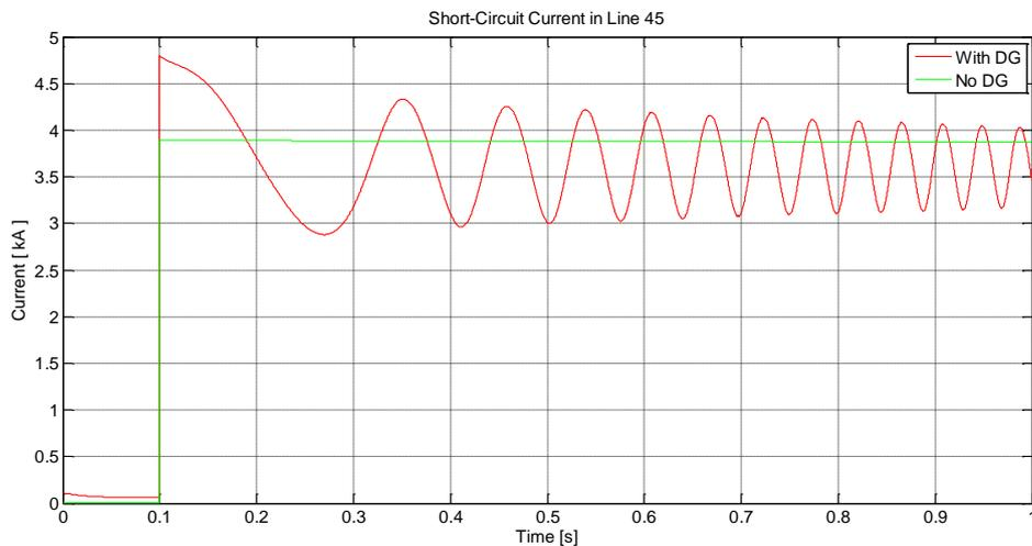
**Fig. 4.19 Short circuit current comparison in Line45 for Case1 and 2**
