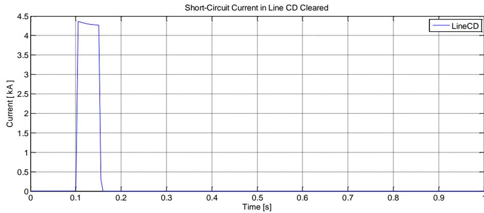
**Fig. 3.16** Clearing fault when DG2 and DG3 are connected to the system
