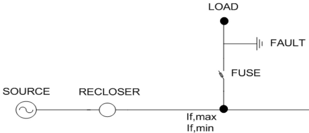
**Fig. 2.12 Part of a distribution network including relay and fuse**
