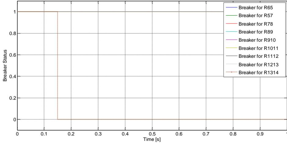
**Fig. 4.9 Status of circuit breaker for a three phase fault in Line1314 for Case2 when relays are setting according to Fig. 4.8**
