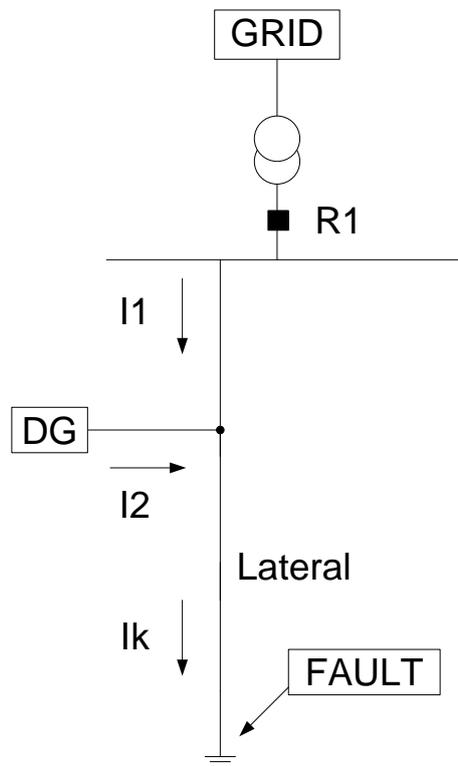
**Fig. 2.11 Reduction of reach of protective devices**
