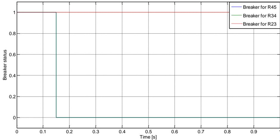
**Fig. 4.18 Status of circuit breaker for a three phase fault in Line45 for Case2 when GTG1 and GTG3 are connected and relays are set according to Fig. 4.16**
