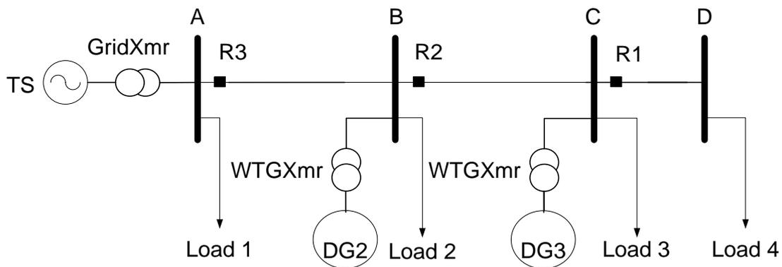
**Fig. 3.13 Multiple DGs connected to radial systems**
