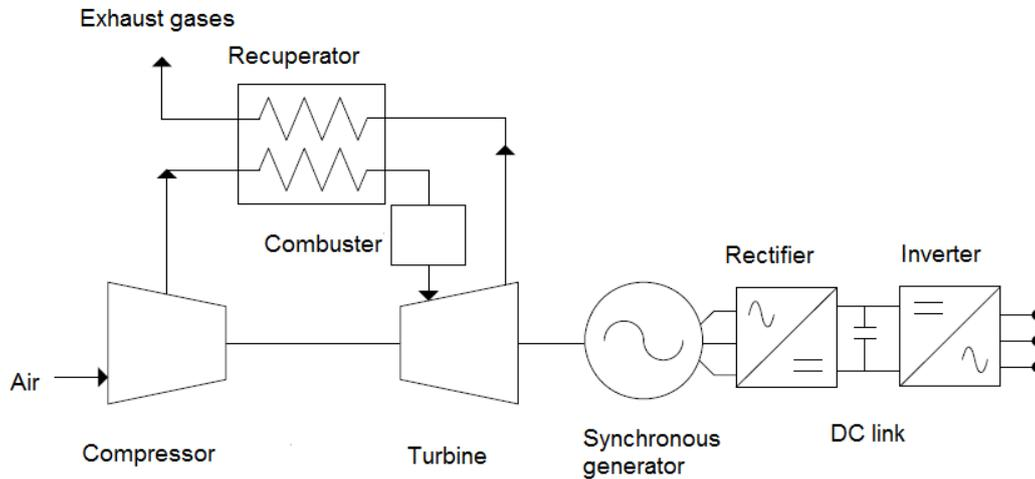
**Fig 2.4 Schematic diagram of a micro-turbine [10]**
