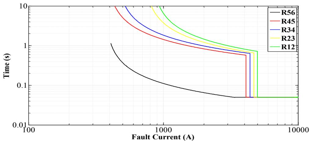
**Fig. 4.23 Time over-current characteristics plot of relays R56, R45, R34, R23 and R12 for Case2 when GTG2 and GTG3 are connected**
