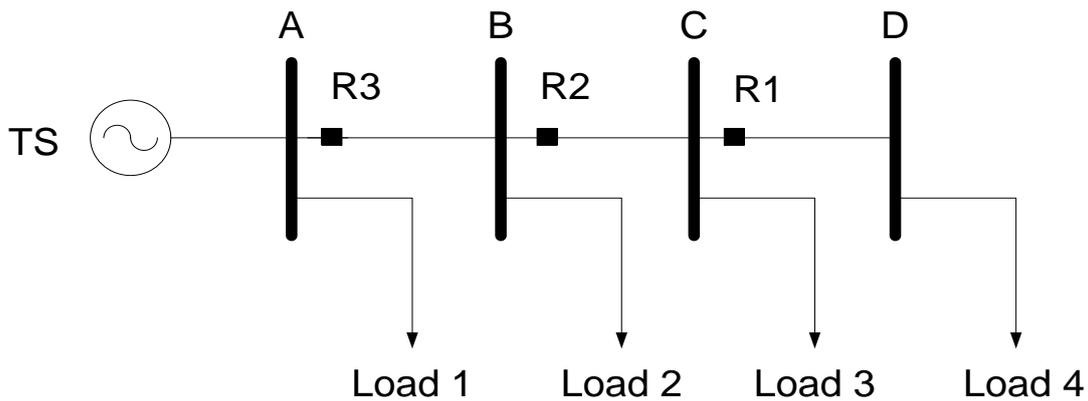
**Fig. 3.6 Distribution system without distributed generation**
