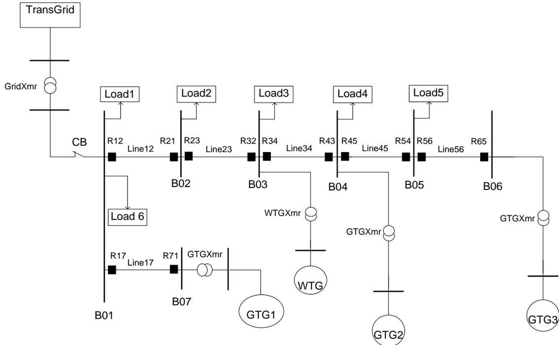
**Fig. 4.15 Modified test distribution system**
