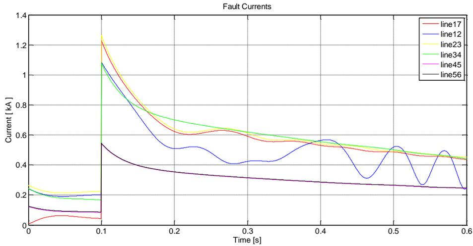
**Fig. 4.32 Fault currents for Case2 when GTG1, GTG2, GTG3 and WTG are connected**
