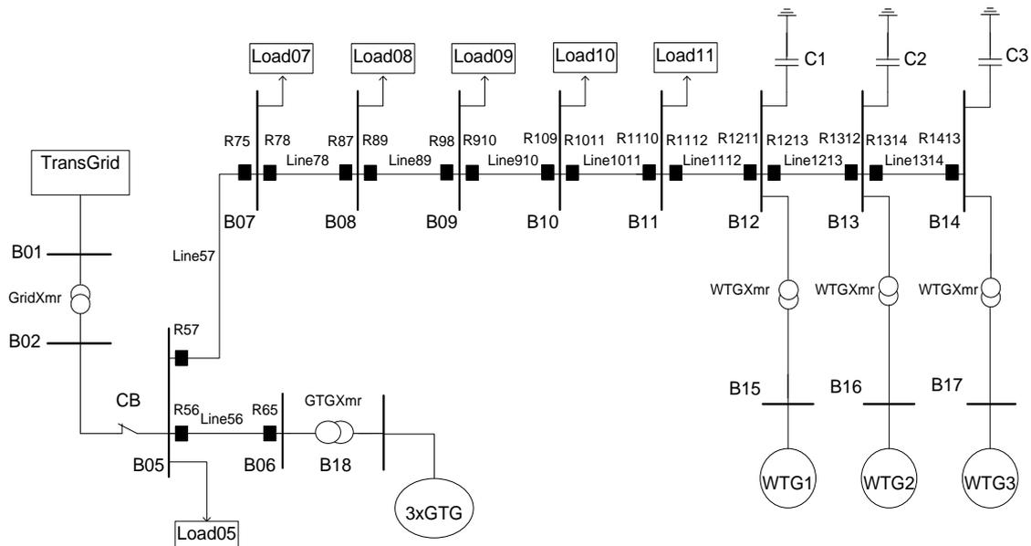
Fig. 4.2 Model of the test distribution network
