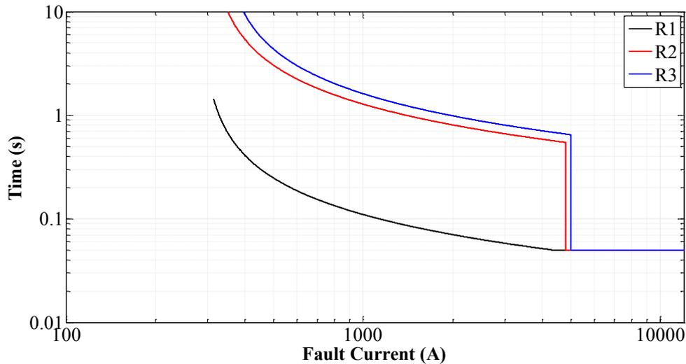
**Fig. 3.9 Time over-current plot of relays R1, R2 and R3.**
