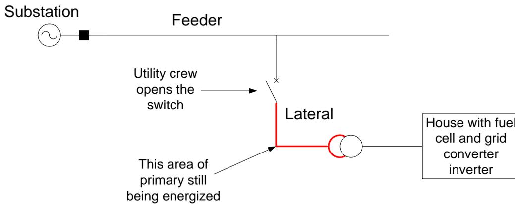
**Fig. 2.9 Islanding of a DG system**
