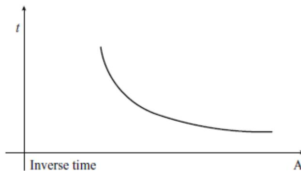
**Fig. 3.3 Inverse time/ current characteristic of over-current relays [7]**
