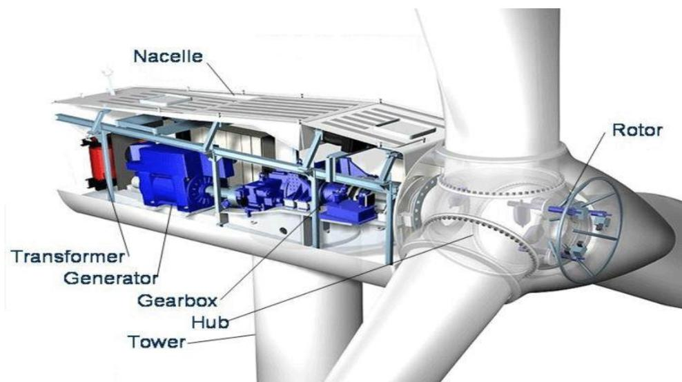
**Fig. 2.2 Schematic operation diagram of a wind turbine [12]**
