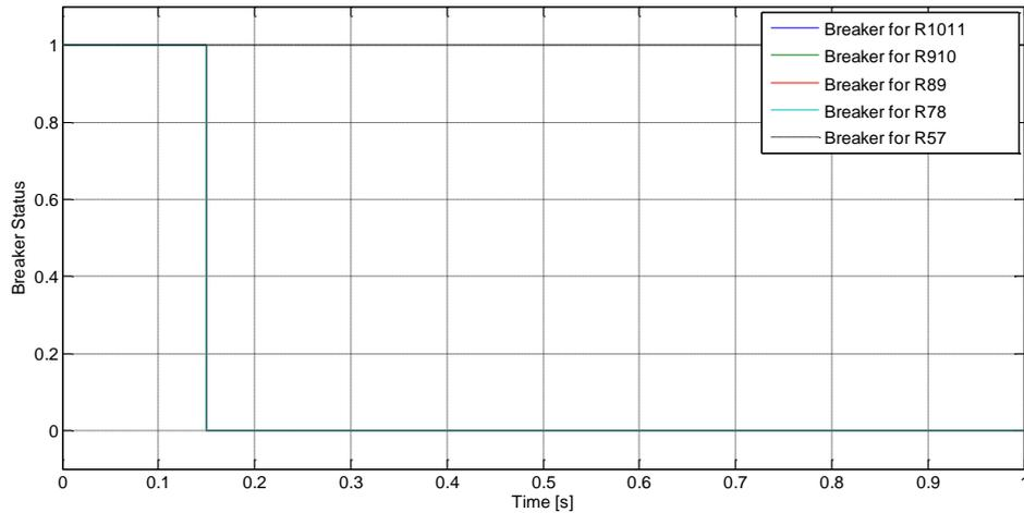
**Fig. 4.6 Status of circuit breaker for a three phase fault in Line1011 for Case2 when relays are setting according to Fig. 4.4**
