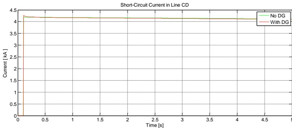
**Fig. 3.8 Short circuit current in line CD with and without DG1**
