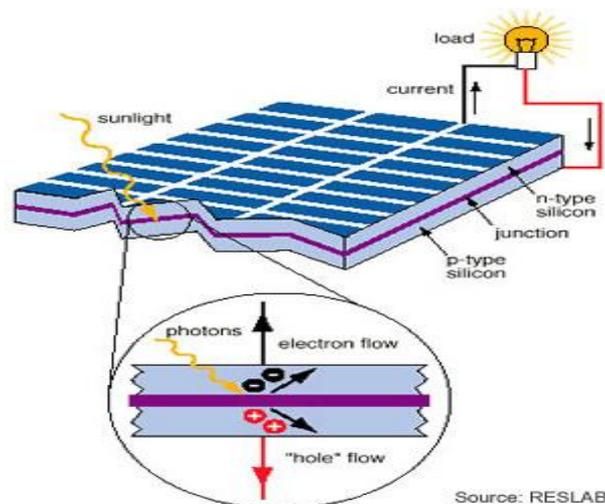
**Fig. 2.1 Schematic diagram of a photovoltaic system [11]**
