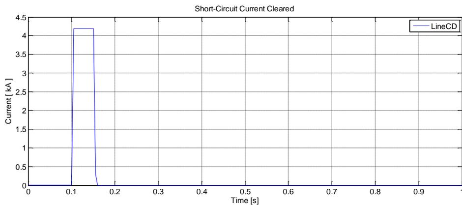
**Fig. 3.10 Fault cleared after the relay picks up time**
