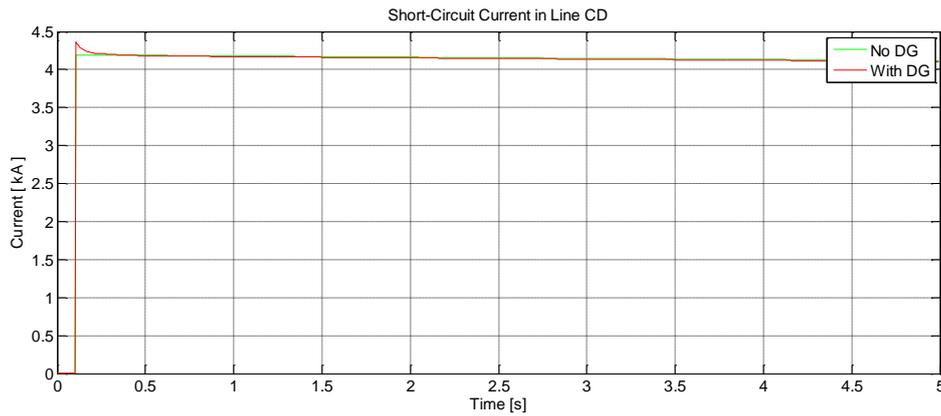
**Fig. 3.14 Short circuit current in line CD with DG2, DG3 connected and without DG**
