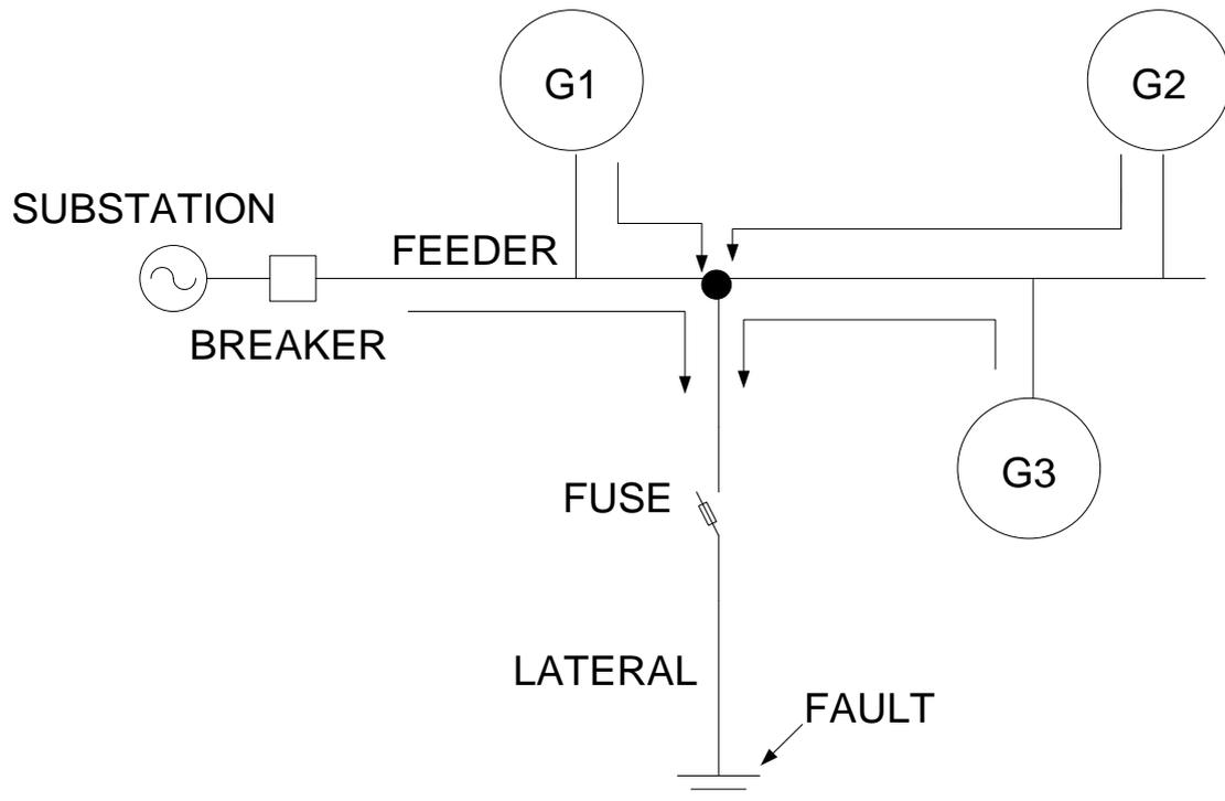
**Fig. 2.7 Fault contributions due to DG units 1, 2 and 3 are embedded in the system. Fuse-breaker coordination may be no longer achieved**
