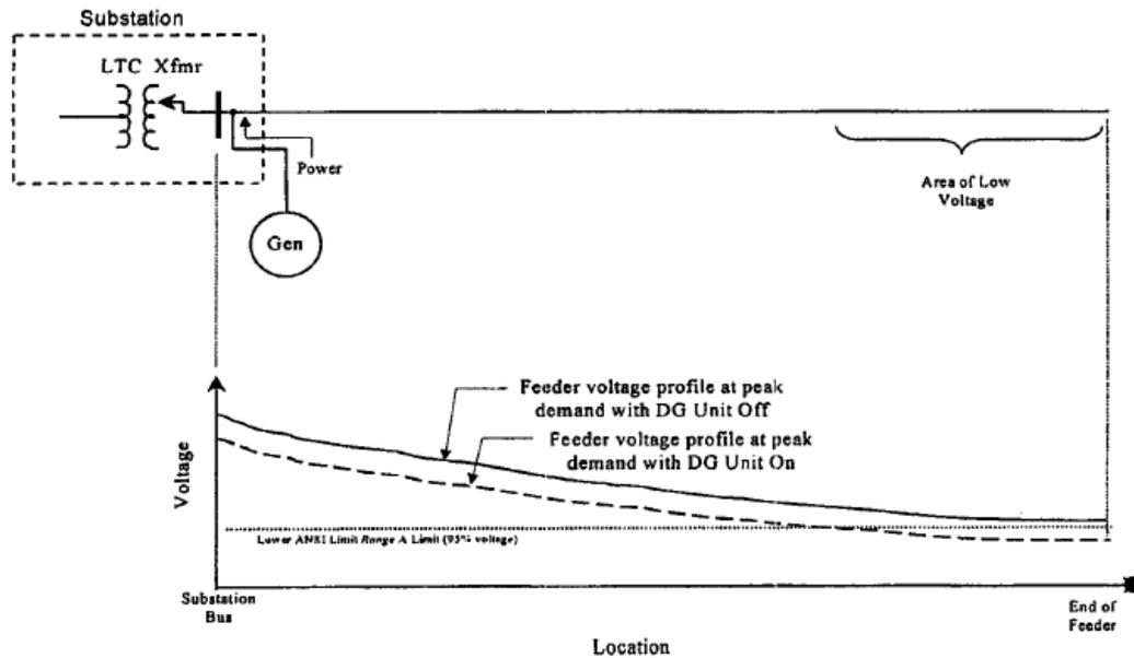
**Fig. 2.5 Voltage profiles with and without DG [3]**
