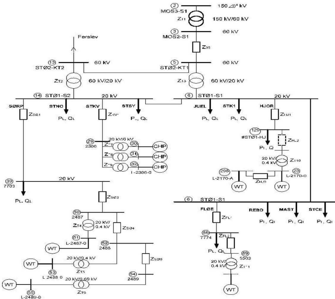
Fig. 4.1 Local distribution network at Støvring in Nordjylland [31]
