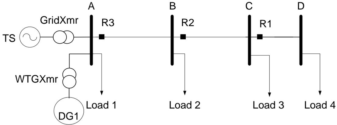
**Fig. 3.7 Single DG connected to bus A**
