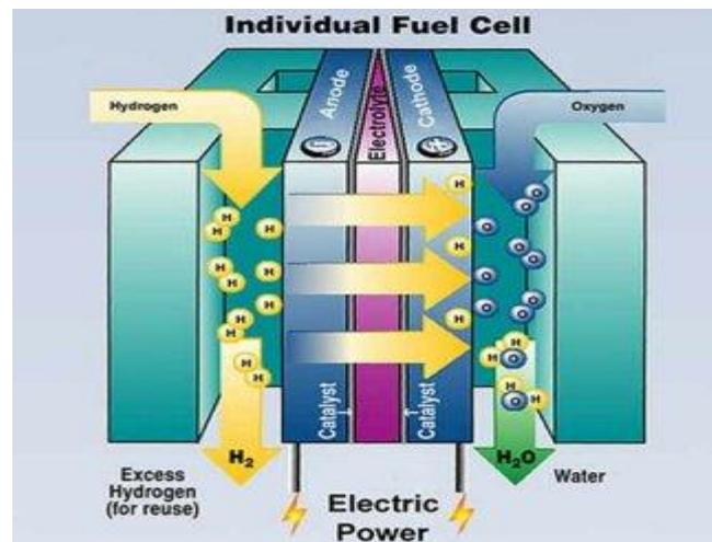
**Fig. 2.3 Schematic diagram of a fuel cell [13]**
