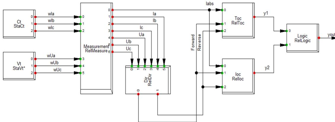
**Fig. 3.5 Block diagram of directional over-current relay**
