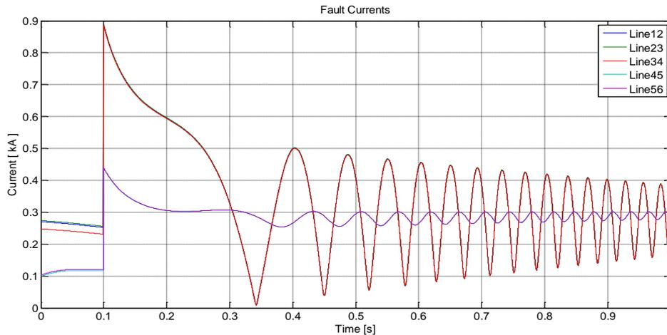
**Fig. 4.24 Fault currents seen by the relays R21, R32, R43, R54 and R65 for a fault in Line12 close to Bus 02 when GTG2 and GTG3 are connected**
