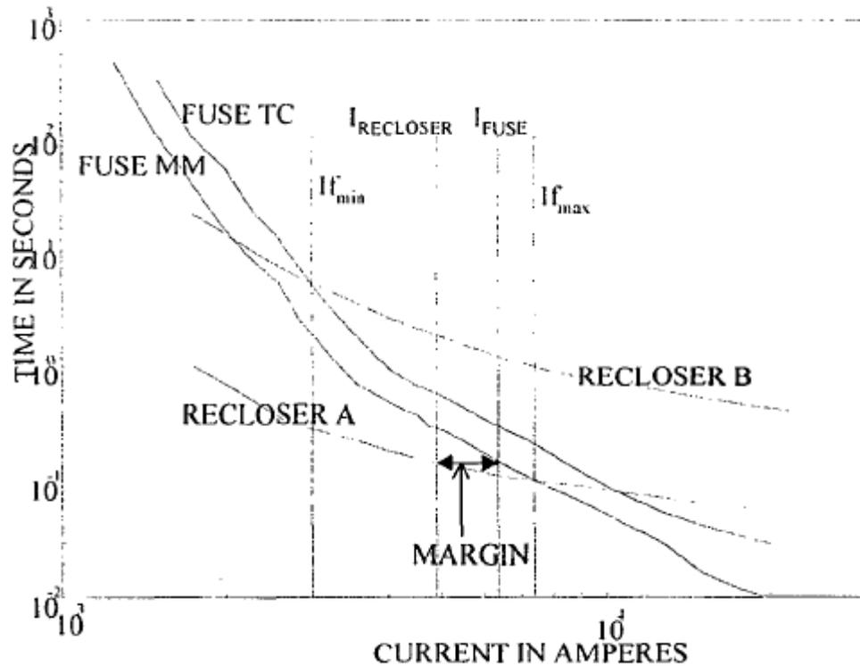
**Fig. 2.15 Coordination margin between fuse and recloser**
