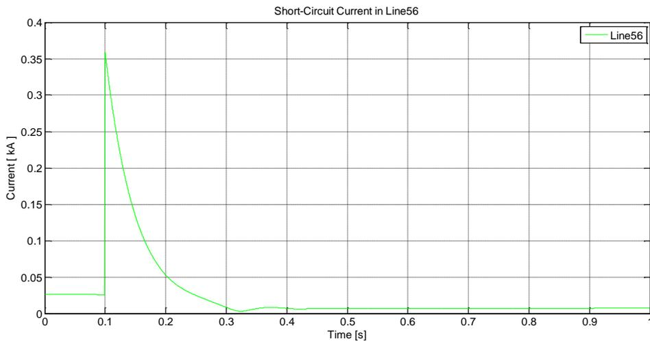
**Fig. 4.10 Short circuit current seen in Line56**
