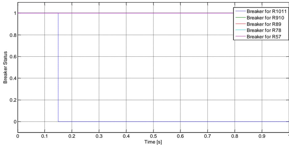
**Fig. 4.5 Status of circuit breaker for a three phase fault in Line1011 for Case1 when relays are setting according to Fig. 4.4**
