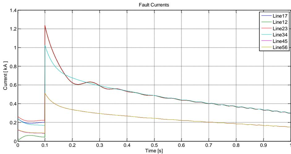
**Fig. 4.33 Fault currents seen by the relays R21, R32, R43, R54 and R65 for a fault in Line17 close to Bus 01 when GTG1, GTG2, GTG3 and WTG are connected**
