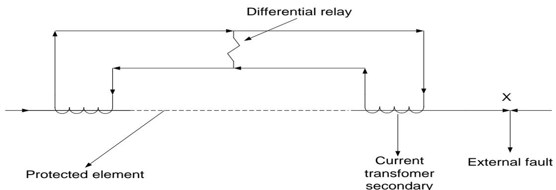
**Fig. 4.34 Differential relay behaviour for an external fault**
