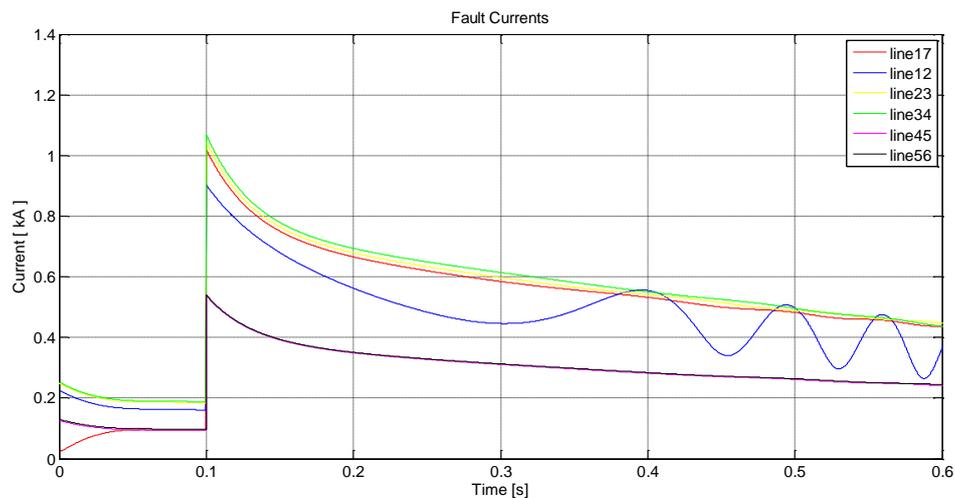
**Fig. 4.28 Instantaneous pickup currents for Case2 when GTG1, GTG2 and GTG3 are connected**
