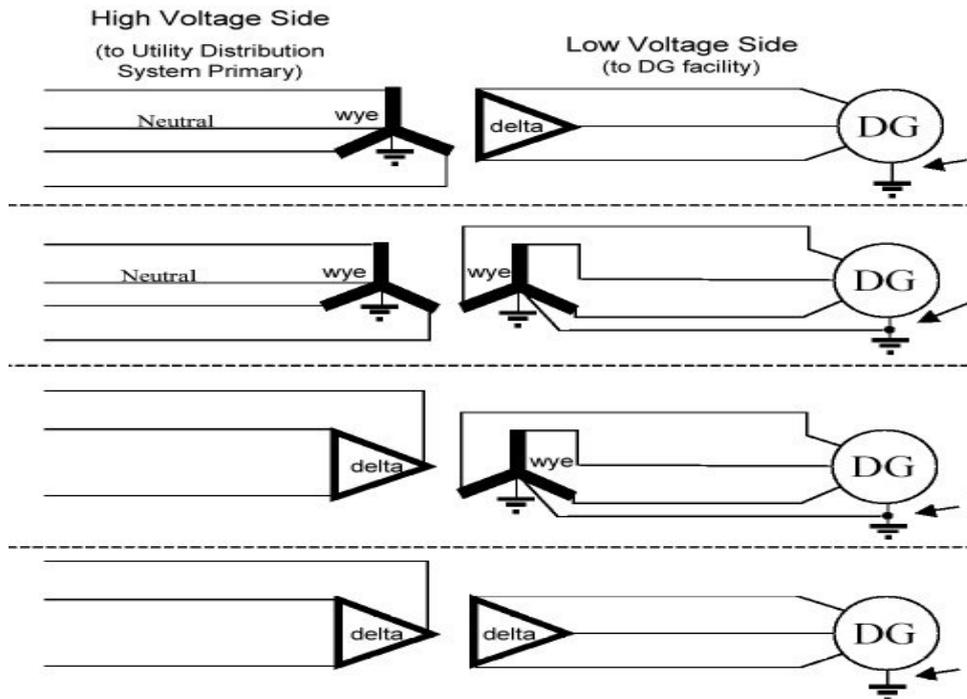
**Fig. 2.8 Commonly transformer connections used with DG [17]**
