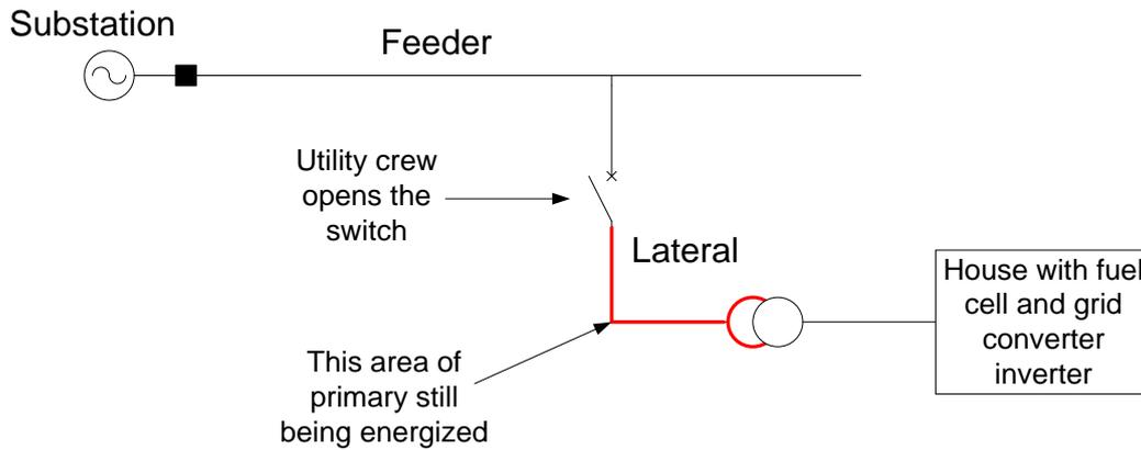
**Fig. 2.9 Islanding of a DG system**
