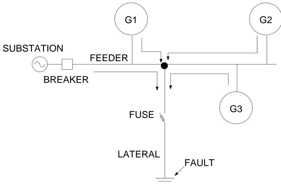
**Fig. 2.7 Fault contributions due to DG units 1, 2 and 3 are embedded in the system. Fuse-breaker coordination may be no longer achieved**
