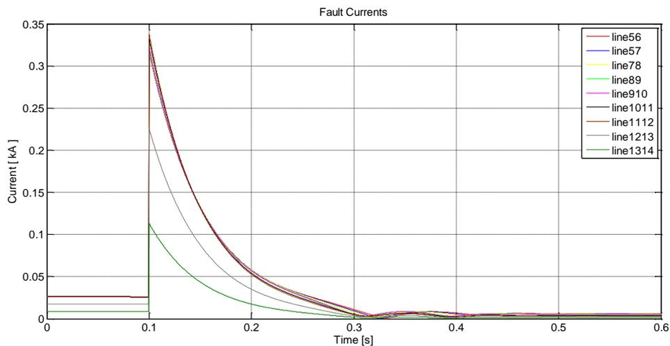
**Fig. 4.11** Fault currents seen by relays R56, R75, R87, R98, R109, R1110, R1211, R1312 and R1413 for three phase faults in each line of the test system
