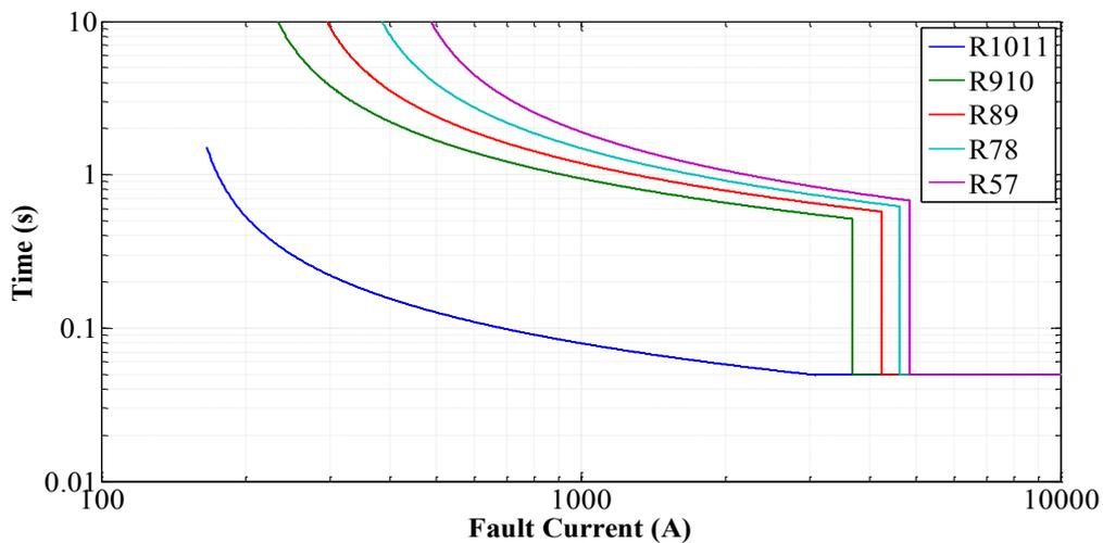
**Fig. 4.4 Time over-current characteristic plot of relays R1011, R910, R89, R78 and R57 for Case1**
