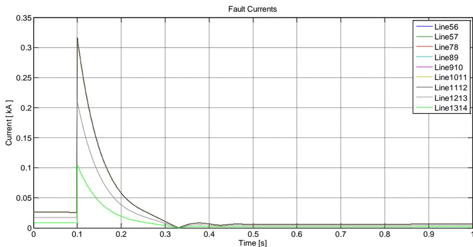
**Fig. 4.12** Fault currents seen by the relays R56, R75, R87, R98, R109, R1110, R1211, R1312 and R1413 for a fault in Line56 near to Bus 05
