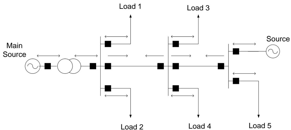
**Fig. 3.4 Application of directional over-current relays in multi-source networks**
