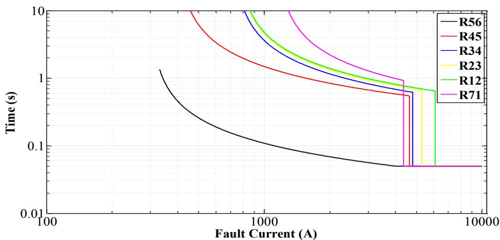
**Fig. 4.27 Time over-current characteristics plot of relays R56, R45, R34, R23, R12 and R71 for Case2 when GTG1, GTG2 and GTG3 are connected**
