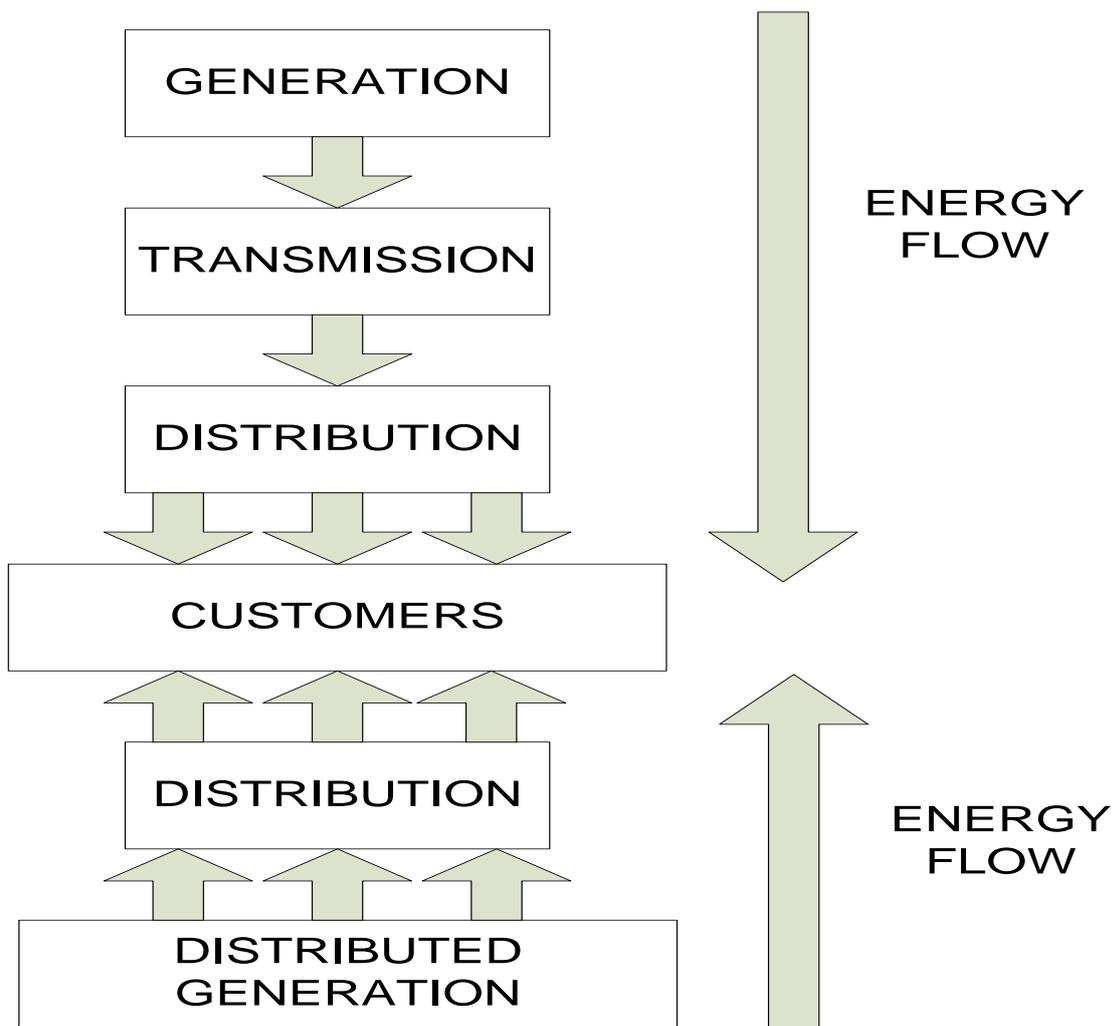
**Fig. 1.2 New industrial conception of the electrical energy supply**
