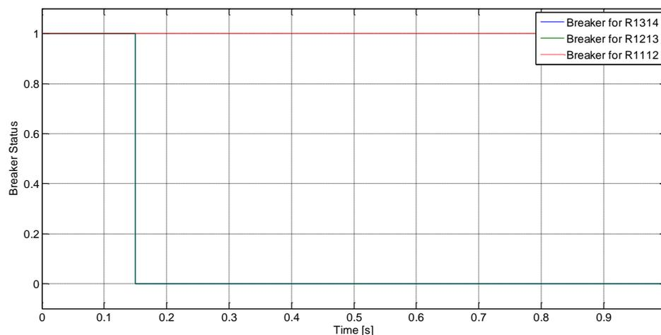
**Fig. 4.13 Status of circuit breaker for a three phase fault in Line1314 for Case2 where the WTGs have been replaced by GTGs and relays are set according to Fig.4.8**
