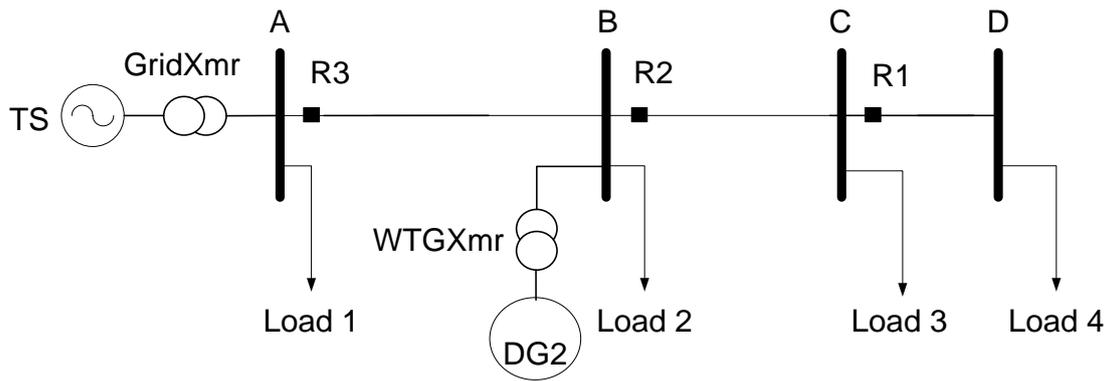
**Fig. 3.11** Single DG connected to bus B.
