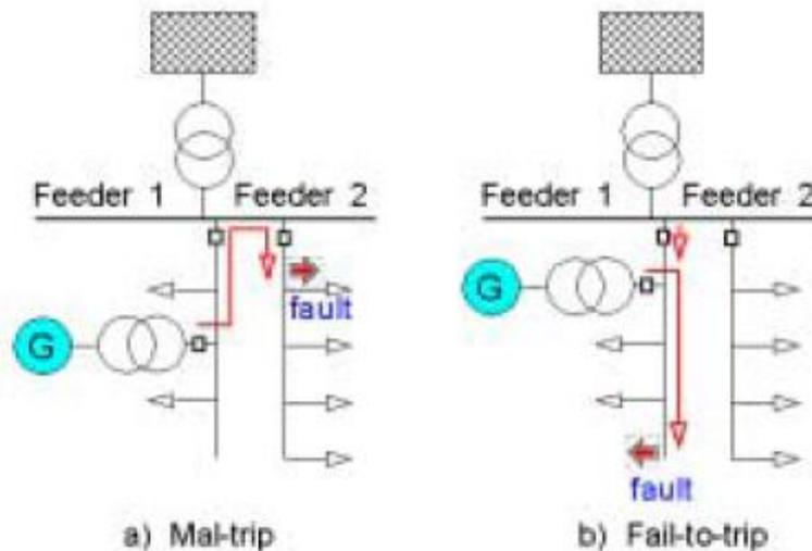
**Fig. 2.10 Mal trip and fail to trip [25]**
