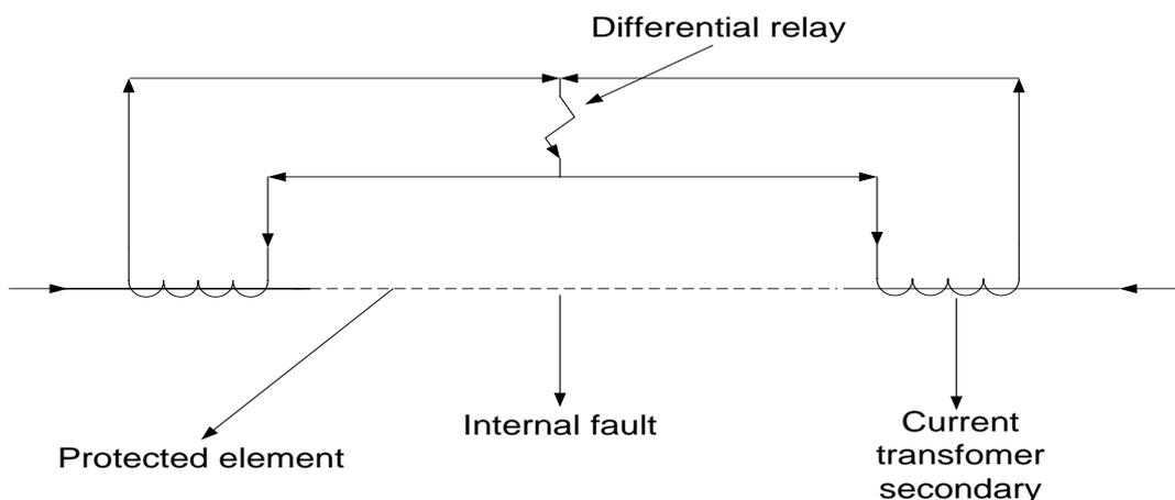
**Fig. 4.35 Differential protection relay behaviour for an internal fault**
