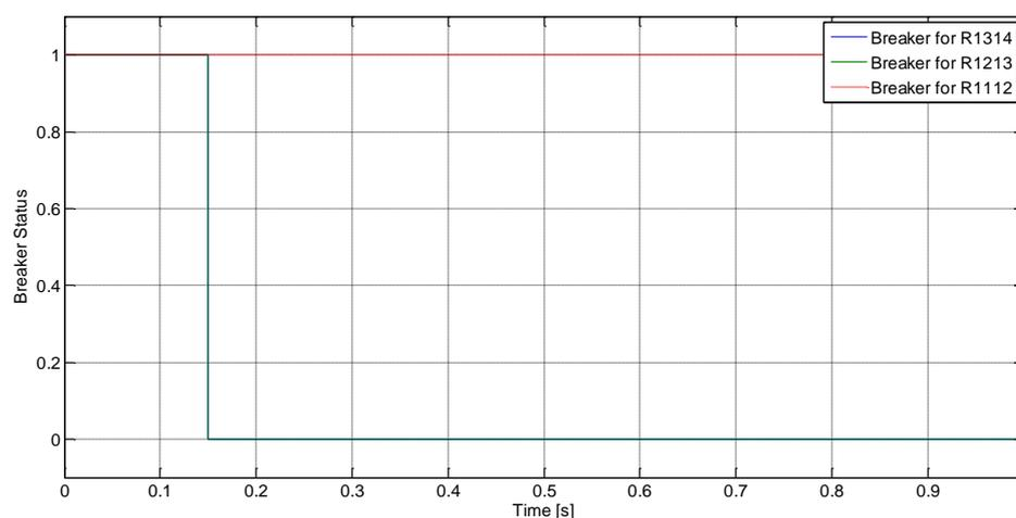
**Fig. 4.13 Status of circuit breaker for a three phase fault in Line1314 for Case2 where the WTGs have been replaced by GTGs and relays are set according to Fig.4.8**
