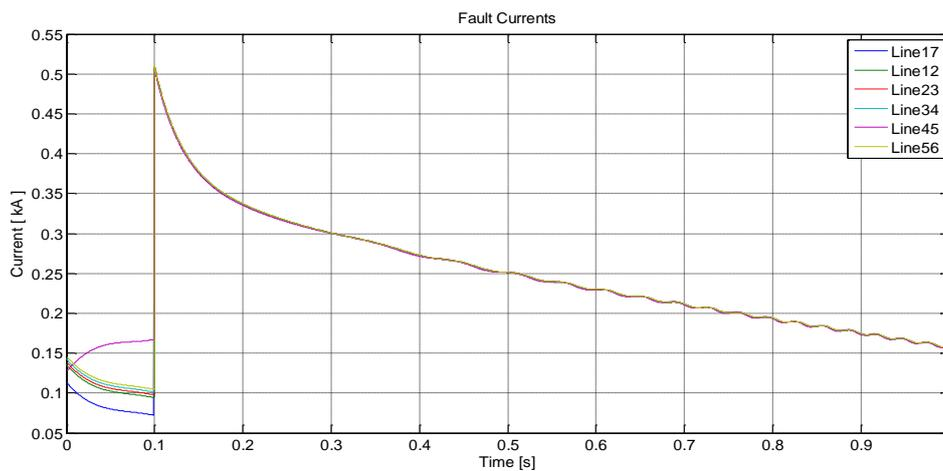
**Fig. 4.21 Fault currents seen by the relays R17, R21, R32, R43, R54 and R65 for a fault in Line17 close to Bus 01 when GTG1 and GTG3 are connected**
