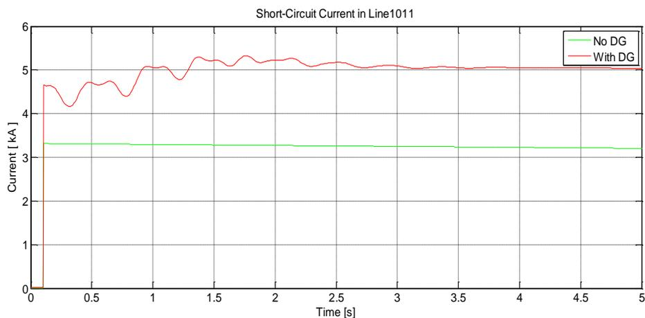
**Fig. 4.7 Short circuit current comparison in Line1011 for Case1 and Case2**
