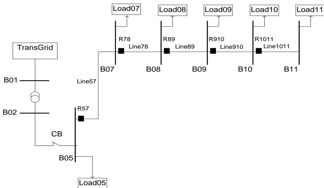
**Fig. 4.3 Modified radial distribution system for Case1**
