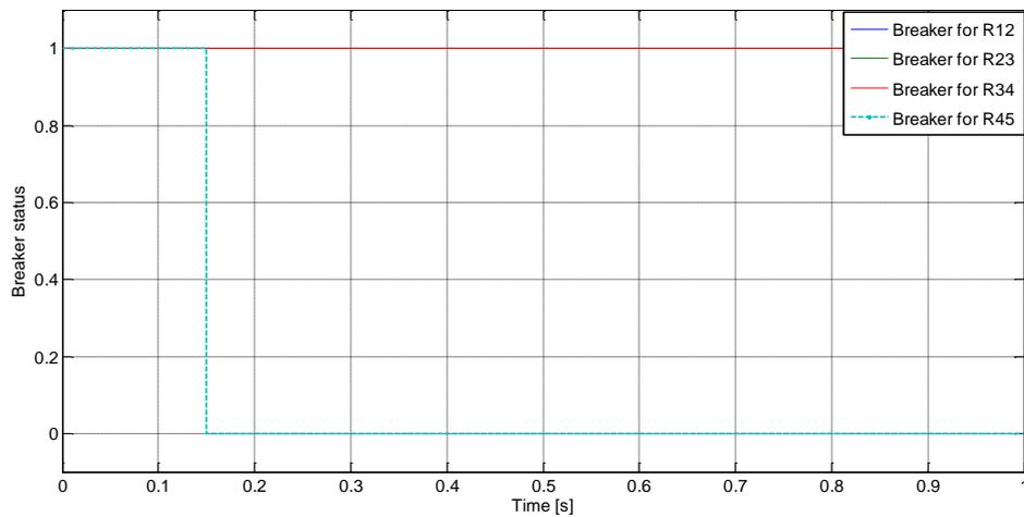
**Fig. 4.17 Status of circuit breaker for a three phase fault in Line45 for Case1 and relays are set according to Fig. 4.16**
