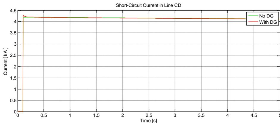
**Fig. 3.12** Short circuit current in line CD with DG2 connected
