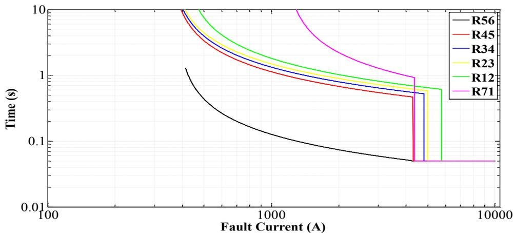
**Fig. 4.20 Time over-current characteristics plot of relays R56, R45, R34, R23, R12 and R71 for Case2 when GTG1 and GTG3 are connected**
