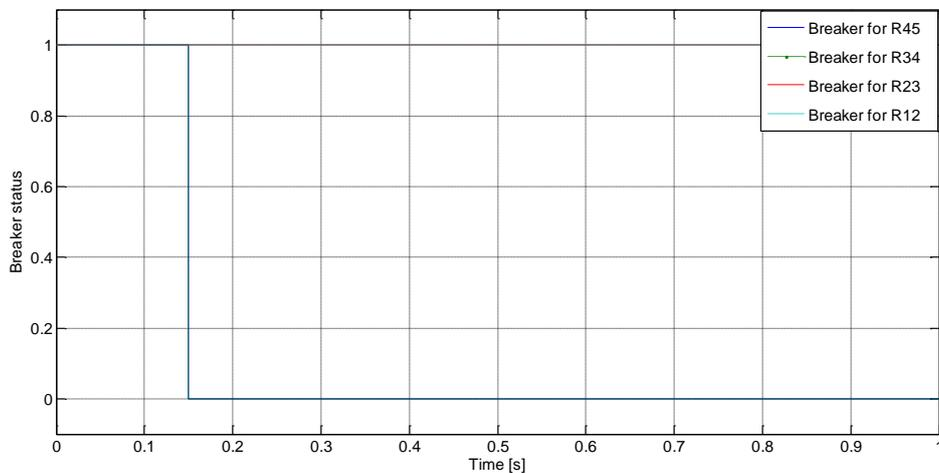
**Fig. 4.26 Status of circuit breaker for a three phase fault in Line45 for Case2 when GTG1, GTG2 and GTG3 are connected and relays are set according to Fig. 4.28**
