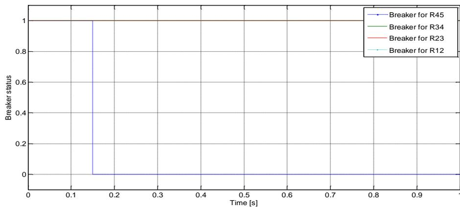
**Fig. 4.30** Status of circuit breaker for a three phase fault in Line45 for Case2 when GTG1, GTG2, GTG3 and WTG are connected and relays are set according to Fig. 4.28
