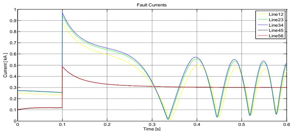
**Fig. 4.25 Fault currents for Case2 when GTG2 and GTG3 are connected**
