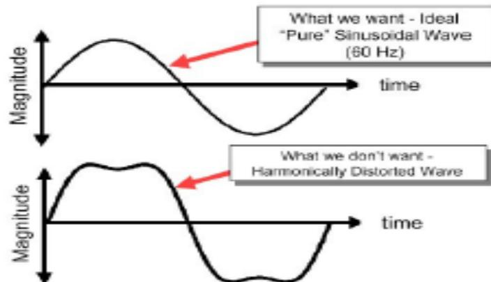
**Fig. 2.6 Comparison between pure sinusoidal wave and distorted wave [17]**
