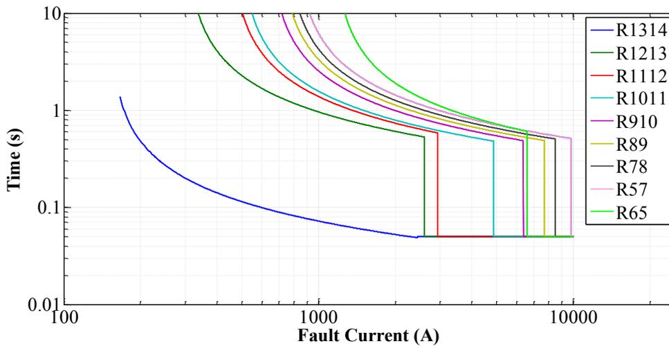
**Fig. 4.8 Time over-current characteristics of relays R1314, R1213, R1112, R1011, R910, R89, R78, R57 and R65 for Case2**
