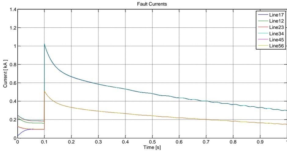
**Fig. 4.29** Fault currents seen by the relays R21, R32, R43, R54 and R65 for a fault in Line45 close to Bus 05 when GTG1, GTG2 and GTG3 are connected
