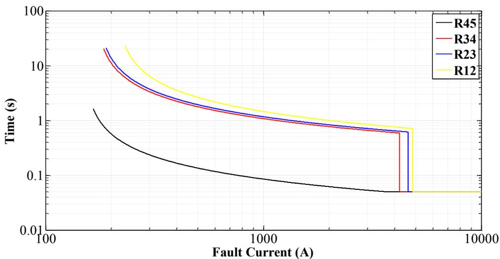
**Fig. 4.16 Time over-current characteristics plot of relays R45, R34, R23 and R12 for Case1.**
