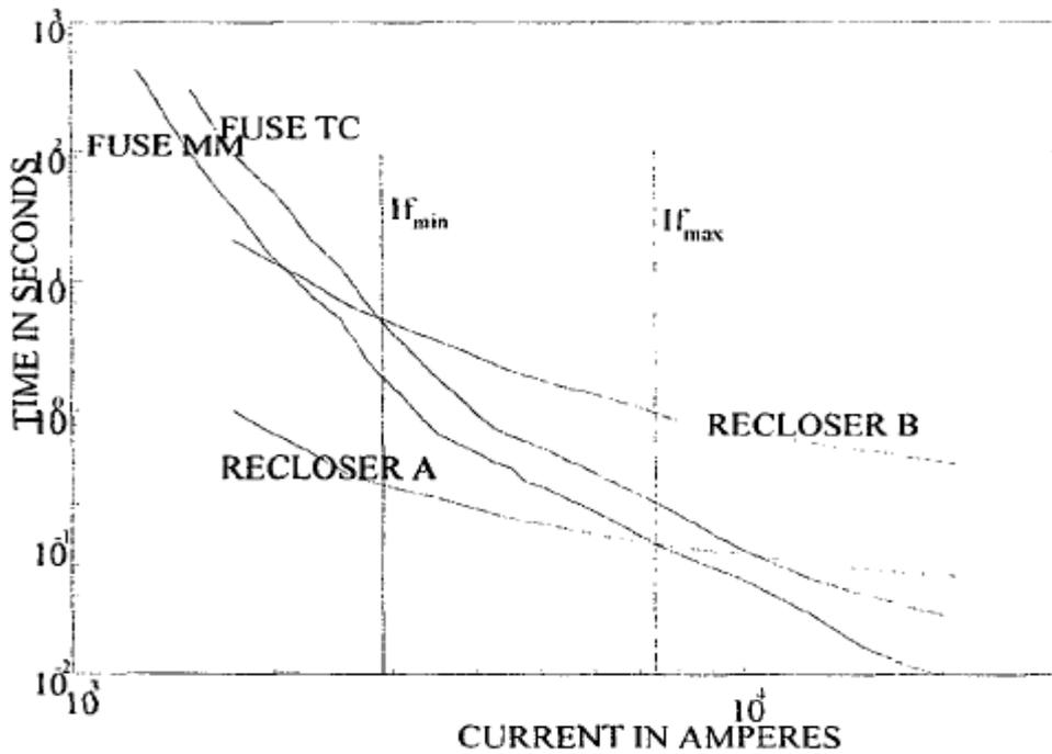
**Fig. 2.13 Coordination between recloser and fuse for the case shown in figure 2.12**
