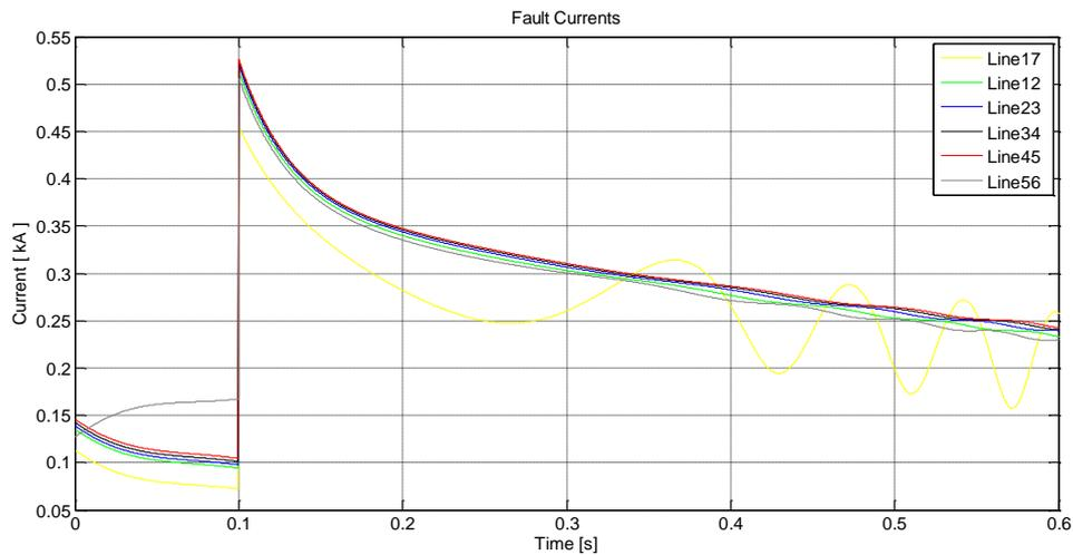
**Fig. 4.22** Fault currents for Case2 when GTG1 and GTG3 are connected
