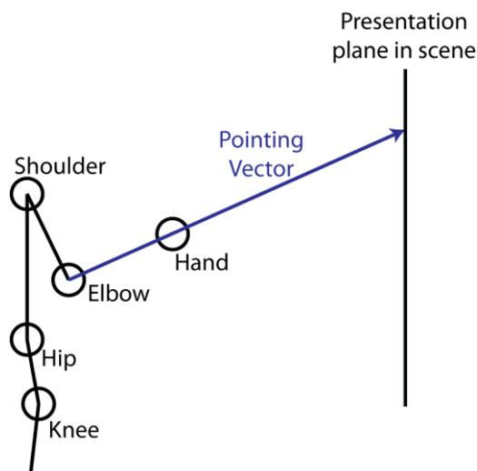
**Illustration 8.1:** Pointing in the skeleton tracking approach happens through creating a vector from elbow, through the hand and onto the presentation plane in the Unity scene.
