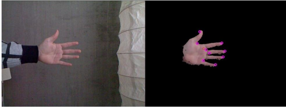
**Illustration 6.4:** Using the code described in this chapter will be able to track a hand and identify fingertips and dips as seen in the image above. The picture on the left is the original input image and the picture on the right is the segmented image. Magenta colored circles are detected tips or dips and the red circle is the centre of mass.
