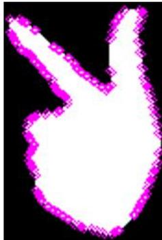
**Illustration 6.3:** Having found all the points along an OpenCV contour produces quite an extensive list of points. All the magenta colored circles are points along the contour, returned by OpenCV.
