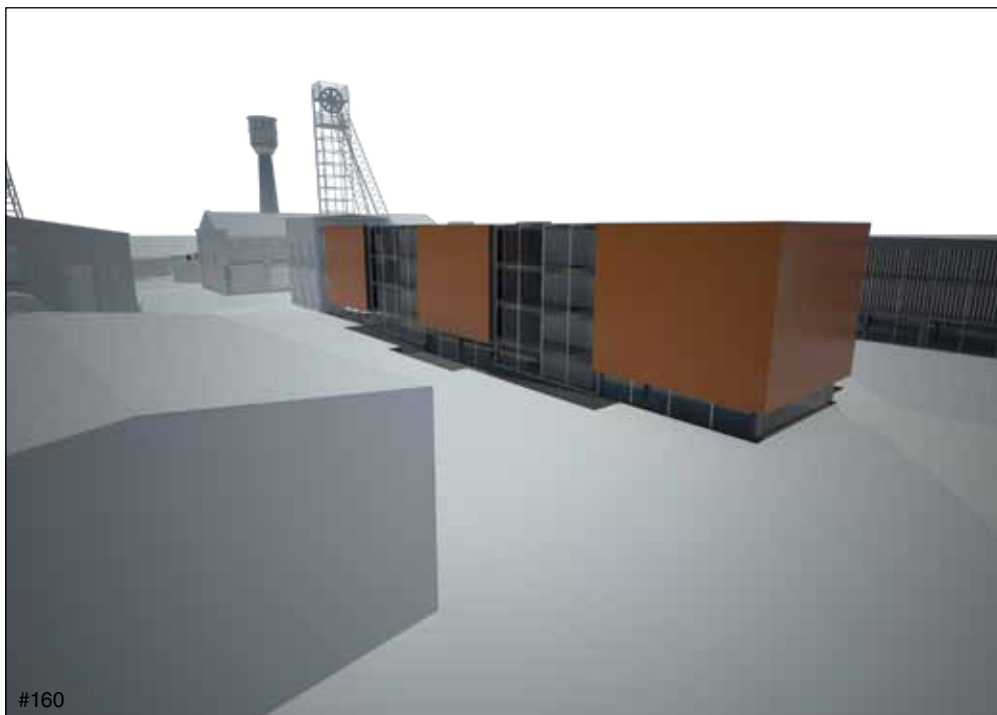
Digital sketch of the office nr1 concept. The building is divided into zones. The office rooms are placed behind perforated facade and the access area with meeting rooms would be covered with glazed facade. The glazed ground floor works as an exhibition area and a visual connection between the two sides of the building. The glazed connection area between the Glowacki shaft and the rest of the building is a fully open high space where the old facade would be visible from out side.
