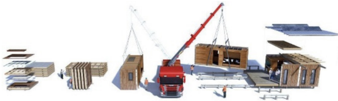
Figure 5: Modular timber construction process [38].
