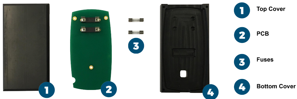
Figure 3.2: The parts for the dummy phone with black coloured covers. For this project 1 is a white color, 4 is a blue color and the two fuses in 3 are pre-installed on the PCB in 2 [5]
