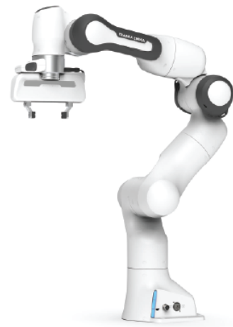
Figure 3.1: The Franka Panda robot arm. [4]
