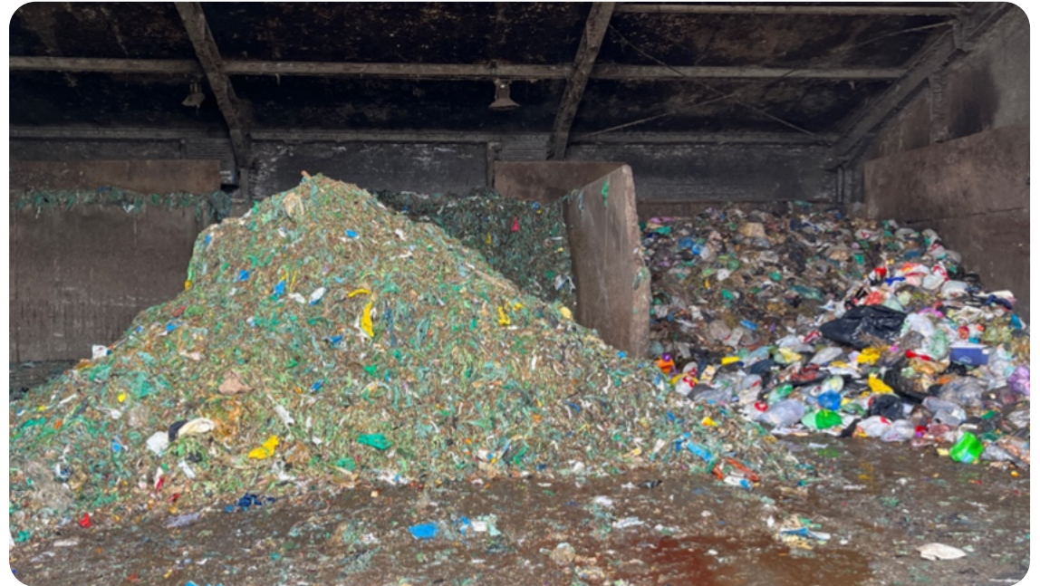
Picture 17: Pile of rejected material (left) and pile of bags full of food waste from households (right) ready to start the journey in the treatment facility to be turned into biogas and compost
