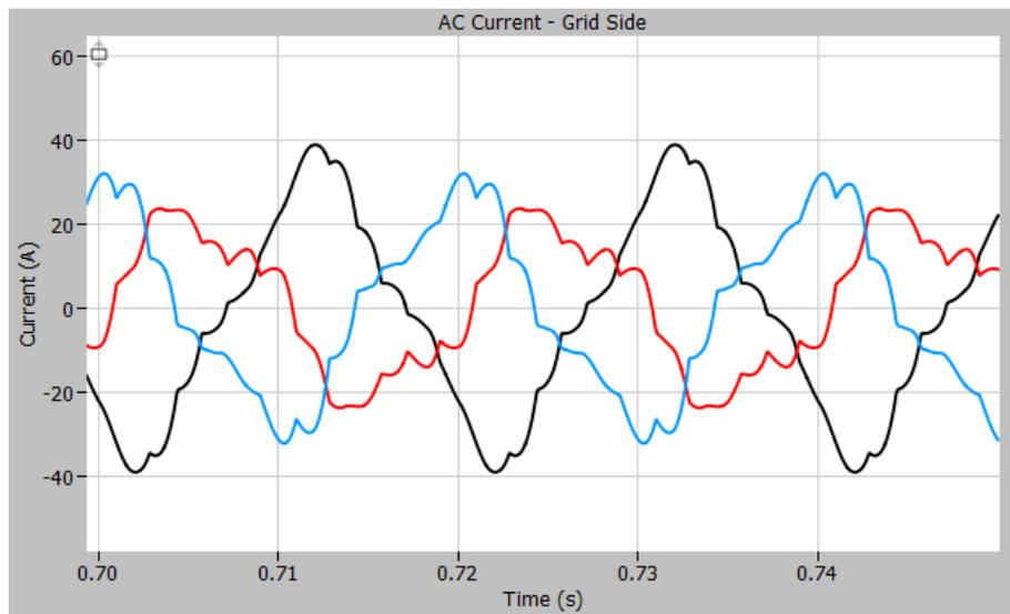
Figure 64: Current measurement with 10% decrease of voltage magnitude phase B without trap filter.
