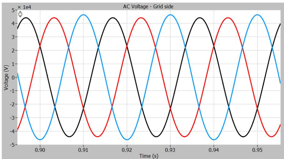
Figure 44: Voltage measurement with 10% decrease of voltage phase B with trap filter.
