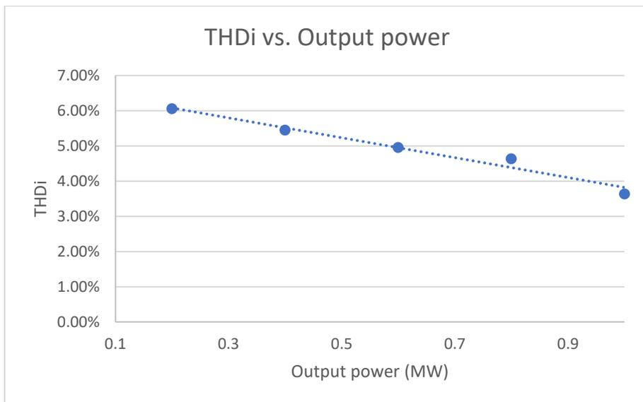
Figure 50: Load variation vs THD for the topology 12-TR, with passive trap filter
