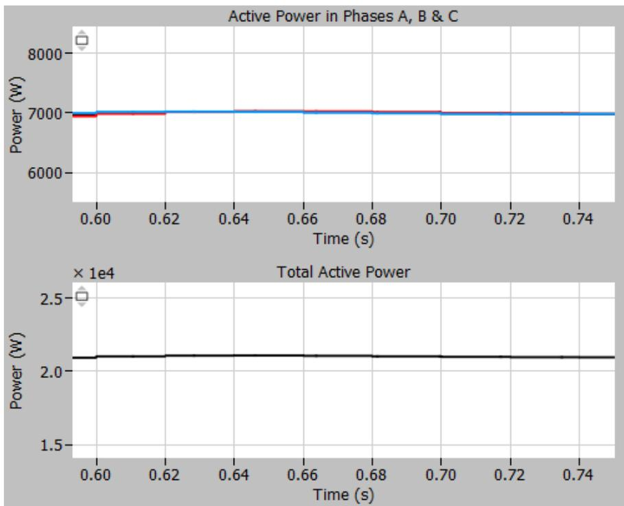
Figure 123: Active Power of Single Phases A, B & C & Total Grid Side Active Power
