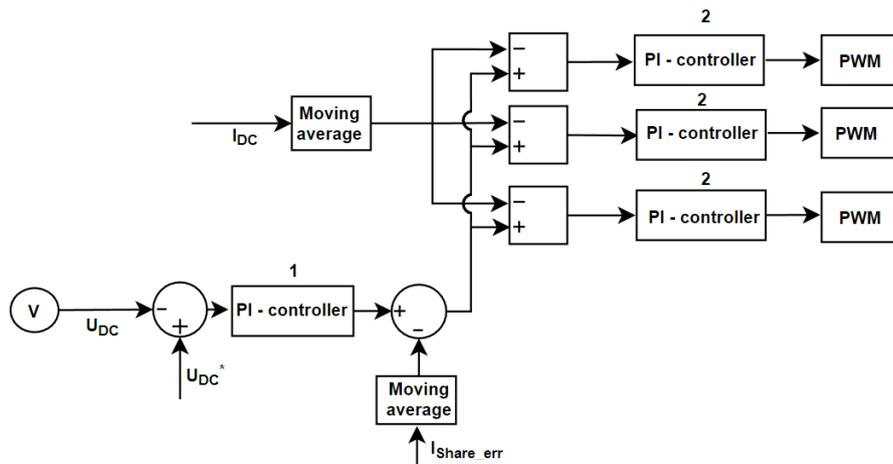
Figure 16: Control diagram for the DC/DC chopper circuit
