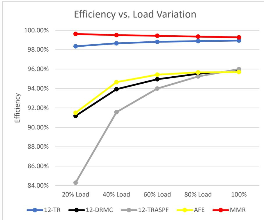
Figure 134: Efficiency at different loading conditions for all the discussed topologies
