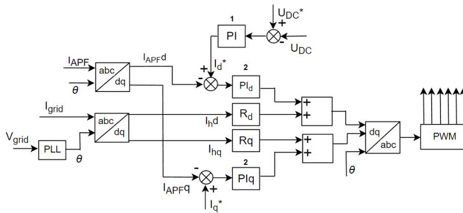
Figure 12: Control Scheme of 12-TRASPF topology
