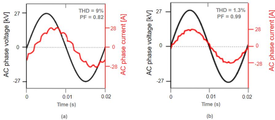
Figure 3: Grid Voltage and Current waveforms when a passive 12-pulse rectifier is connected to the grid (a) without passive harmonic filter (b) with passive harmonic filter
