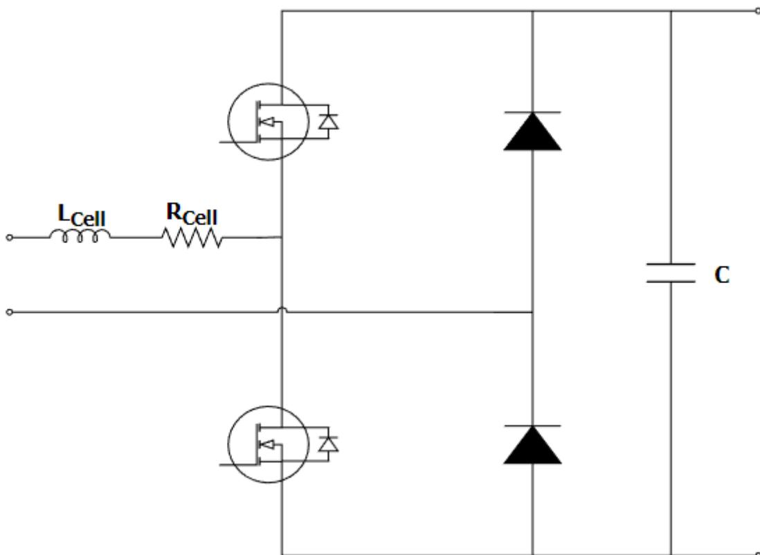
Figure 109: Totem pole bridgeless boost converter configuration (AC/DC Stage)
