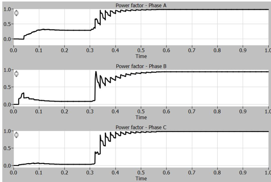
Figure 47: Power Factor of Phases A, B, and C with a decrease of 10% voltage magnitude of phase B with trap filter
