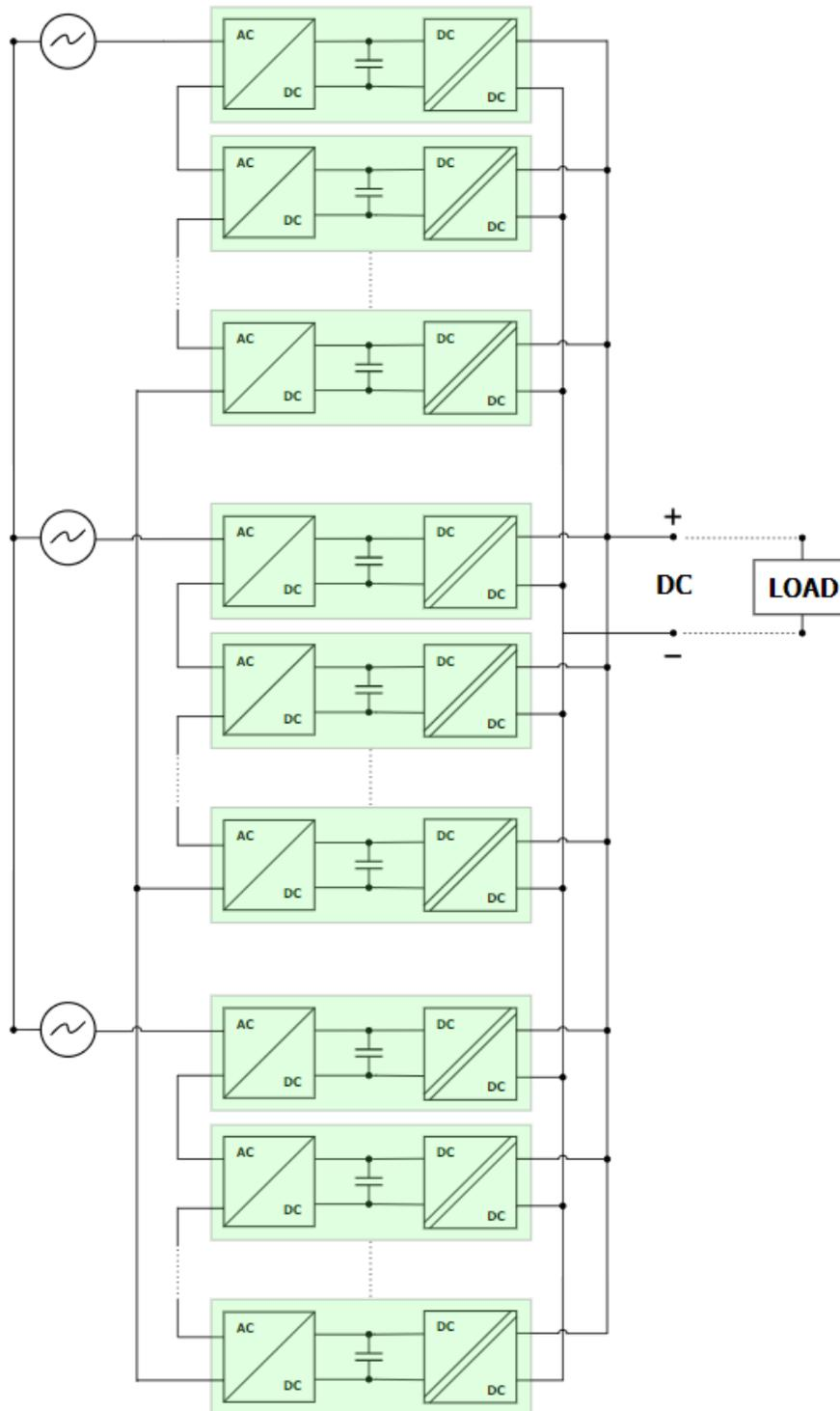
Figure 107: Circuit Diagram of Modular Multicell Rectifier (MMR)
