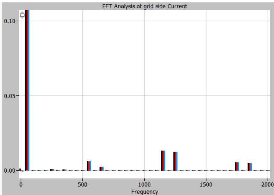
Figure 62: Harmonic spectrum of grid side current with Trap Filters. Normalized at fundamental frequency of 50 Hz
