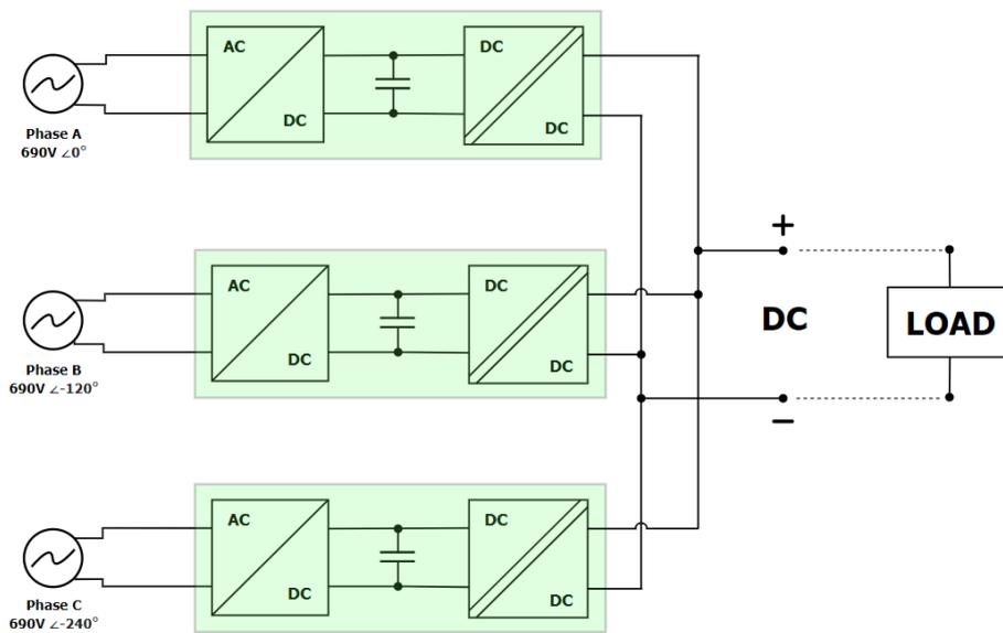
Figure 113: MMR Topology used in the Simulations
