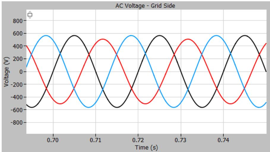
Figure 120: Grid Side Voltages under unbalanced condition
