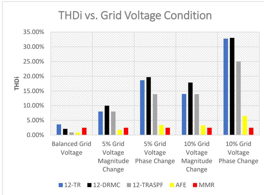
Figure 131: THD at different unbalance types
