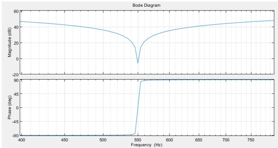
Figure 19: Bode Diagram of the trap filter for the 11th Harmonic (550 Hz)
