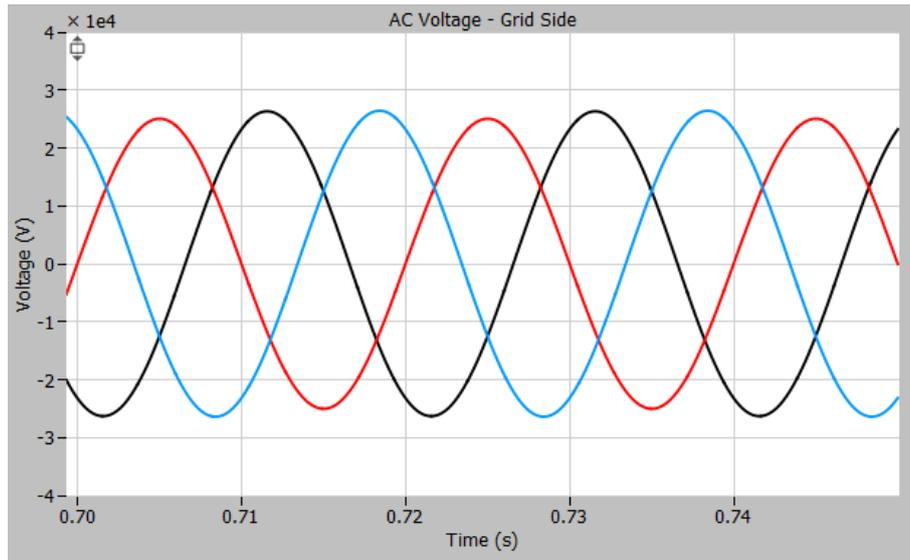
Figure 65: Voltage measurement with 10% decrease of voltage magnitude phase B without trap filter.
