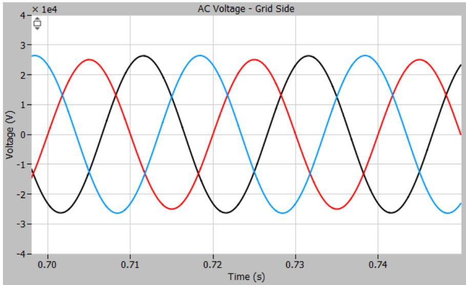
Figure 70: Voltage measurement with 10% decrease of voltage phase B without trap filter
