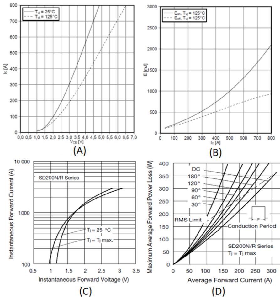
Figure 78: The conduction and switching loss for the IGBT in figure A and figure B, similarly for the diode in figure C and figure D
