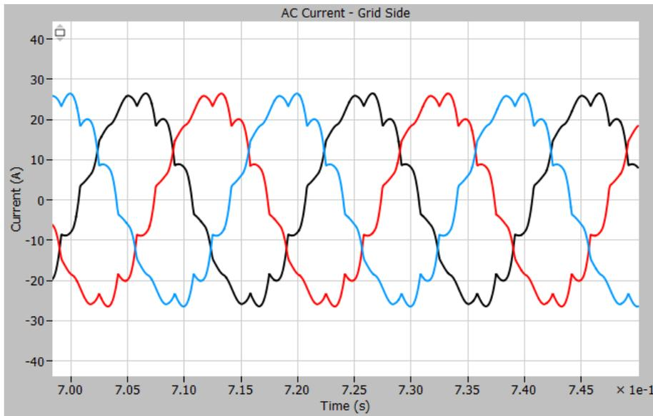
Figure 58: Current measurement on the grid side for 12-DRMC
