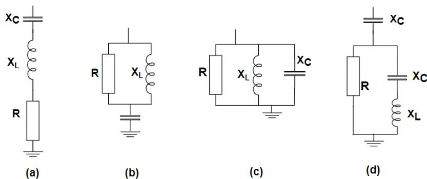
Figure 18: Series, high-pass, band-pass, C-type respectively
