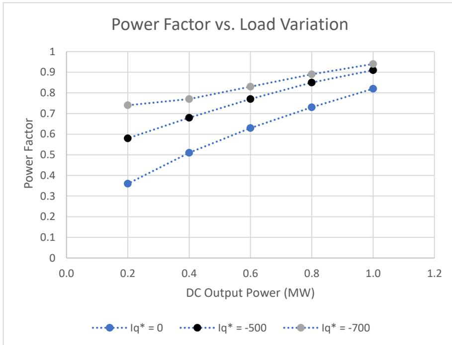
Figure 90: Trend in PF for increasing load variation percentage for 3 different values of 'Iq\*'
