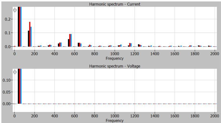
Figure 40: Harmonic spectrum of 10% decrease of voltage magnitude. Normalized to fundamental frequency of 50 Hz
