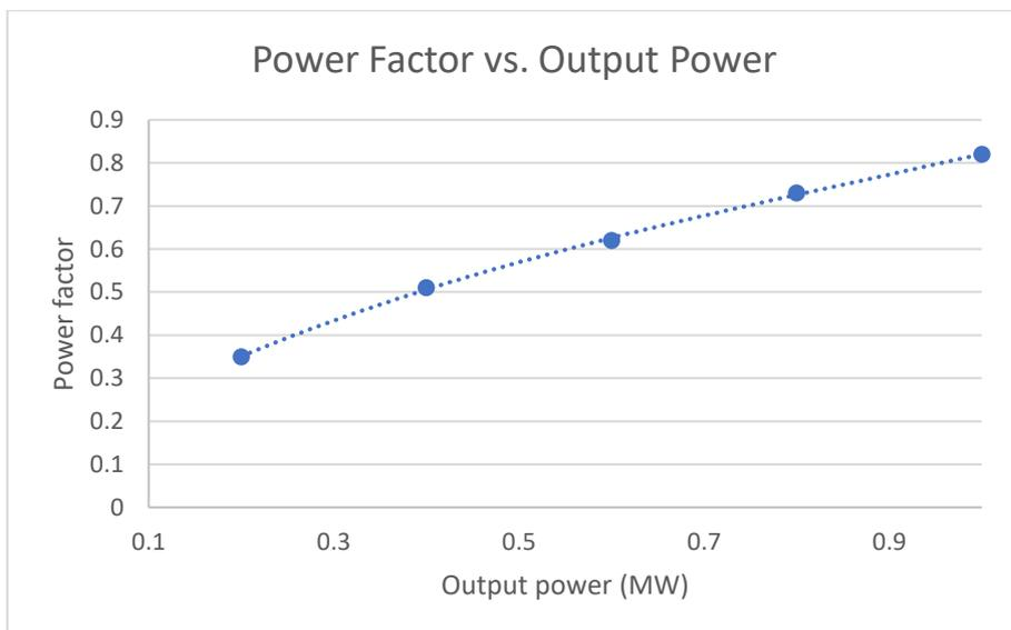
Figure 49: Output power vs power factor for 12-TR without trap filter
