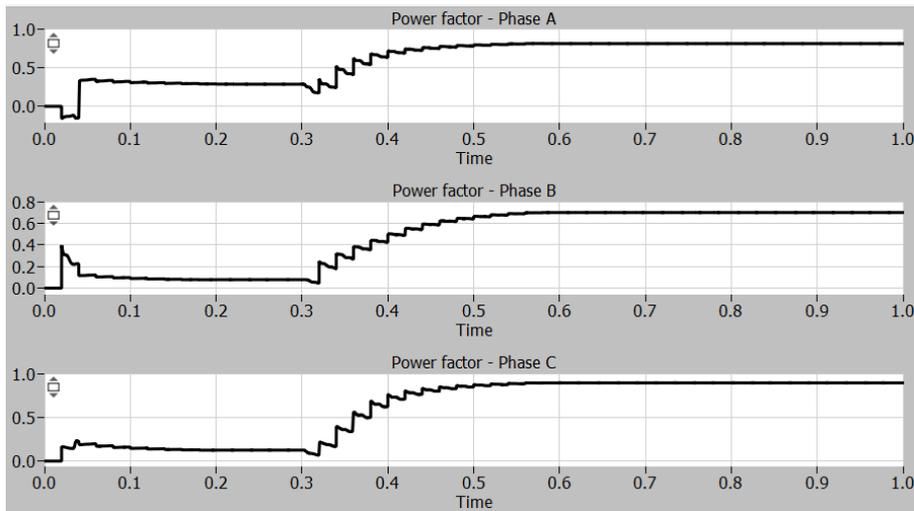
Figure 42: Power Factor of Phases A, B, and C with a decrease of 10% voltage magnitude of phase B
