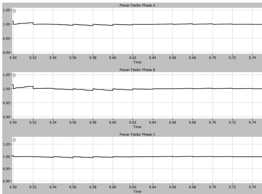
*Figure 124: Single phase (A, B, C) power factor during the unbalanced grid.*
