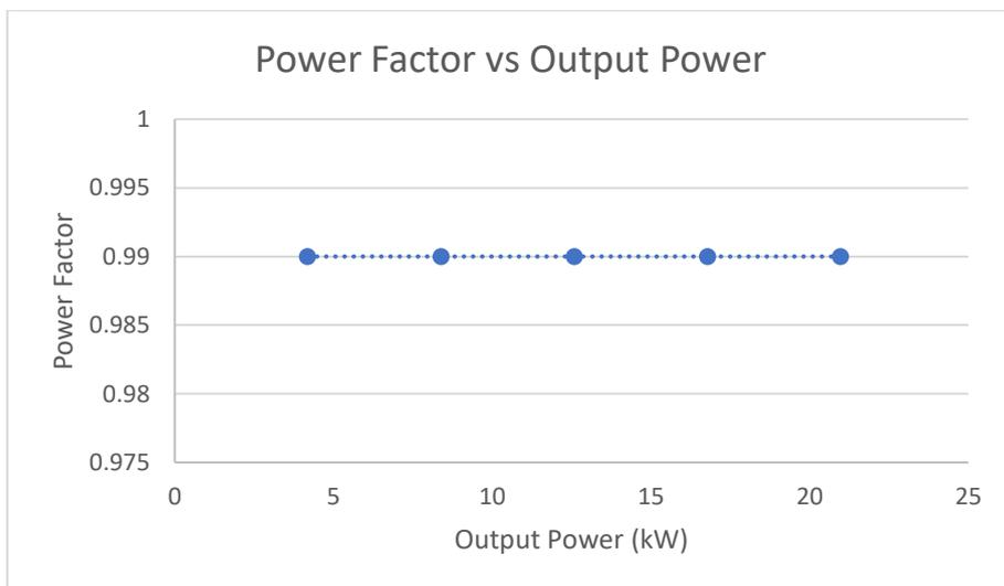
Figure 126: Power Factor (Phase A) vs. Load variation for the MMR Topology
