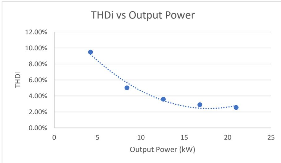
Figure 125: THD vs. Output Power for the MMR Topology
