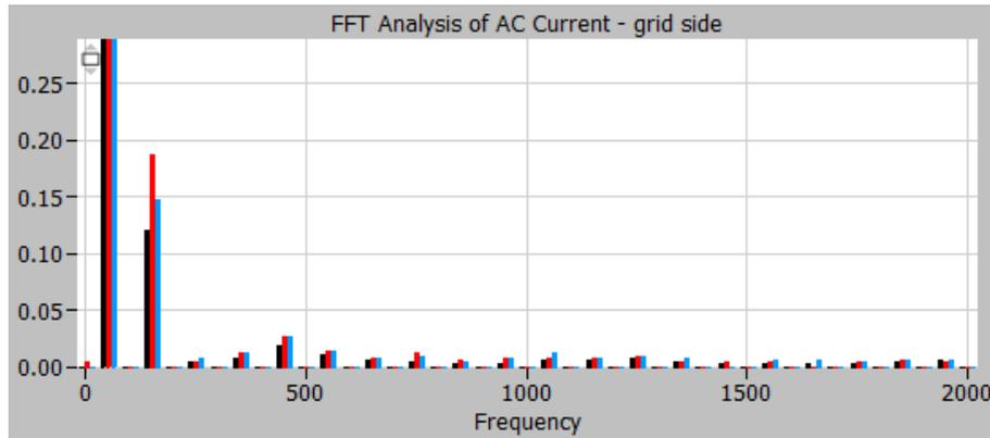
Figure 87: FFT Analysis of Grid side Current of 12-TRASPF with 10% voltage magnitude decrease in phase B.
