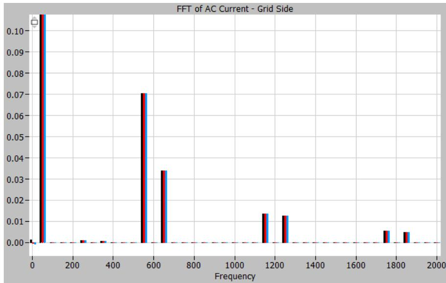
Figure 59: Harmonic spectrum of grid side current, without trap filter. Normalized at fundamental frequency of 50 Hz
