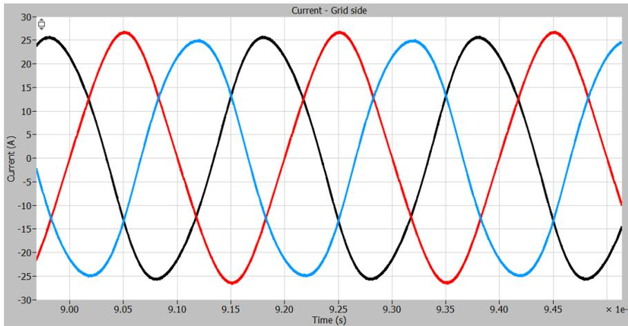
Figure 100: Current measurement with 10% decrease of voltage magnitude of a single-phase.
