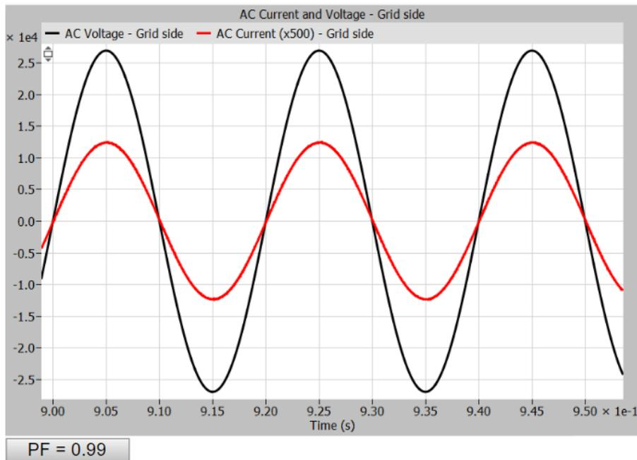
Figure 99: Current (x500) and voltage – grid side – With power factor of 0.99
