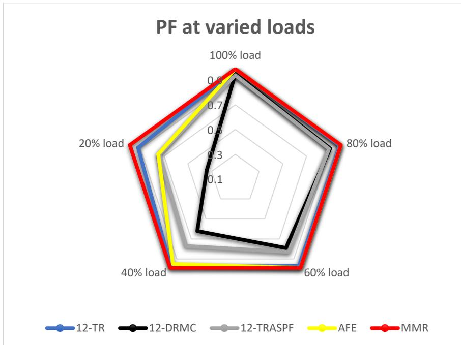
*Figure 132: Power Factor at different load variations*
