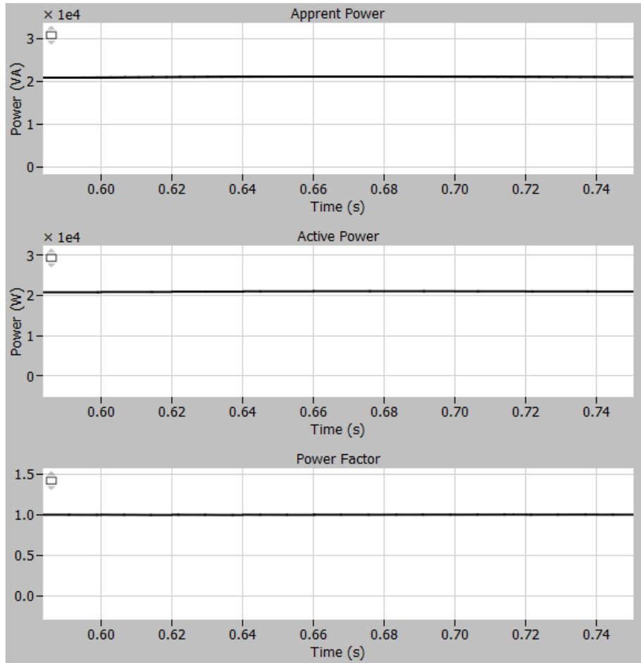
Figure 119: Apparent Power, Active Power & Power Factor from Grid Side for MMR
