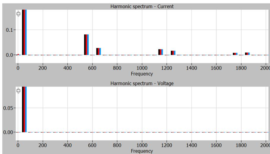
Figure 31: Harmonic spectrum of the current & voltage harmonics on the grid side. Normalized at fundamental frequency of 50 Hz
