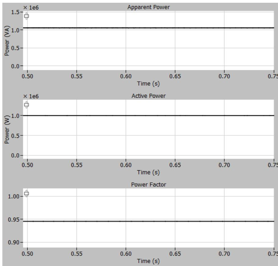
Figure 63: Plots of Apparent power (S), Active power (P) and Power factor (PF).
