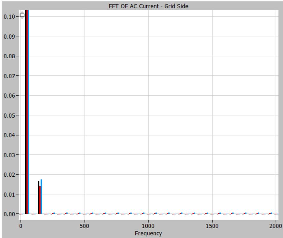
Figure 122: Harmonic spectrum during the unbalance for MMR topology. Normalized at the fundamental frequency of 50 Hz
