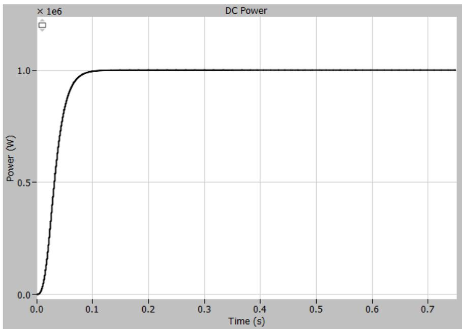
Figure 57: Power at the DC side from 12-DRMC
