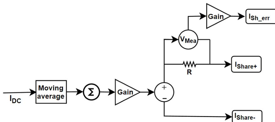
Figure 17: Control diagram for the current sharing.
