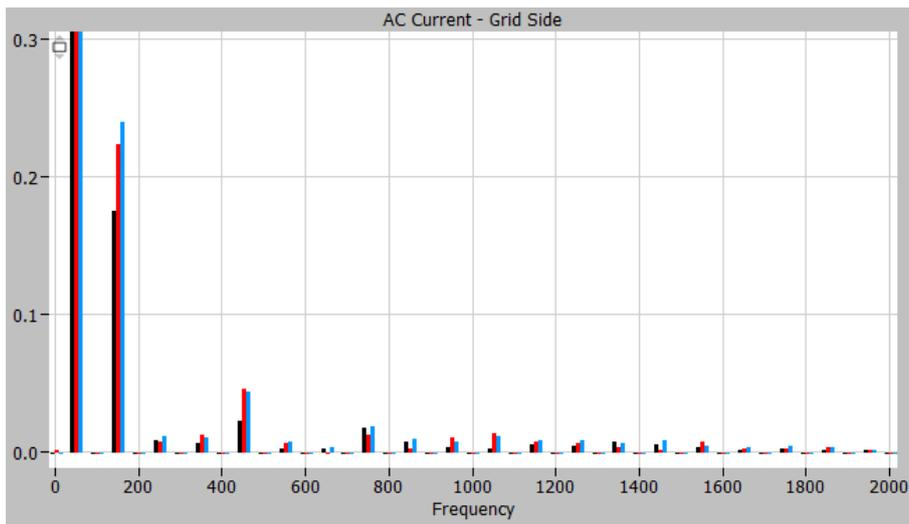
Figure 71: Grid Side Current Harmonic spectrum with 10% magnitude decrease in phase B with trap filters. Normalized to fundamental frequency of 50 Hz
