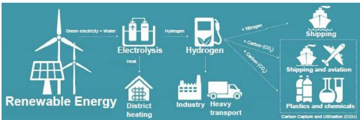
Figure 2: P2X process from renewable to heat and hydrogen [3].
