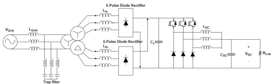
Figure 6: 12-Pulse Diode Rectifier with Multi-phase Chopper
