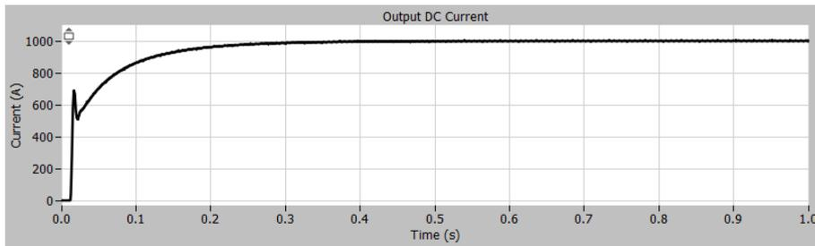
Figure 81: Output DC Current of 12-TRASPF converter
