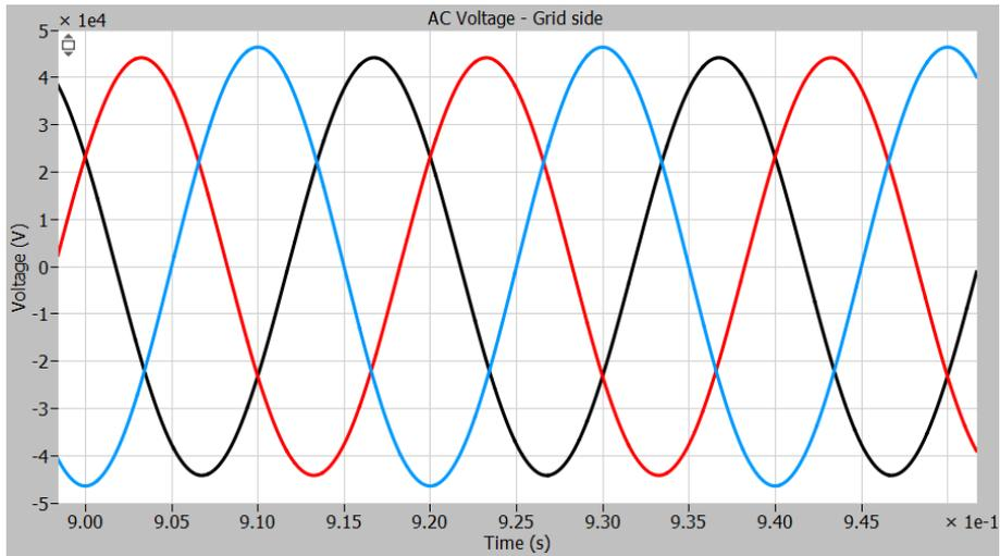
Figure 39: Voltage measurement with 10% decrease of voltage phase B without trap filter.
