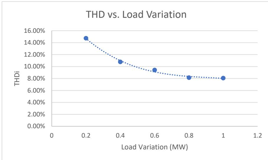
Figure 74: Load Variation vs THD for 12-DRMC
