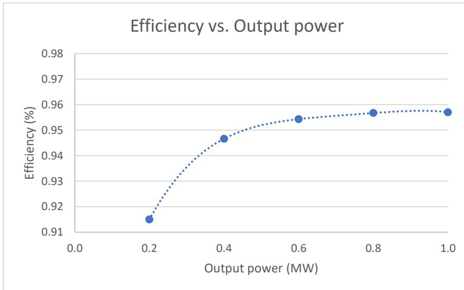
Figure 106: Efficiency vs power for AFE
