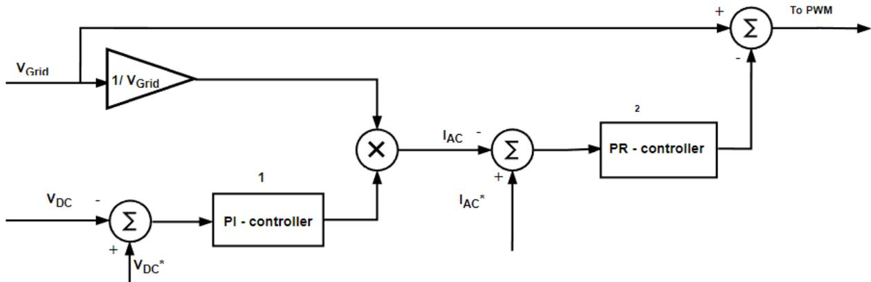
Figure 110: Control technique for AC/DC Converter
