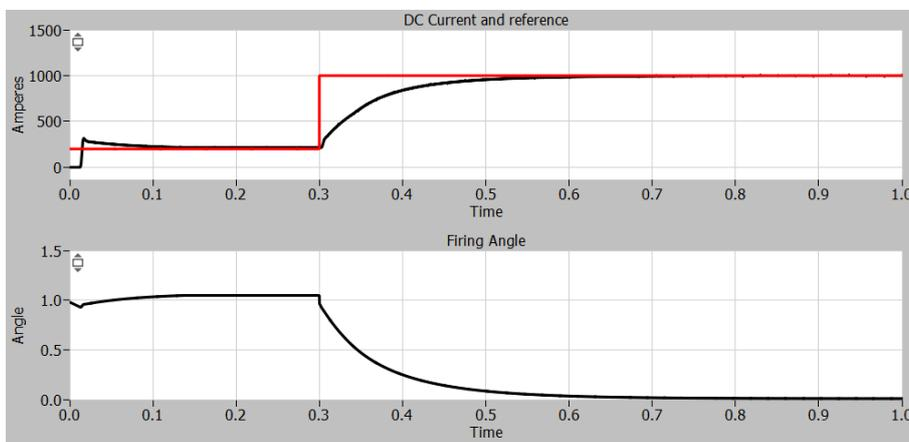
Figure 28: The reference current (Red) and DC current (Black) and the firing angle of the 12-TR with passive trap filter
