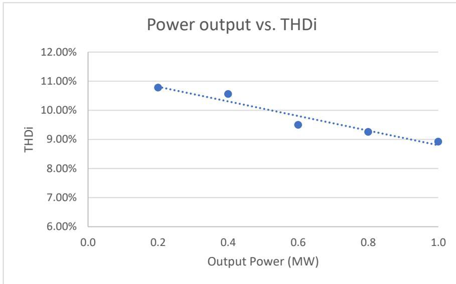
Figure 48: Power output vs THDi for the topology 12-TR without trap filter
