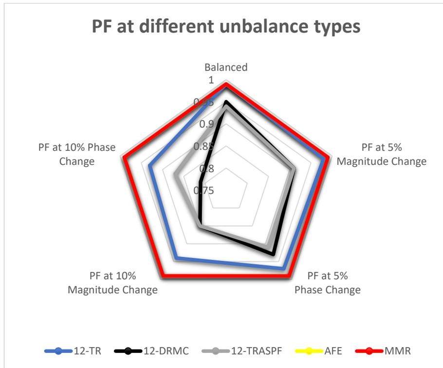
Figure 130: Radar Graph showing Power Factor of all the discussed topologies at different unbalance types
