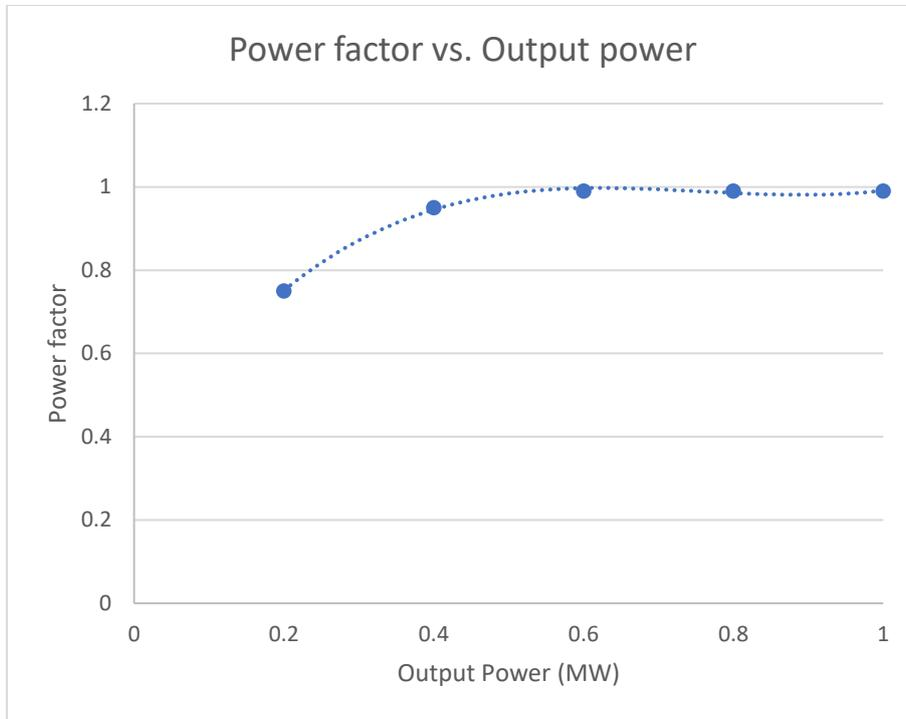
*Figure 105: Load Variation vs Power Factor for AFE*
