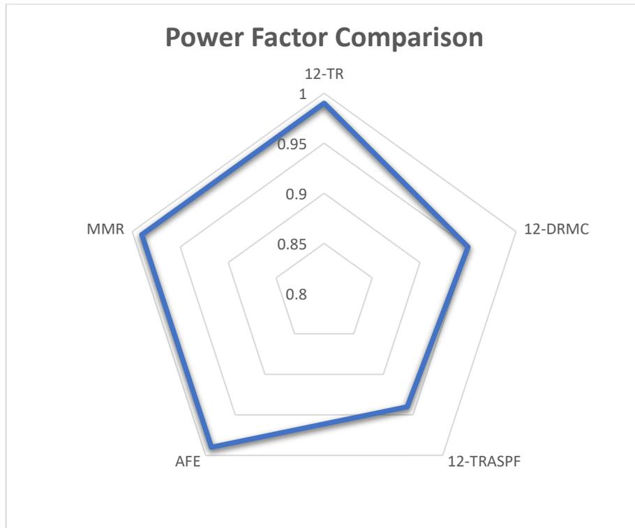
*Figure 129: Radar Graph showing Power Factor of different topologies*
