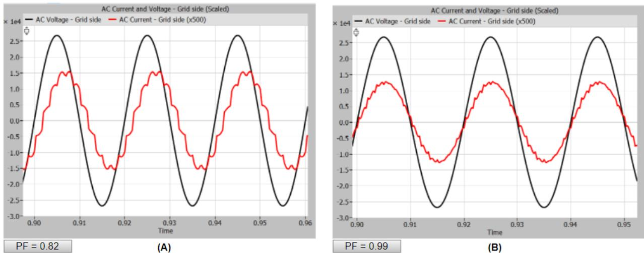
Figure 37: Current and voltage – grid side – (A) depict the waveform with PF of 0.82 while (B) shows with 0.99
