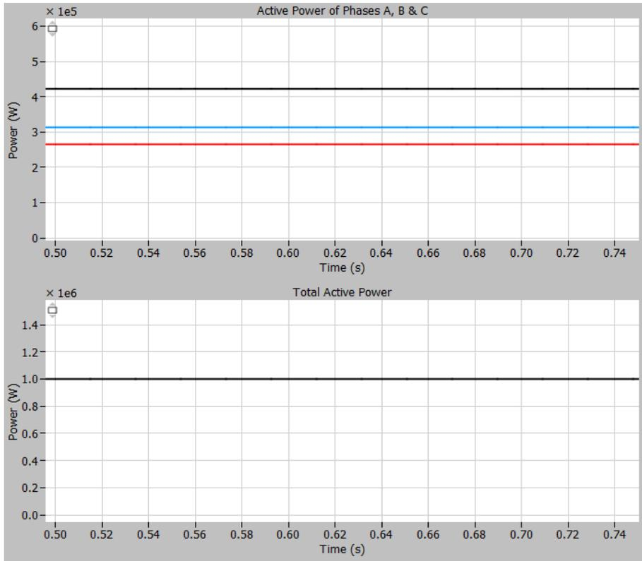
Figure 67: Active Power of Single Phases A, B & C & Total Grid Side Active Power
