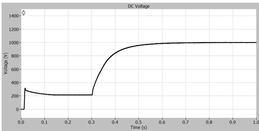
Figure 26: DC voltage from the 12-TR with passive trap filter
