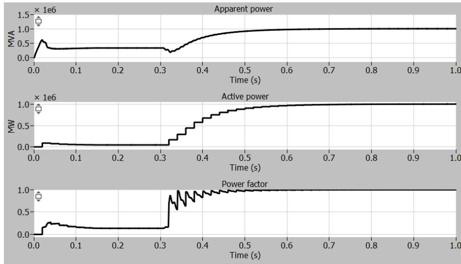
Figure 36: Graphs of Apparent power (S), Active power (P) and Power factor (PF) with passive trap filter.
