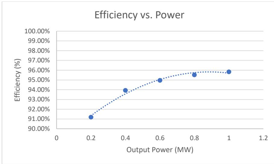
Figure 79: Efficiency vs Power graph for 12-DRMC
