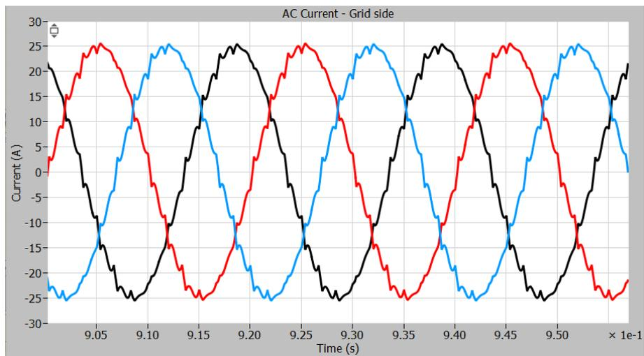
Figure 33: Measurement current on the grid side with passive trap filter
