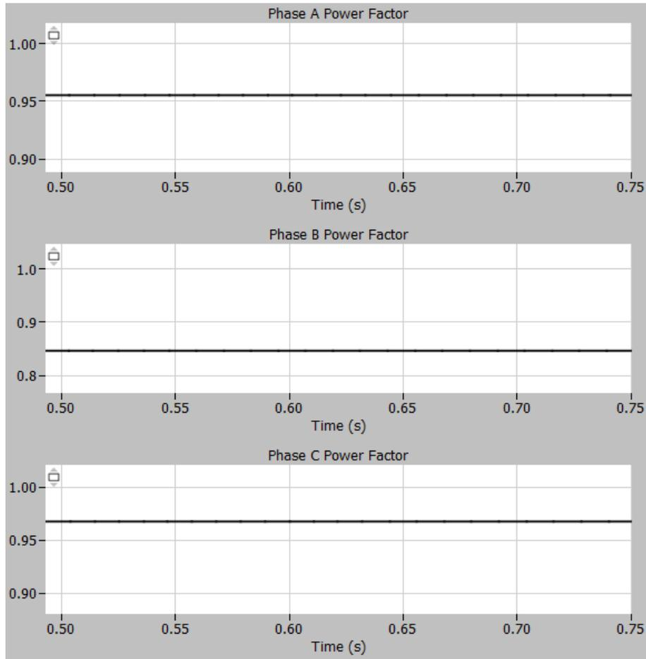
Figure 73: Power Factor of Phases A, B & C
