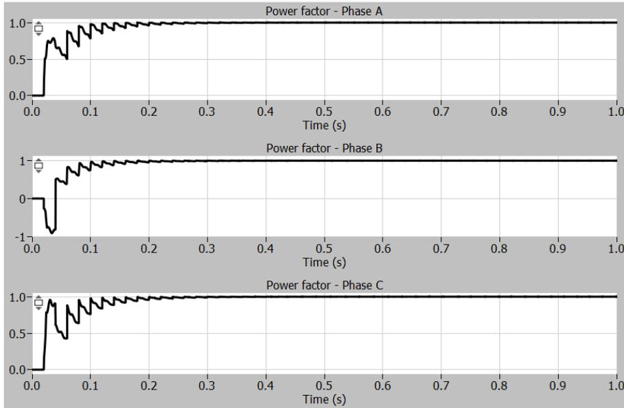
Figure 103: Single phase (A, B, C) power factor with 10% decrease of voltage magnitude.
