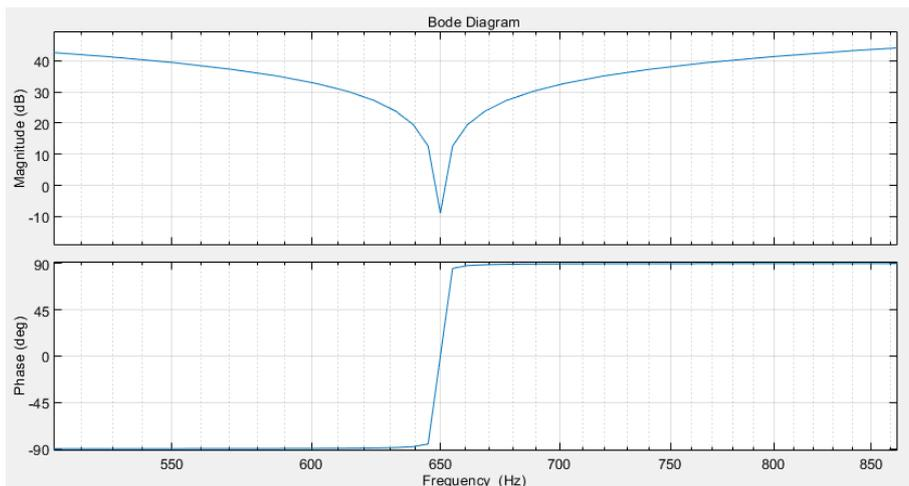
Figure 20: Bode Diagram of the trap filter for the 13th Harmonic (650 Hz)
