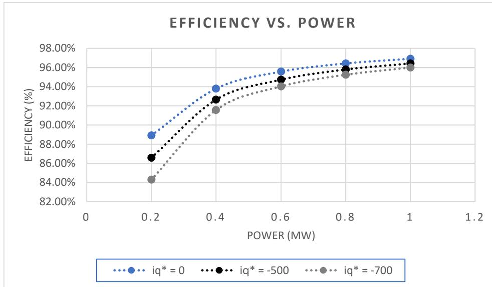
Figure 92: Efficiency vs Power for 12-TRASPF with various reactive compensation
