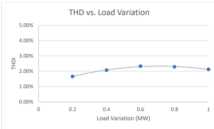
Figure 76: Load Variation vs THD for 12-DRMC with Filter
