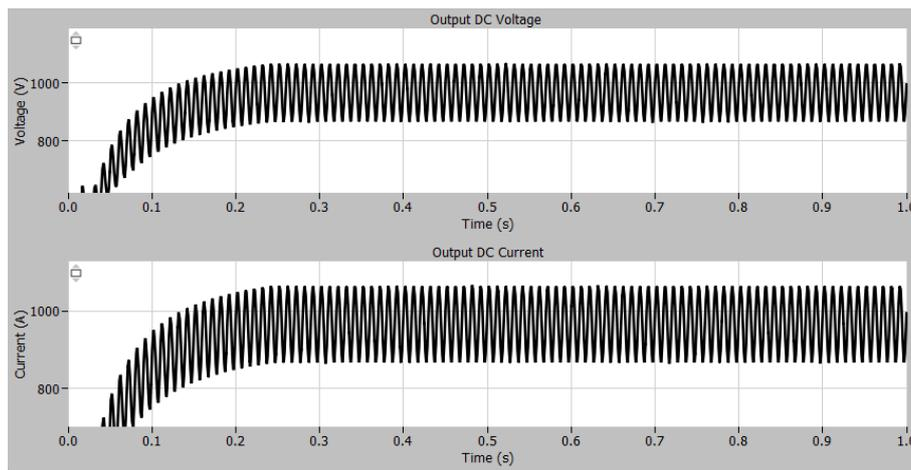
Figure 88: Output DC Voltage (upper plot) and Output DC Current (lower plot) with 10% Grid Volt. magnitude unbalance
