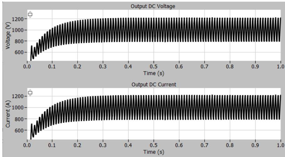
Figure 89: Output DC Voltage (upper plot) and Output DC Current (lower plot) with 10% Grid Phase Volt. unbalance
