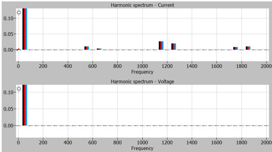
Figure 35: Harmonic spectrum of the current & voltage harmonics on the grid side with passive trap filter. Normalized to fundamental frequency of 50 Hz
