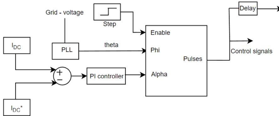
Figure 5: Control diagram of the 12-TR
