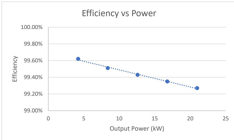
Figure 127: Efficiency vs Power graph for MMR
