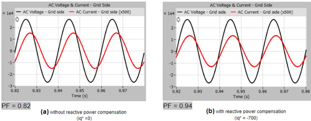
Figure 85: Grid Side Phase Voltage & Grid Side Phase Current (x500) when (a) ' $i_q^* = 0$ ' and (b) ' $i_q^* = -700$ '
