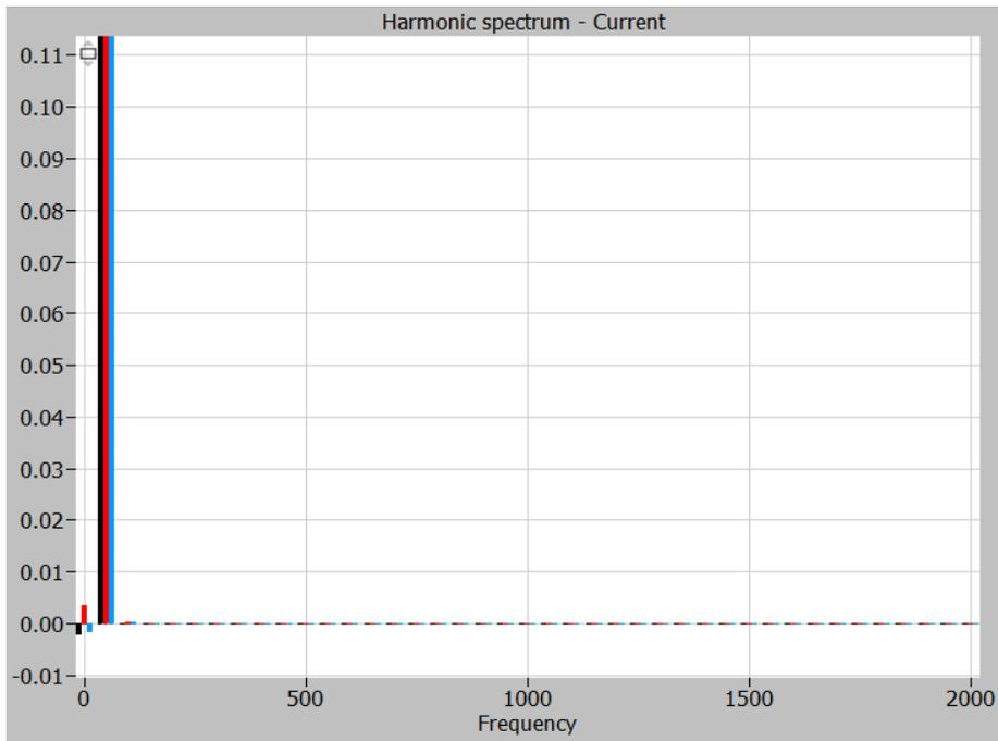
Figure 97: Harmonic spectrum of the current harmonics on the grid side. (Normalized with respect to the fundamental frequency of 50 Hz with magnitude value of 1)
