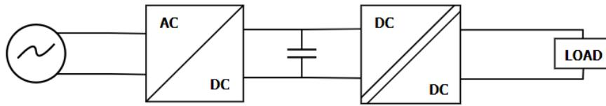
Figure 108: Single Cell construction in the MMR Topology
