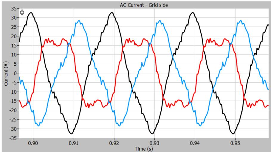
Figure 43: Current measurement with 10% decrease of voltage phase B with trap filter.
