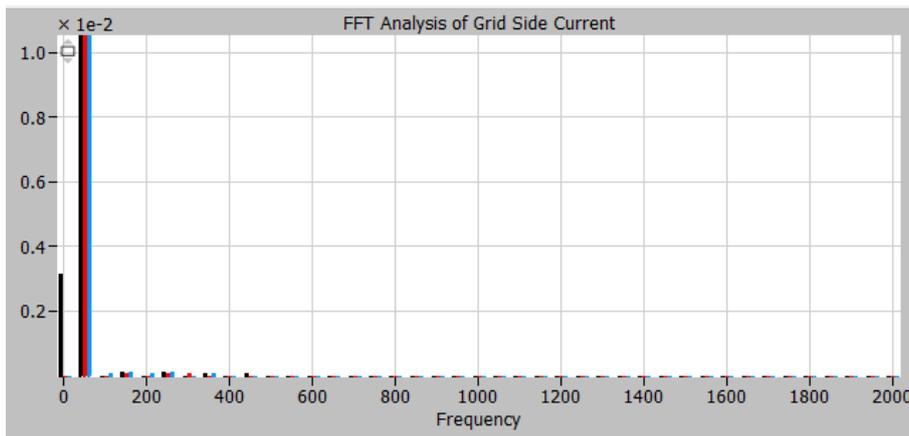
Figure 83: FFT Analysis of Grid side Current of 12-TRASPF with harmonic compensation and  $i_q^* = 0$
