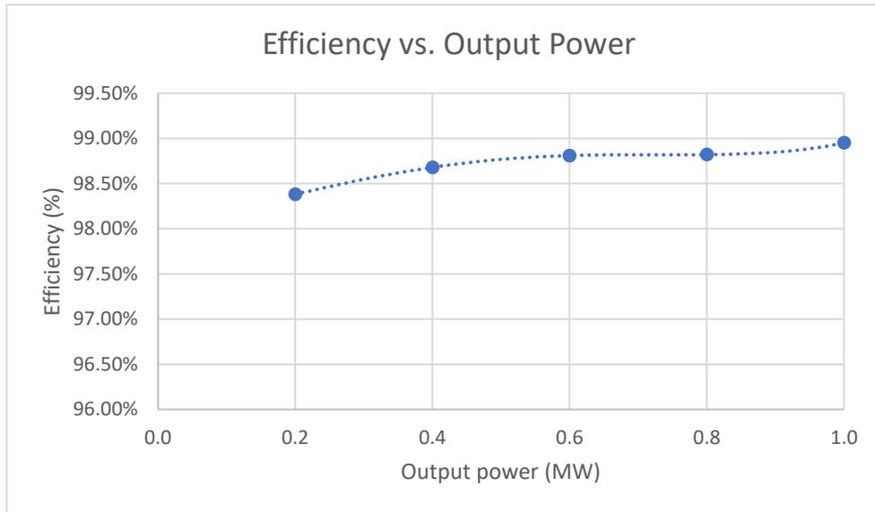
Figure 53: Efficiency vs power graph for 12-TR
