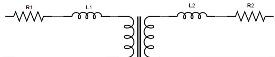
Figure 24: Simplistic Equivalent Circuit of a Transformer
