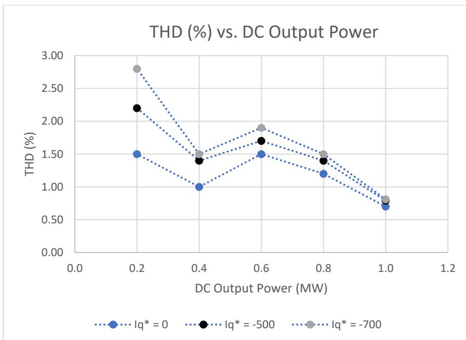
Figure 91: THD (%) vs. Active Power (MW) for 3 different values of 'Iq\*'
