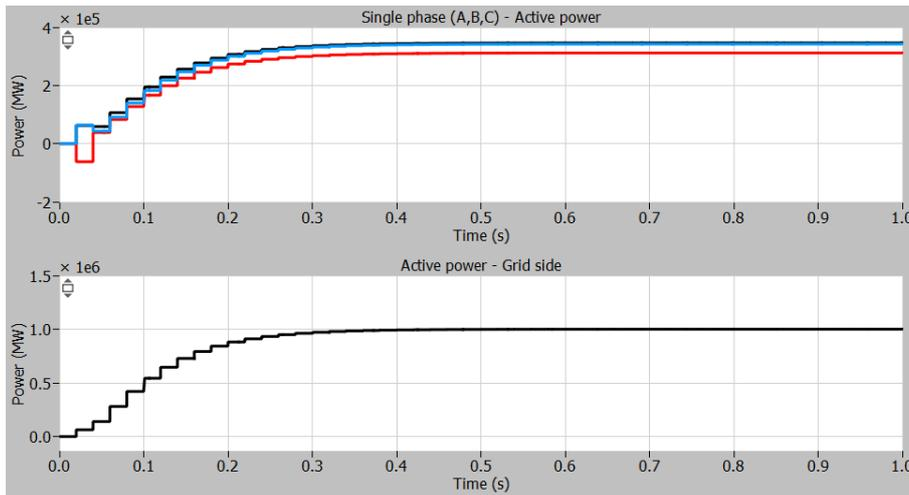
Figure 102: Single phase (A, B, C) and combined active power measurement, with a 10% decrease of phase B voltage magnitude
