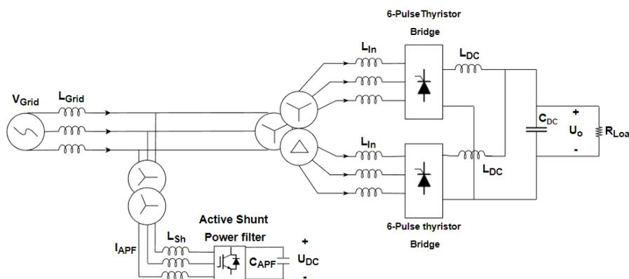
Figure 10: 12-TRASPF Hybrid Filter Topology
