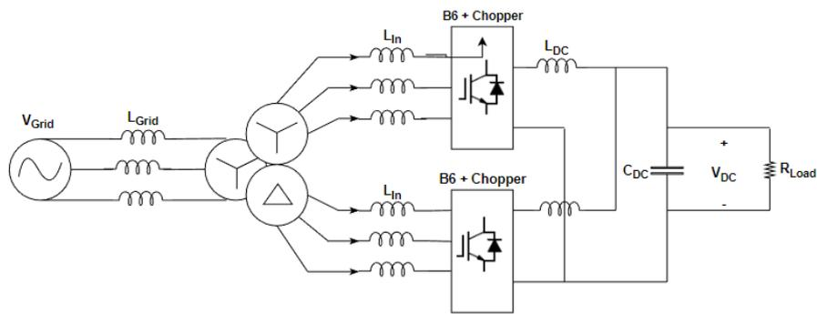
Figure 13: Active Front End Rectifier, with B6+Chopper.
