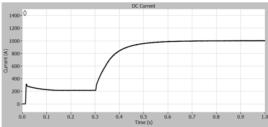
Figure 25: DC current from the 12-TR with passive trap filter
