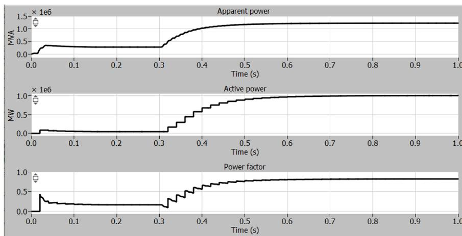
*Figure 32: Graphs of Apparent power (S), Active power (P) and Power factor (PF).*
