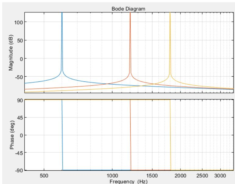
Figure 21: Bode Diagrams of Resonant controllers tuned to 12<sup>th</sup>, 24<sup>th</sup> & 36<sup>th</sup> order harmonic frequencies
