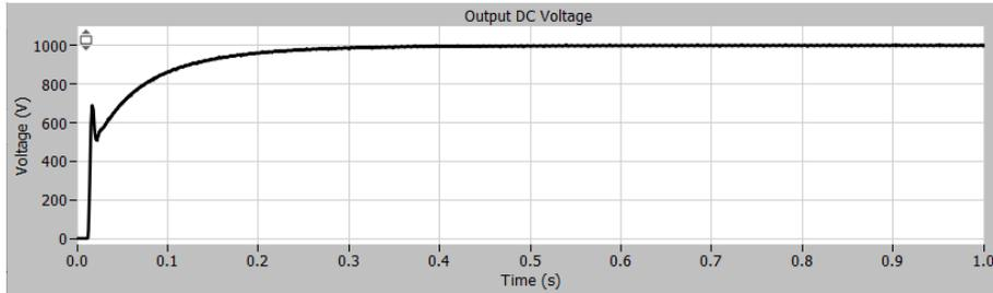
Figure 80: Output DC Voltage of 12-TRASPF converter
