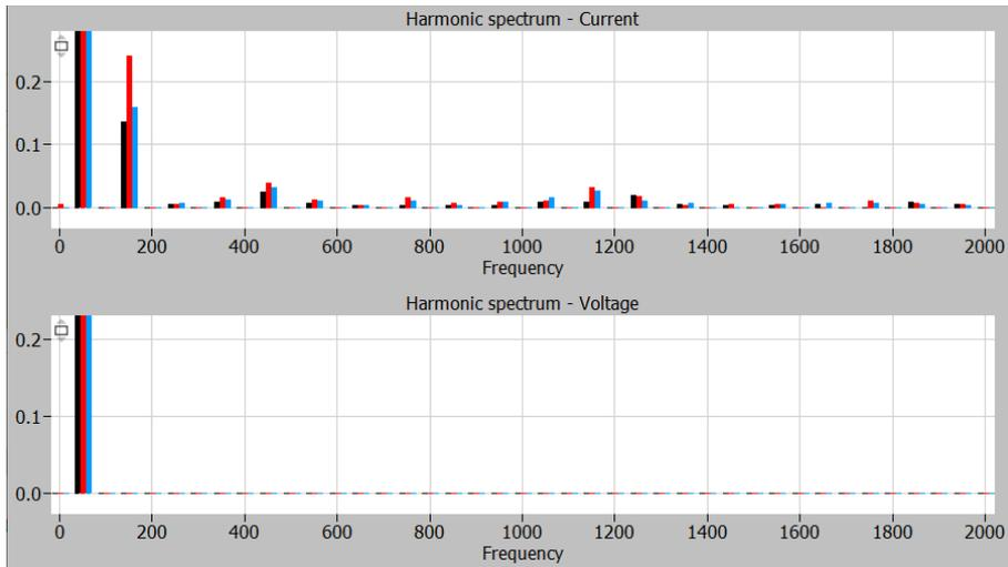
Figure 45: Harmonic spectrum of current and voltage with 10% decrease of voltage magnitude and trap filter. Normalized at fundamental frequency of 50 Hz
