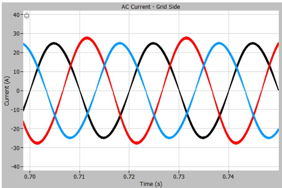
Figure 121: Grid side currents under unbalanced condition
