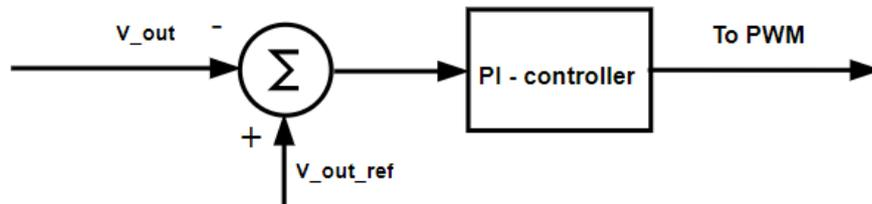
*Figure 112: Control technique for DC/DC Converter*
