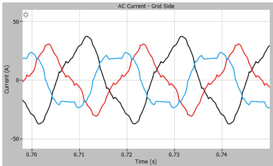
*Figure 69: Current measurement with 10% decrease of voltage phase B with trap filter*
