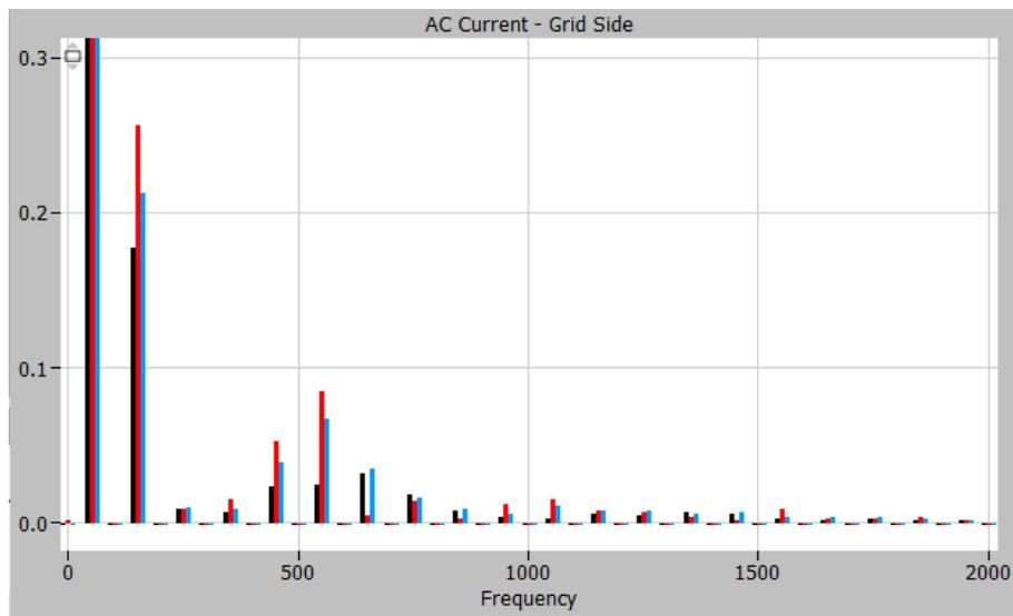
Figure 66: Grid Side Current Harmonic spectrum with 10% magnitude decrease in phase B. Normalized to fundamental frequency of 50 Hz
