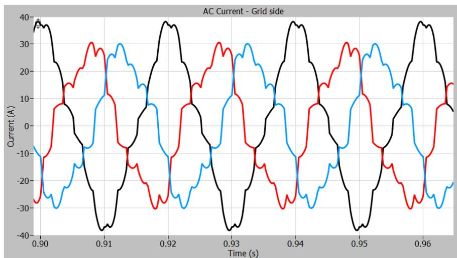
Figure 38: Current measurement with 10% decrease of voltage phase B without trap filter.
