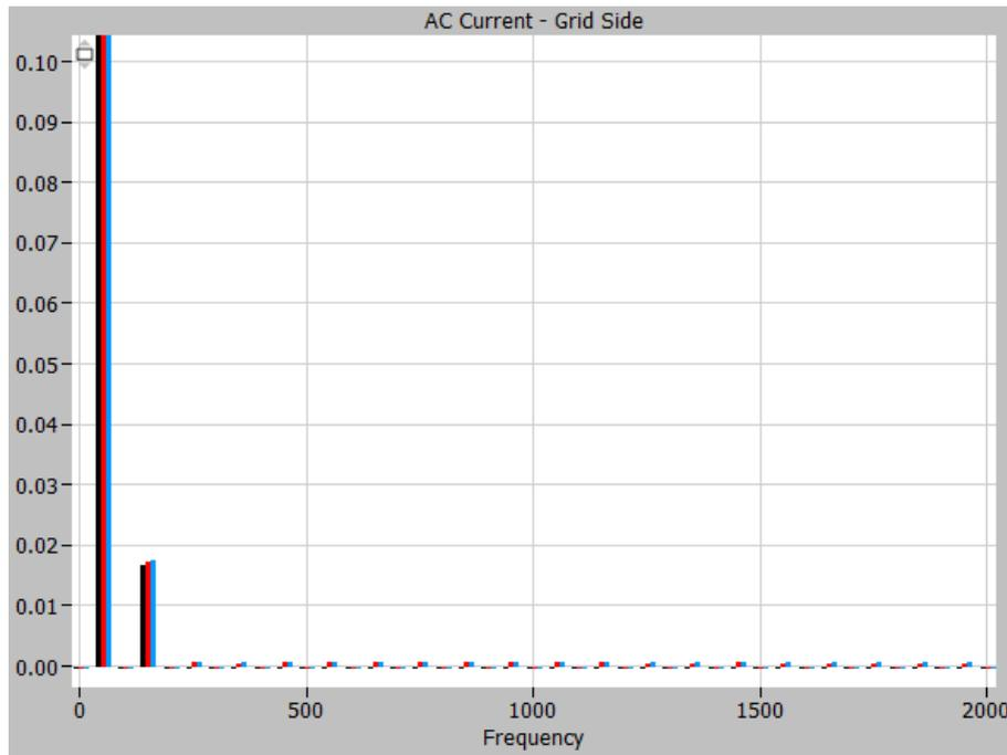
Figure 118: Harmonic Analysis of the Grid Side Current
