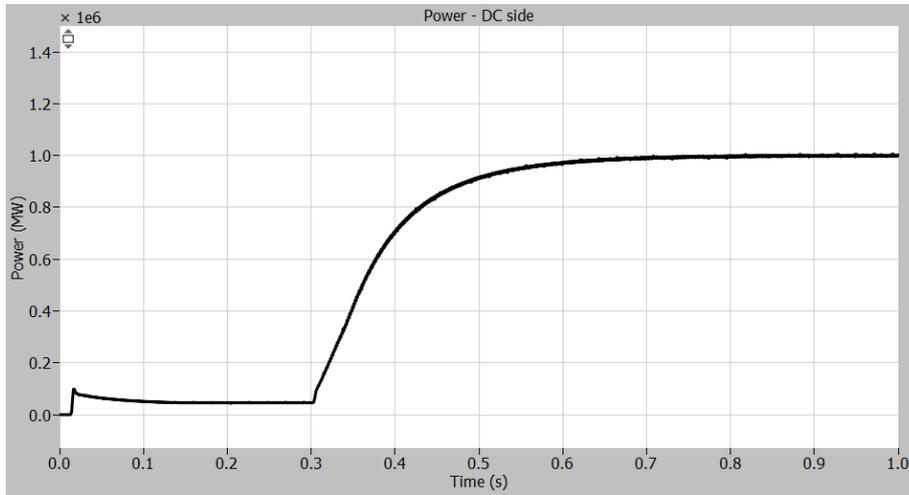
Figure 27: Power at the DC side from the 12-TR with passive trap filter
