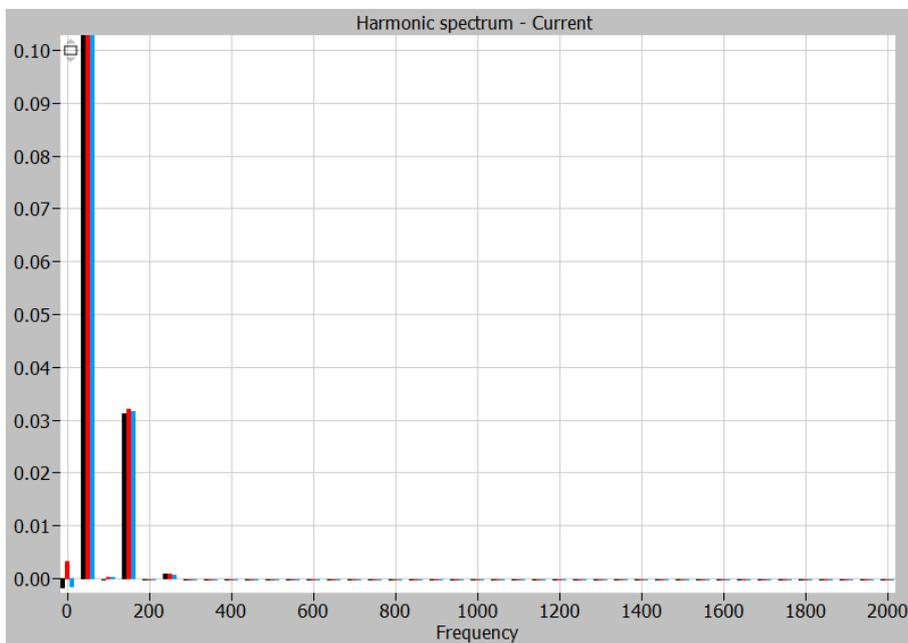
Figure 101: Harmonic spectrum of 10% decrease of voltage magnitude. Normalized to the fundamental frequency of 50 Hz, with magnitude '1'
