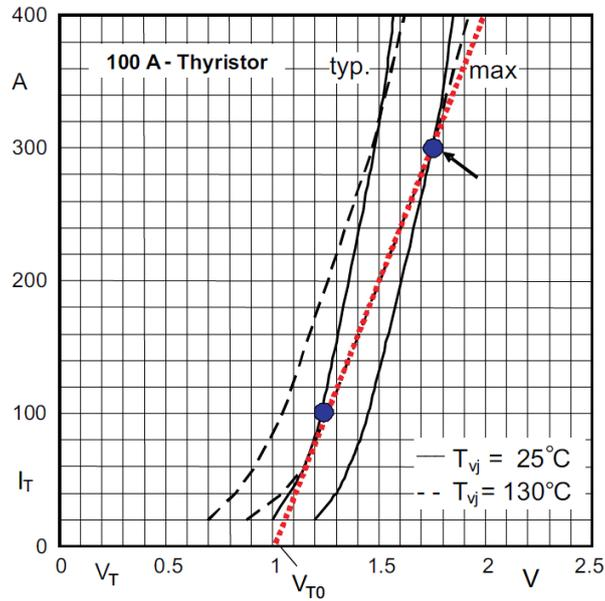
Figure 23: Example of  $V_{T(T0)}$  and straight line between  $1 * I_{T(Av)}$  and  $3 * I_{T(Av)}$  [35].
