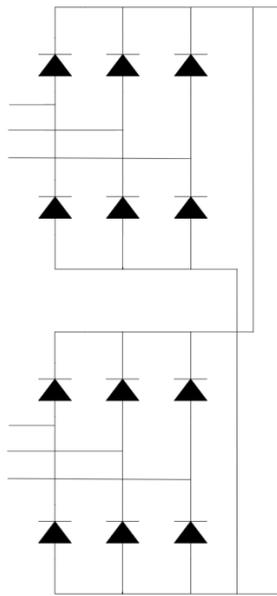
Figure 7: Rectifier stage, AC is converted to DC
