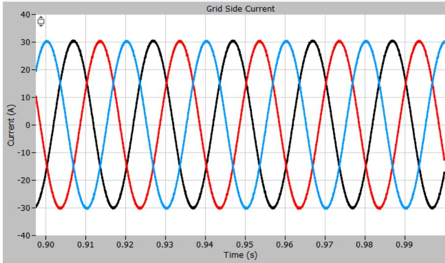
Figure 82: Grid Side Current and Grid side Current of 12-TRASPF with harmonic compensation and  $i_q^* = 0$
