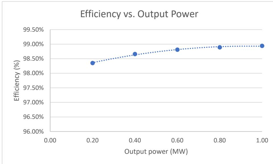
Figure 54: Efficiency vs power
