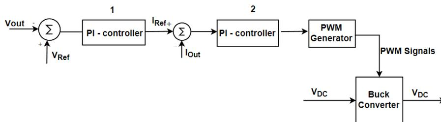
Figure 8: Control Diagram for Buck Converter
