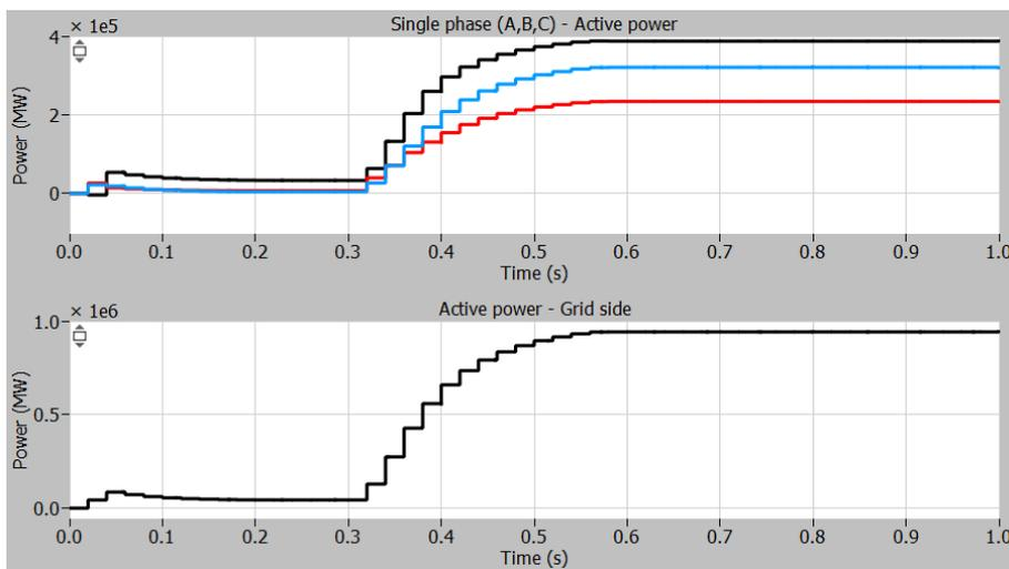
Figure 46: Active Power of Single Phases A, B & C & Total Grid Side Active Power with passive trap filter.
