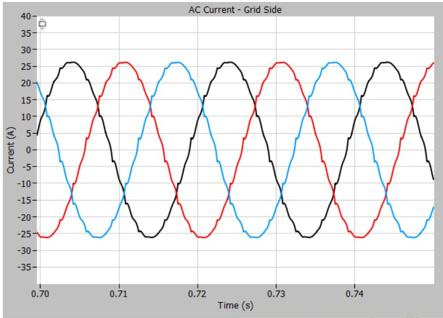
Figure 61: Current measurement on the grid side for 12-DRMC with Filter
