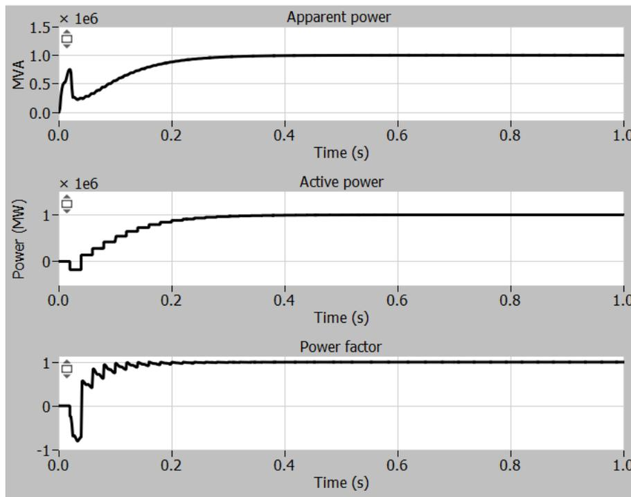
*Figure 98: Graphs of Apparent power (S), Active power (P) and Power factor (PF).*
