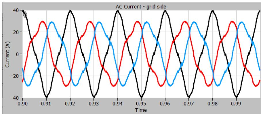
Figure 86: Grid Side Current of 12-TRASPF with 10% grid voltage magnitude decrease in phase B
