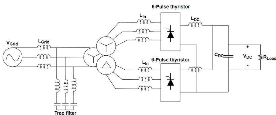
Figure 4: 12-TR model as a single line diagram.
