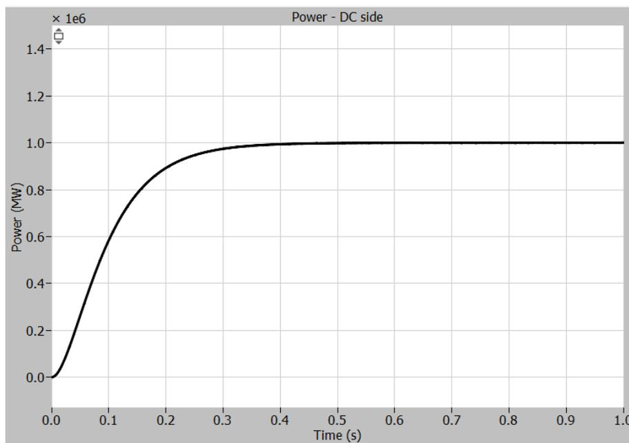
Figure 95: Power at the DC side from AFE
