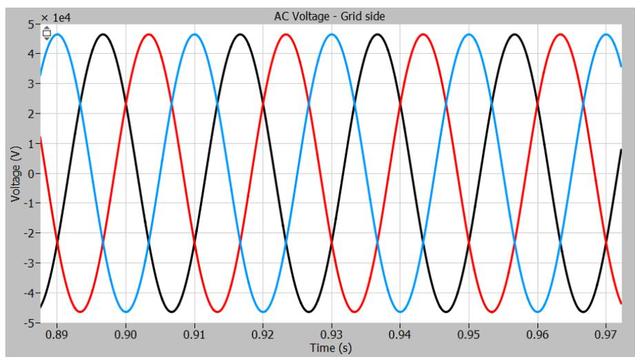
Figure 34: Measurement of voltage on the grid side with passive trap filter
