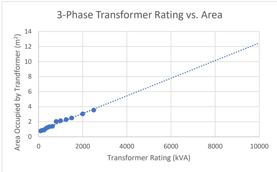
Figure 22: 3-phase Transformer Rating vs. Area Occupied
