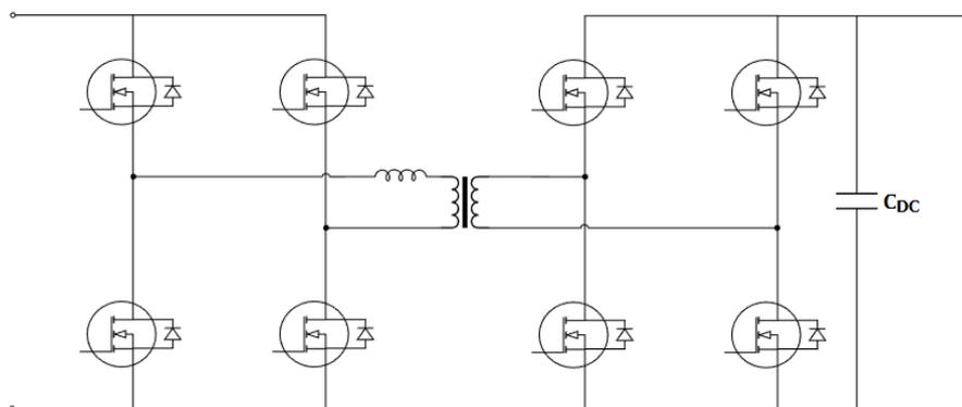
Figure 111: Dual Active Bridge configuration (DC/DC Stage)
