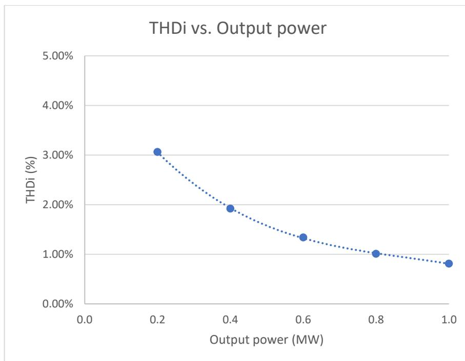
Figure 104: Load variation vs THD for the topology AFE
