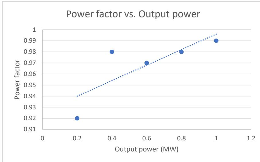
Figure 51: Load Variation vs Power Factor for 12-TR, with passive trap filter
