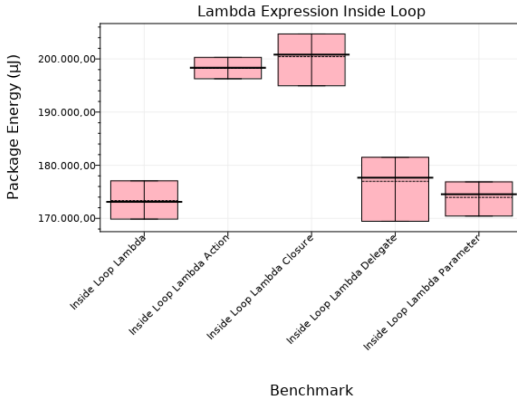
Figure 3.2: Energy Consumption for Lambda Expressions that are initialized inside the for loop
