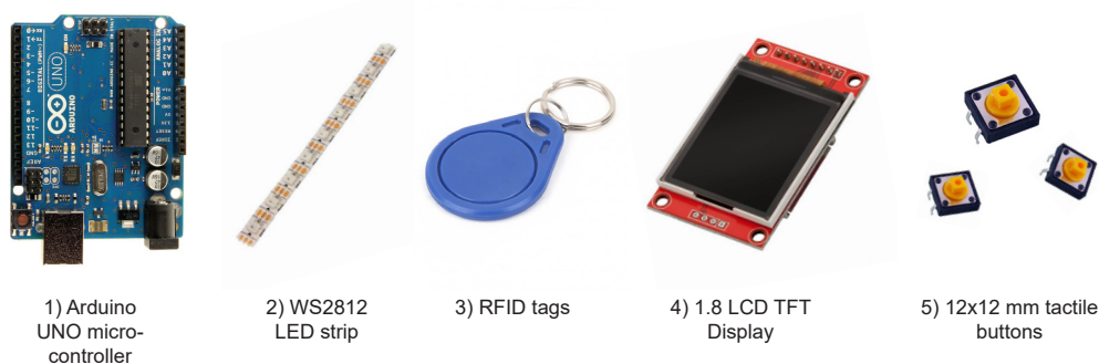
Figure 8.5: The five different technical components used for the Game Hub.
