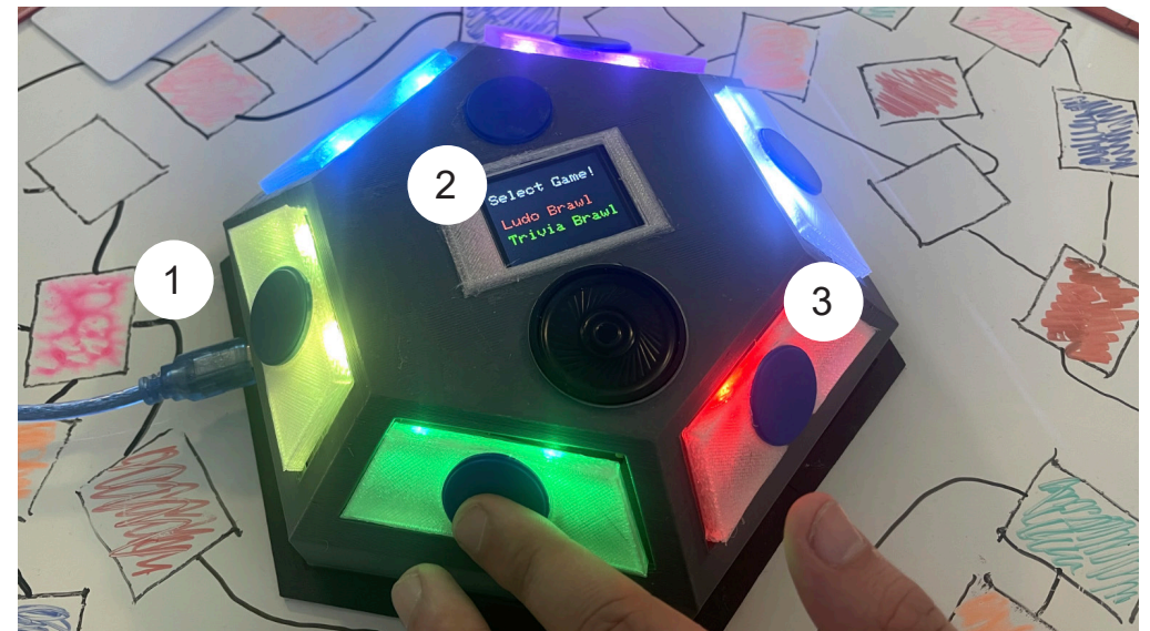
Figure 8.4: The Game Hub placed on the Trivia Board, where the screen displays the initial stage of HYBRIDA.
