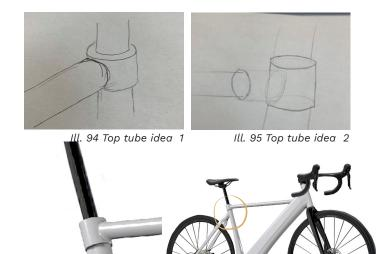
*Ill. 96 Top tube first solution* The first solution was reviewed. By adding other insertion point at the top of the seat tube and top of the down tube the top tube could be attached to the frame by the same method as a
