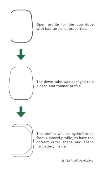
ved, and it was necessary to make FEM analysis of the new geometry, to see how it influenced the strengths and stiffness of the frame.
