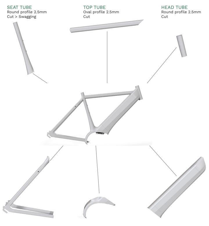
CHAIN & SEAT STAY Round profile 2.5mm Cut > Bend > Press > Weld CRANK BASE Sheet metal 5mm Stamping DOWN RUBE Round profile 2.5mm Cut > Hydroforming
