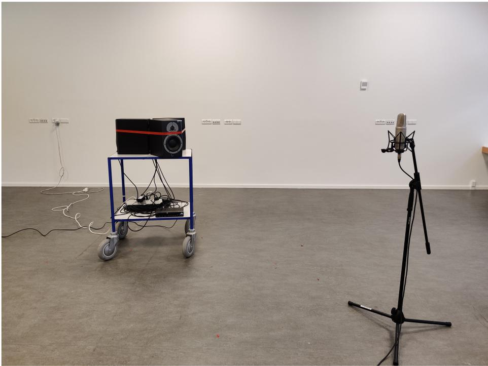
Figure 5.4: IR measurement setup.
