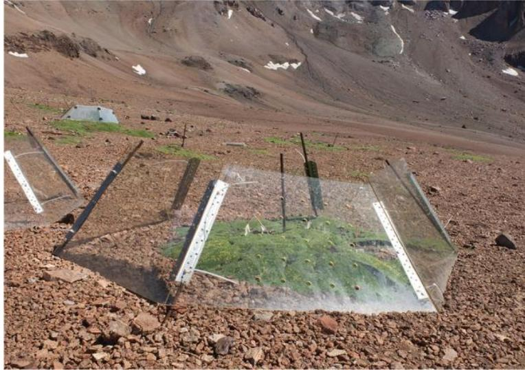
*Figure 4: Photograph of an Open Top Chamber taken in central Chile (Anthelme 2014).*
