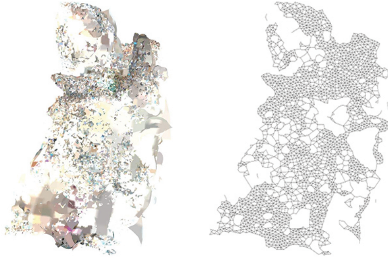
Figure 2.1: An example of a Growing Neural Gas algorithm performing. The parameters for GNG are: \text{max\_Nodes} = 2400 , \text{n\_iter\_before\_neuron\_added} = 100 , \text{after\_split\_error\_decay\_rate} = 0.5 , \text{error\_decay\_rate} = 0.995 , \text{min\_distance\_for\_update} = 0.01 , \text{step} = 0.2 , \text{n\_start\_nodes} = 2 , \text{max\_edge\_age} = 50 , and \text{neighbour\_step} = 0.005
