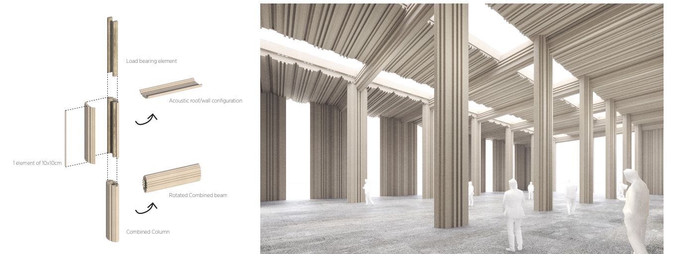
Fig 59: A building system based on reused wooden planks used as acoustic cladding.
