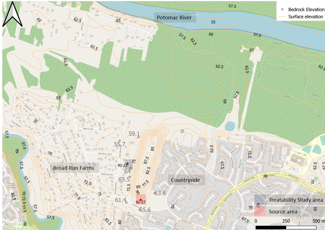
Figure 2.9: Topography and bedrock elevation for the HLLSS. Data from [EPA, 2015b] and [QGIS].
