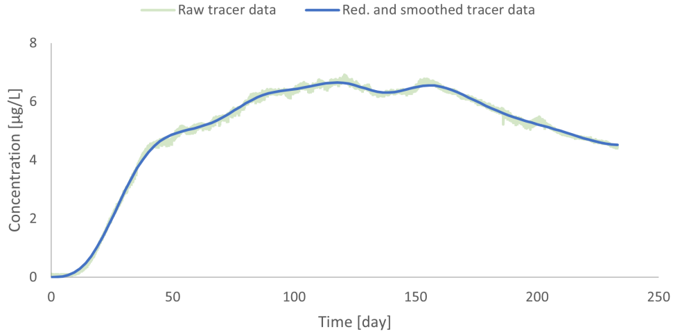
Figure 6.4: Raw and the reduced and smoothed tracer data, for well RI-21S (L2).
