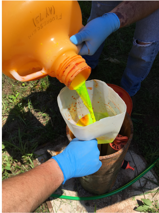
Figure 3.1: Injection of the diluted tracer [Field, 2020].
