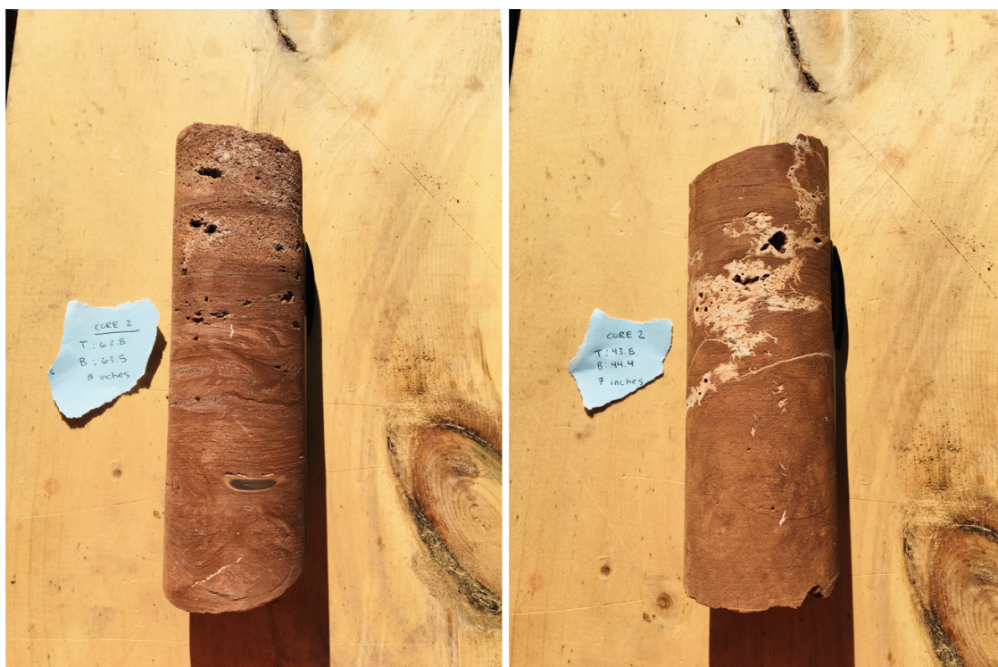
Figure 2.10: Bedrock samples from the HLLSS illustrating the fractures [Field, 2020].
