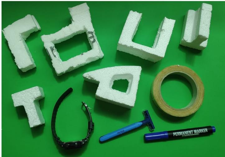
**Figure 4.10:** Pick-and-place test objects consisted of 6 custom shapes and 4 everyday use objects.
