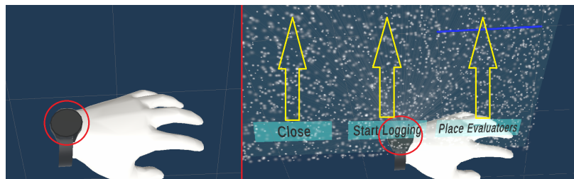
Figure 6.3: Overlapping position of the "start logging" button and the activation of the GUI. The yellow arrows indicate that these buttons should be moved upwards to avoid overlapping and accidental presses.
