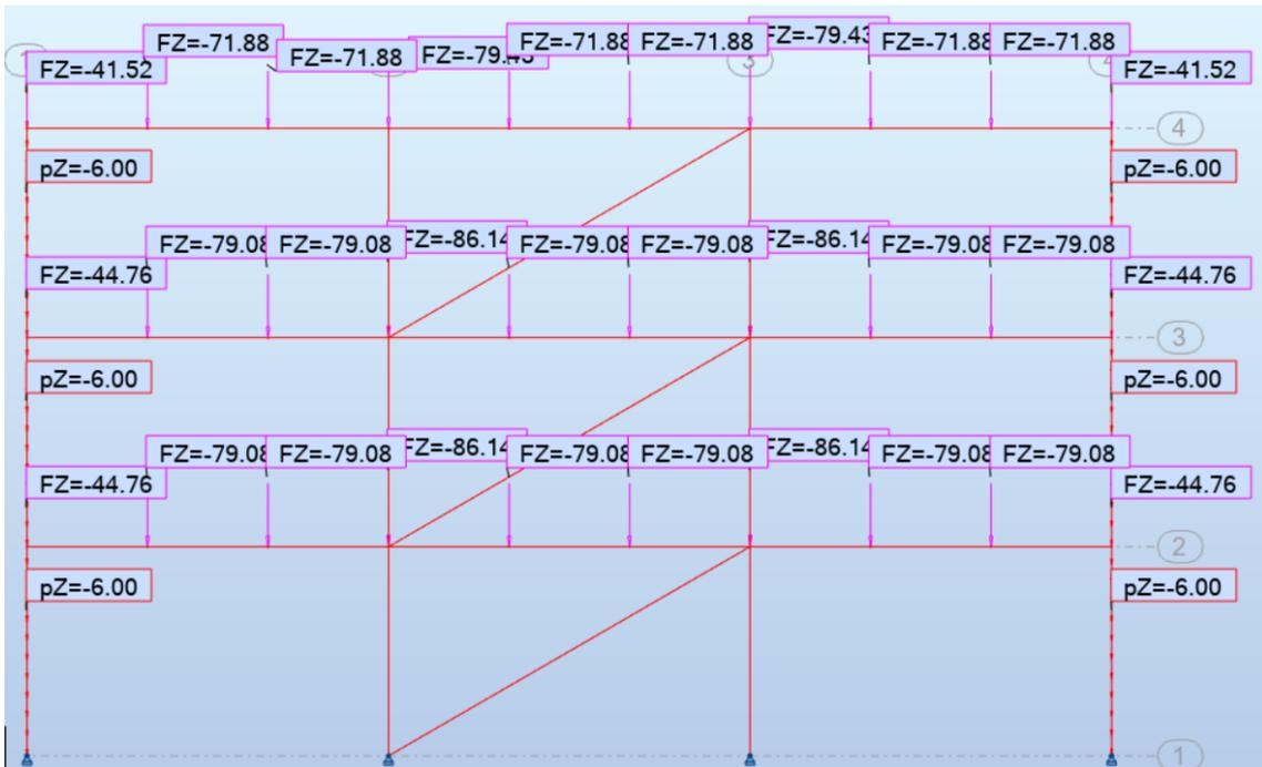
Figure C.4: Vertical (gravity) loads applied on the 2D CBF model in SeismoStruct [2022]. NOTE: self-weight of elements is automatic and not included here!
