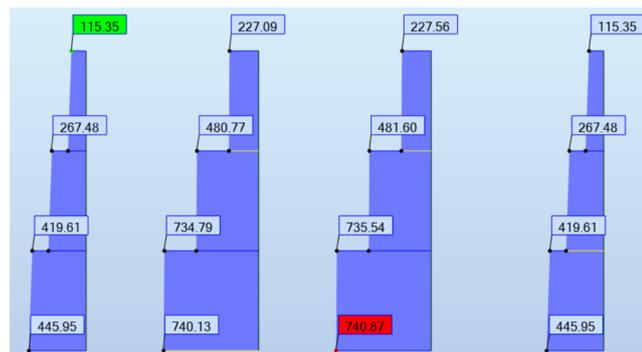
**Figure 8.16:** Axial force diagrams in columns from seismic mass load combination [Autodesk Robot, 2021]
