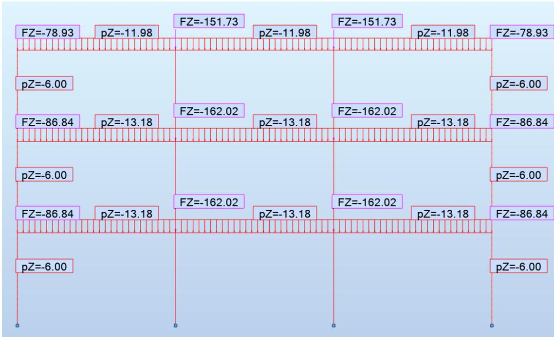
Figure C.3: Vertical (gravity) loads applied on the 2D MRF model in SeismoStruct [2022]. NOTE: self-weight of elements is automatic and not included here!
