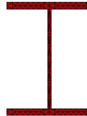
Figure 8.6: Discretization of HE profile section - 150 fibers [SeismoStruct, 2022]
