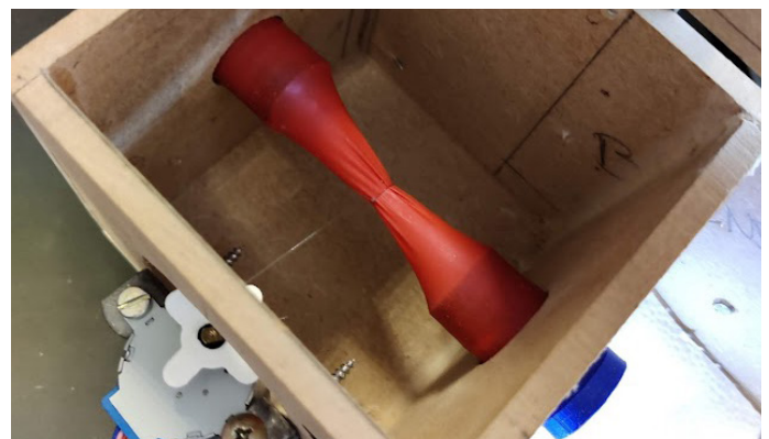
Figure 05: The balloon with thread around connected to the motor.
