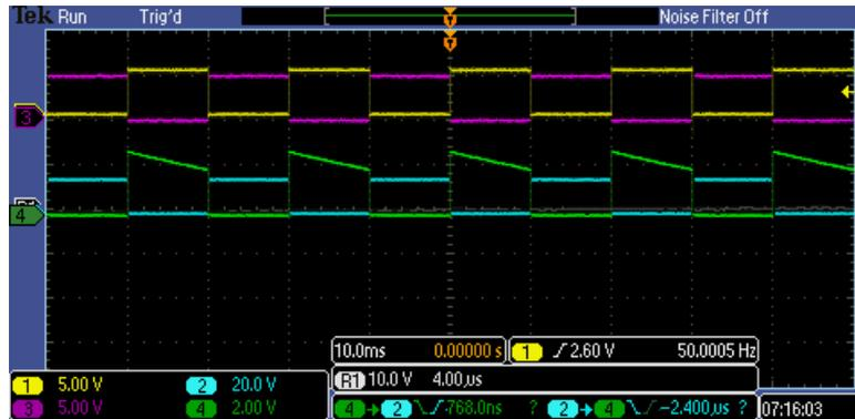
**Figure 5.11.** Gate driver test result on slow switching leg. channel 1 represents the input PWM signal for the up leg MOSFET. channel 2 represents the input PWM signal for the down leg MOSFET. channel 3 represents the output gate driving signal for the up leg MOSFET. channel 4 represents the output gate driving signal for the down leg MOSFET (with  $\frac{1}{5}$ ) scaling ratio caused by the isolation probe.
