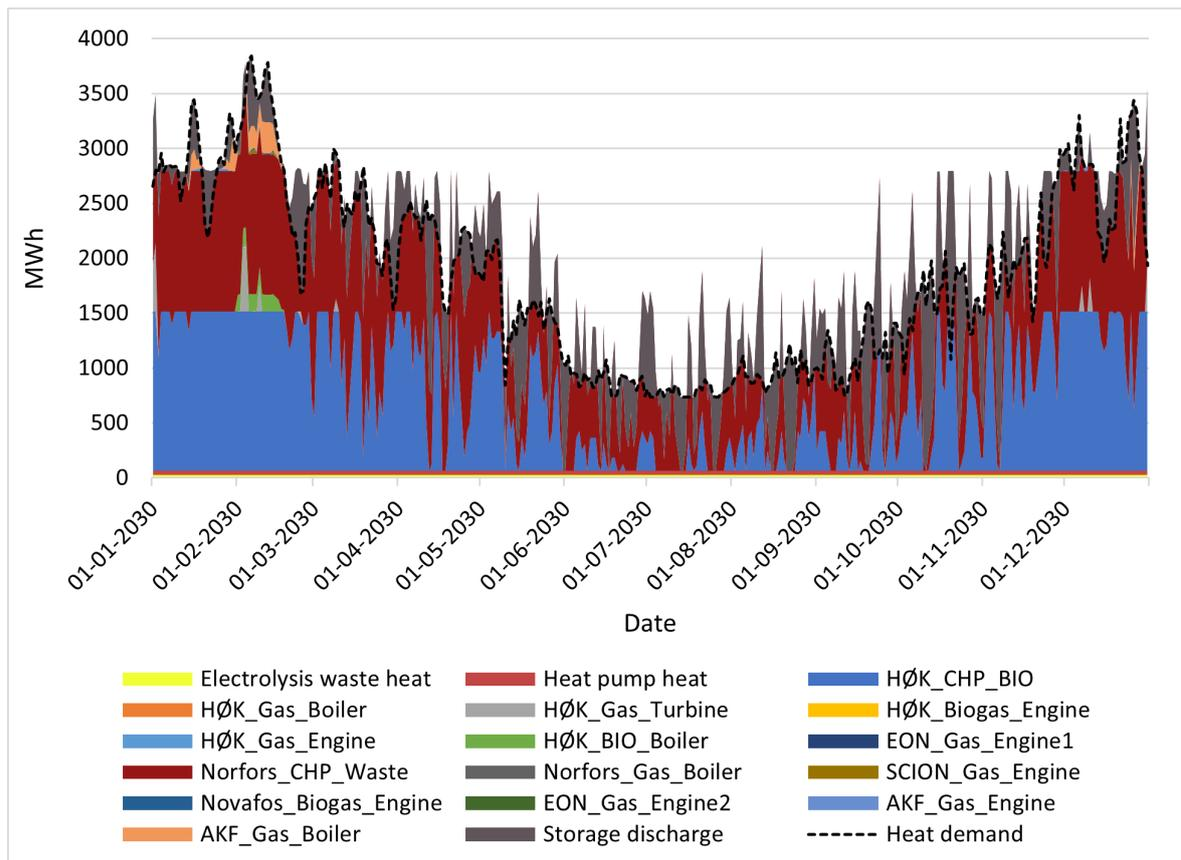
**Figure 9.15.** Heat producing units, heat demand, and storage discharge in the NØS DH system with integration of waste heat from PtX.
