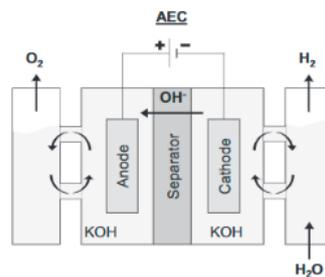
**Figure 3.1.** Operating principle of AEC [DEA, 2021e, p. 94].
