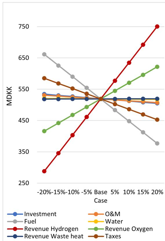
**Figure 9.25.** Sensitivity of the NPV calculation of the NØS electrolyser, plotted in increments of 5% and displayed in MDKK.
