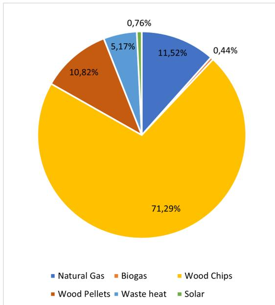
**Figure 9.10.** Heat produced from fuel in the HFV DH system.
