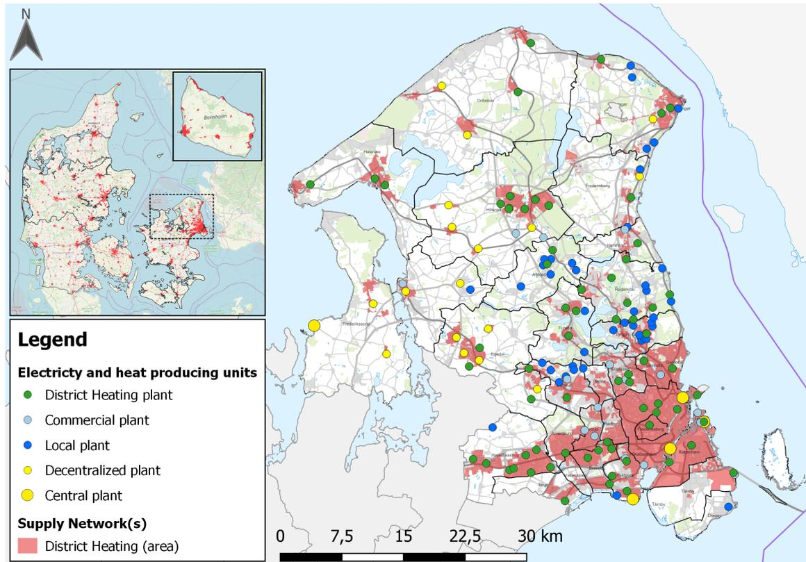
**Figure 2.2.** DH network(s) and electricity and heat producing units in the Capital Region of Denmark [Erhvervsstyrelsen, 2021; Open Data DK, N/A]
