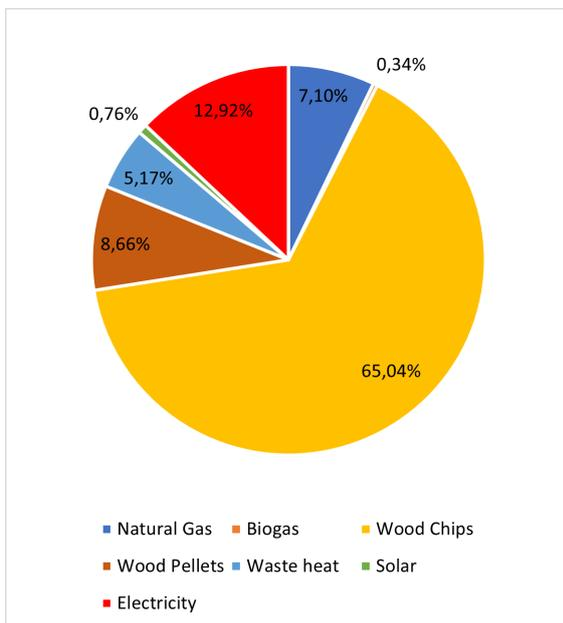
**Figure 9.16.** Heat produced from fuel with integration of waste heat from PtX in the HFV DH system.
