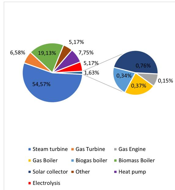
**Figure 9.11.** Heat produced based on technology in the HFV DH system.
