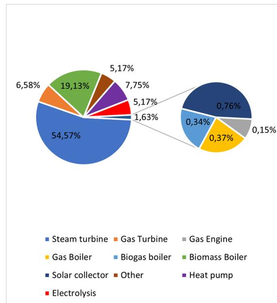
**Figure 9.17.** Heat produced from technology with integration of waste heat from PtX in the HFV DH system.
