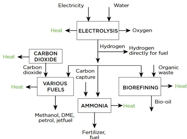
*Figure 2.1.* A variety of value-chains for different PtX technologies [DDHA, 2021, p. 8].
