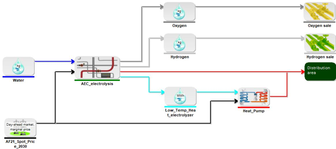
**Figure 8.12.** Setup of the electrolysis plants including heat pump for upgrading low temperature heat.
