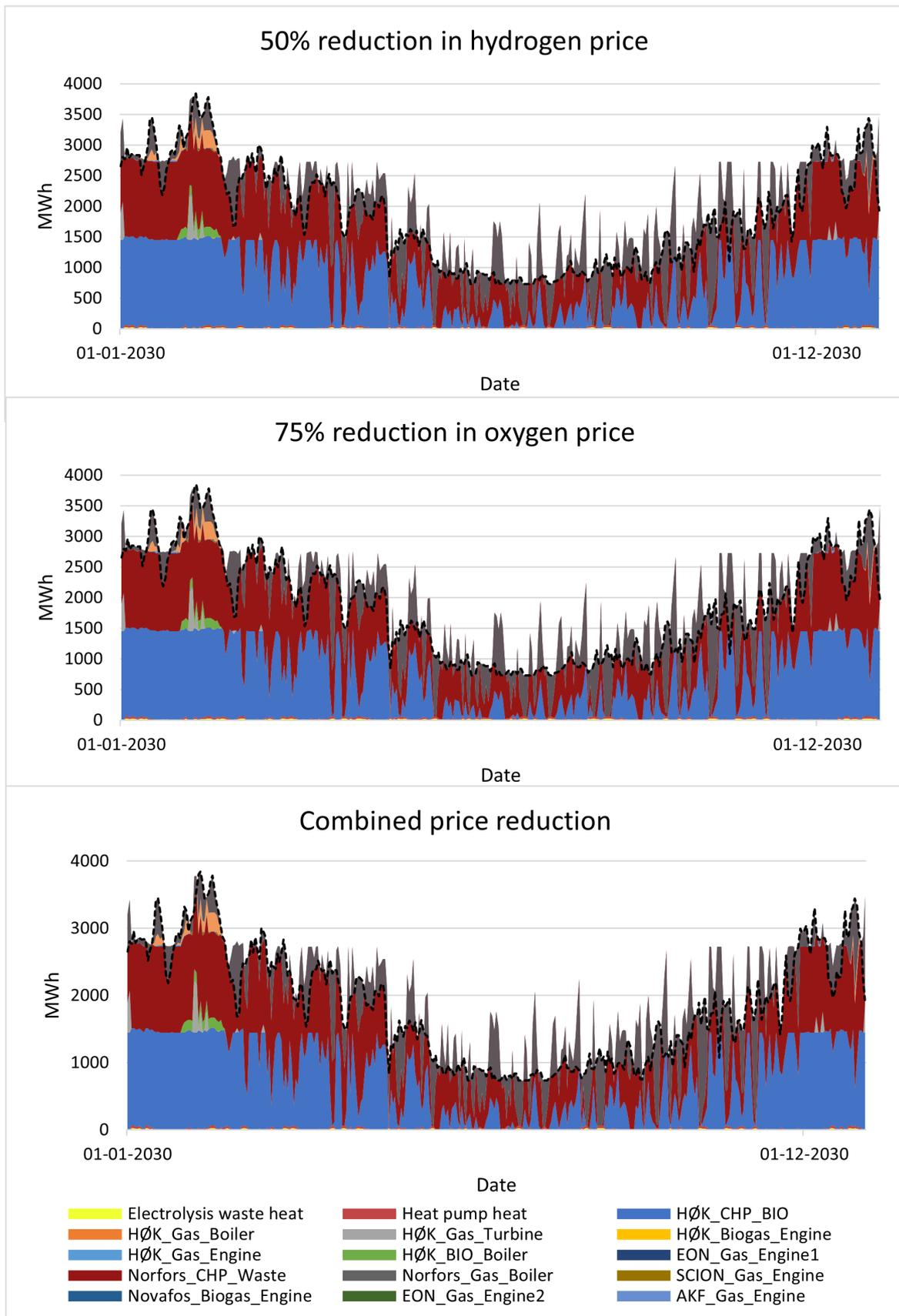
Figure 9.19. Showing the effects on three different sensitivity scenarios on the operation of the NØS system, per day.
