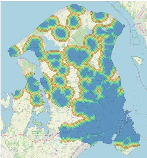
**Figure 8.1.** DH grid in the Capital Region of Denmark with five increments of 500 meters. Data is from [Erhvervsstyrelsen, 2021].
