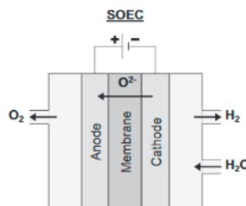
**Figure 3.3.** Operating principle of SOEC [DEA, 2021e, p. 94].
