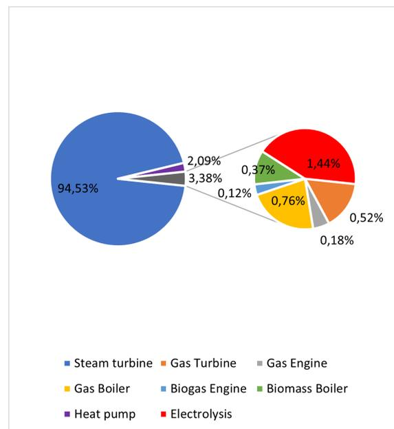
**Figure 9.14.** Heat produced from technology with integration of waste heat from PtX in the NØS DH system.
