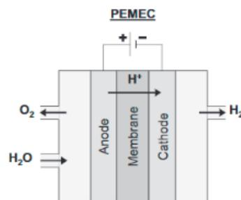
**Figure 3.2.** Operating principle of PEMEC [DEA, 2021e, p. 94].
