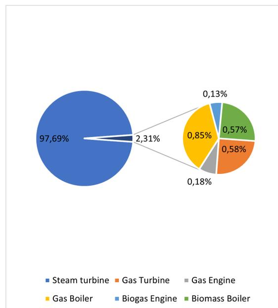
**Figure 9.8.** Heat produced based on technology in the NØS DH system.
