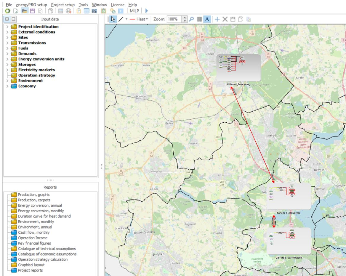
**Figure 8.11.** Screenshot of the energyPRO interface including modelled sites in the reference model for the HFV DH network forecasted to 2030. Liberties are taken to include a background map to illustrate the general location of the modelled sites.
