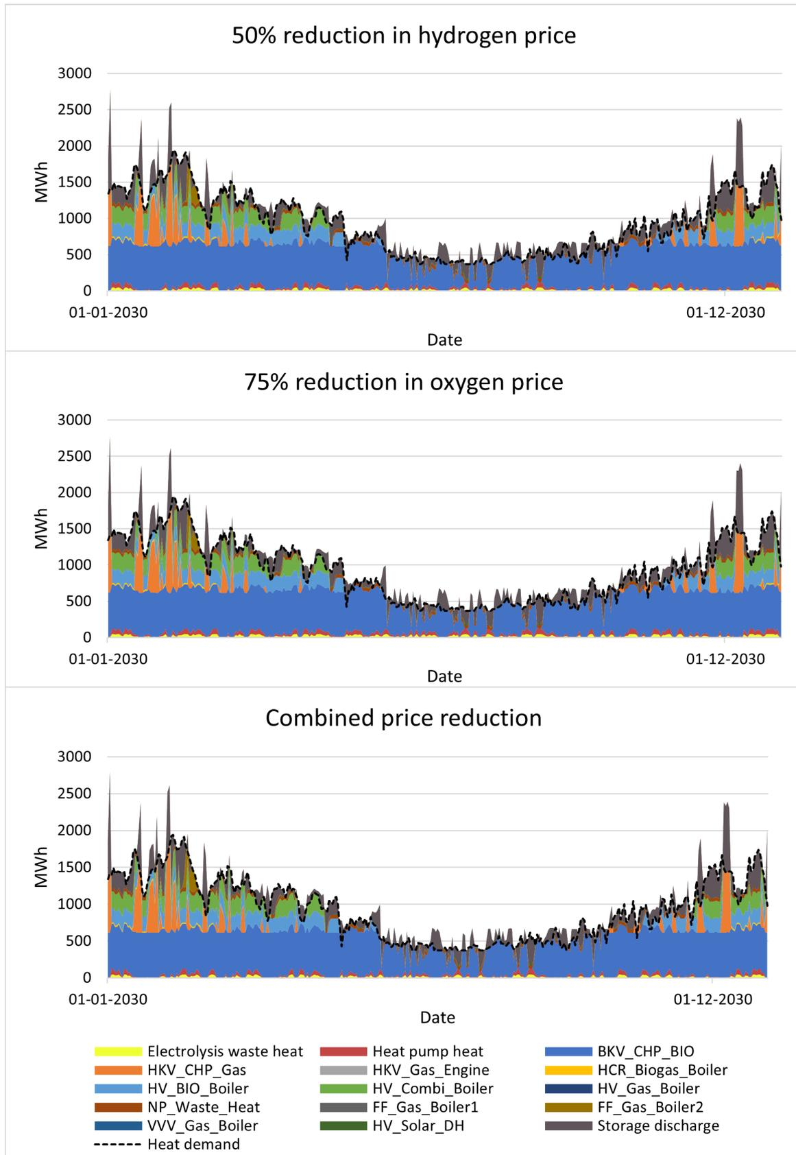
Figure 9.20. Showing the effects on three different sensitivity scenarios on the operation of the HFV system, per day.
