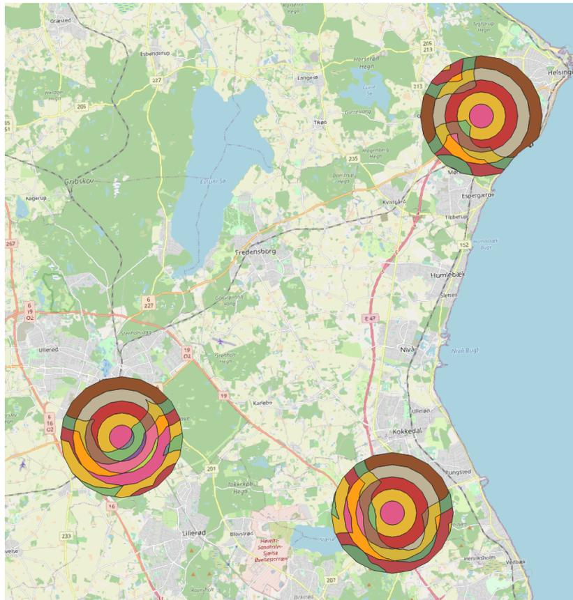
**Figure 8.3.** Zoomed in area of CO<sub>2</sub> point sources according to [EEA, 2021] in the Capital Region of Denmark with five increments of 500 meters, showing overlay with DH ring buffers.
