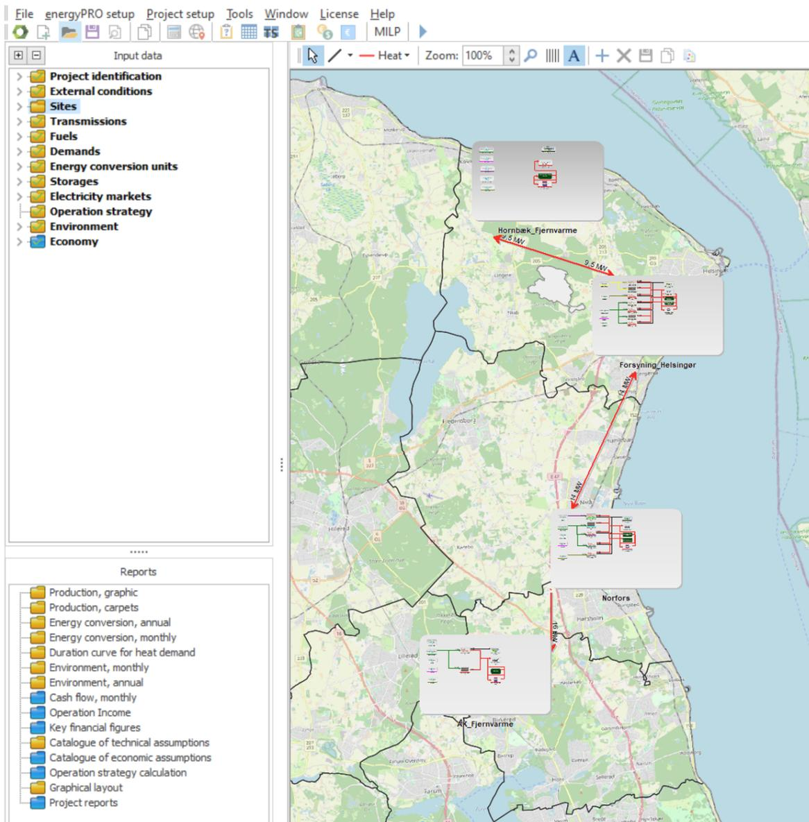
**Figure 8.10.** Screenshot of the energyPRO interface including modelled sites in the reference model for the NØS DH system forecasted to 2030. Liberties are taken to include a background map to illustrate the general location of the modelled sites.
