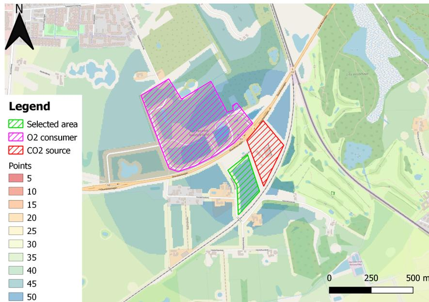
**Figure 9.6.** Suitable locations for placement of PtX-facility in Hillerød. 'Selected area' (green hatched area) is the chosen location for placement of PtX-facility (for further analysis) and the purple hatched area is a potential O<sub>2</sub> consumer and the red hatched area is a CO<sub>2</sub> source.
