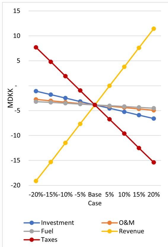
**Figure 9.27.** Sensitivity of the NPV calculation of the NØS heat pump, plotted in increments of 5% and displayed in MDKK.
