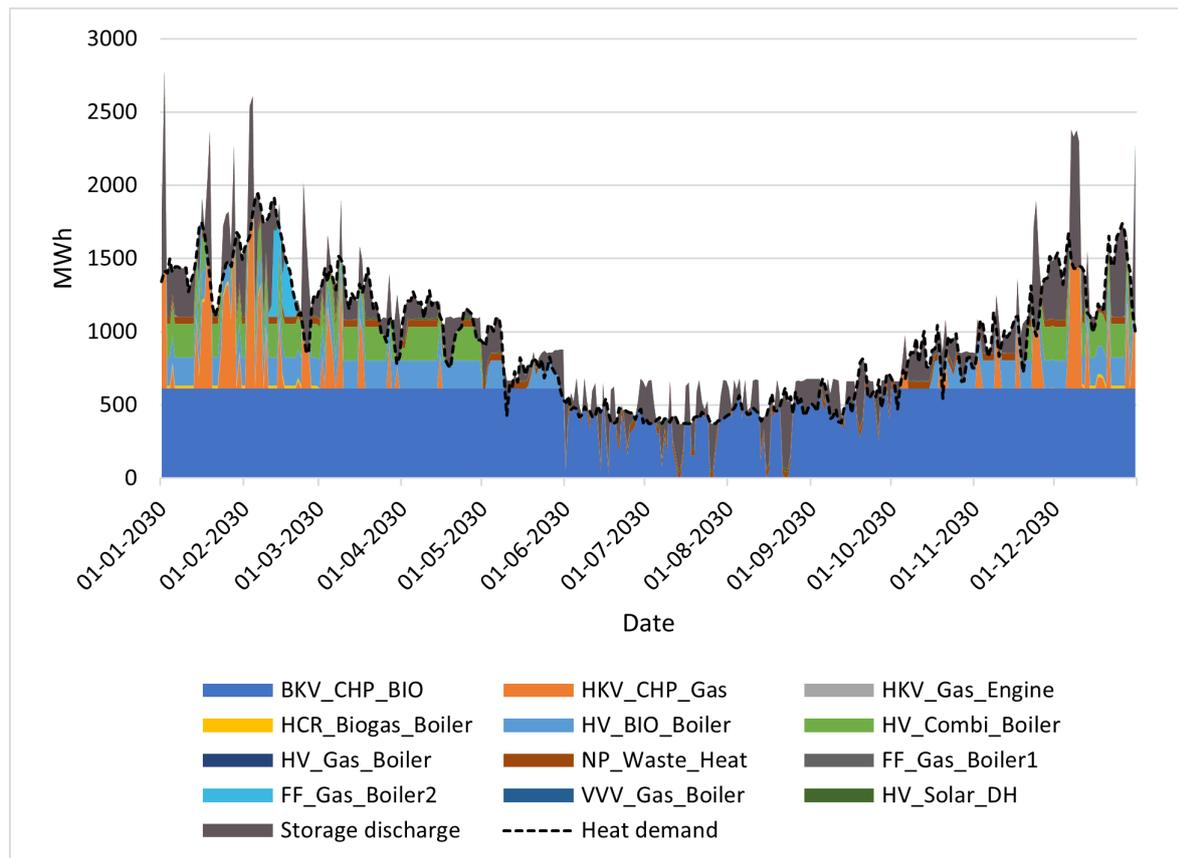
**Figure 9.12.** Heat producing units, heat demand, and storage discharge in the HFV DH system.
