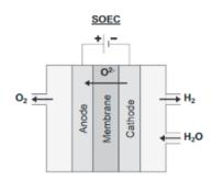
Figure 3.3. Operating principle of SOEC [DEA, 2021e, p. 94].
