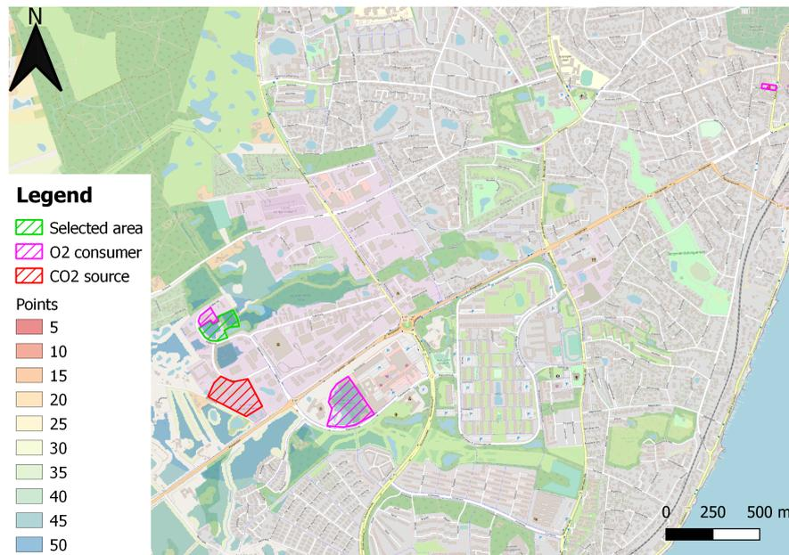
**Figure 9.3.** Suitable locations for placement of PtX-facility in Helsingør. 'Selected area' (green hatched area) is the chosen location for placement of PtX-facility (for further analysis) and the purple hatched areas is a potential O<sub>2</sub> consumer and the red hatched area is a CO<sub>2</sub> source.
