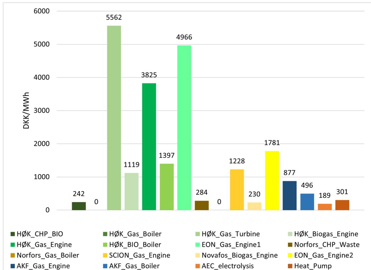
**Figure 9.21.** Heat sale price of the heat producing units in the NØS DH system with integration of PtX. The green columns represent the heat producing units in Forsyning Helsingør A/S. The yellow columns represent the heat producing units in I/S Norfors. The blue columns represent the heat producing units in AK Fjernvarme. The orange columns represent the heat producing units in the PtX site.
