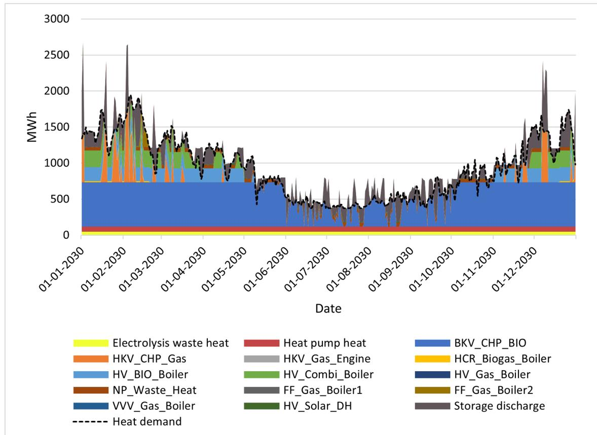
**Figure 9.18.** Heat producing units, heat demand, and storage discharge in the HFV DH system with integration of waste heat from PtX.
