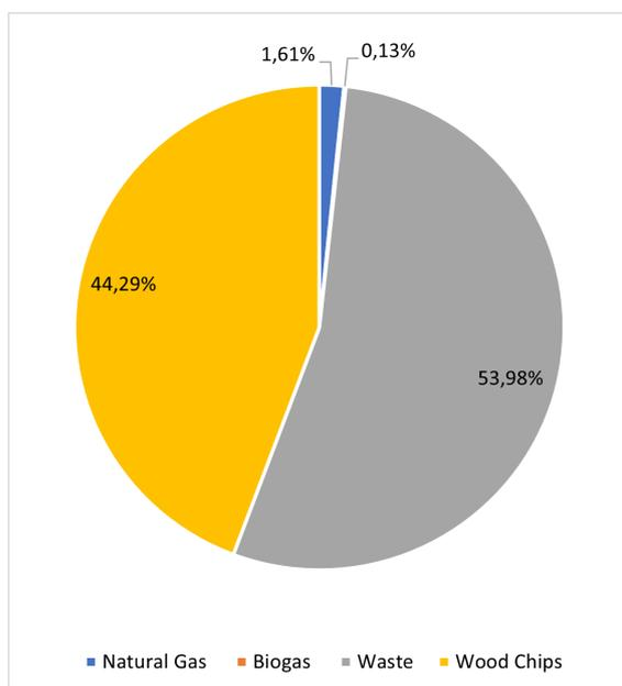
**Figure 9.7.** Heat produced from fuel in the NØS DH system.
