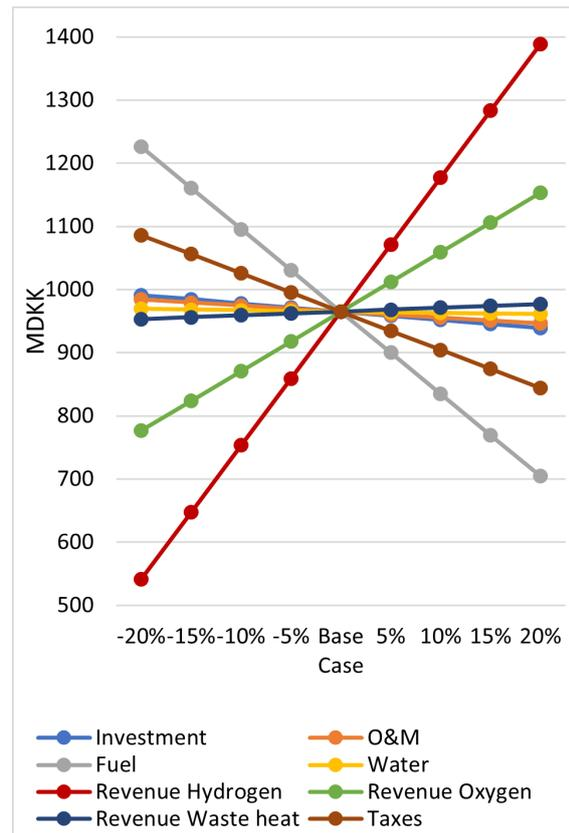
**Figure 9.26.** Sensitivity of the NPV calculation of the HFV electrolyser, plotted in increments of 5% and displayed in MDKK.
