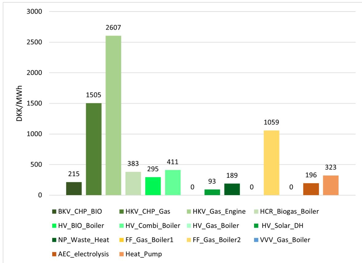
**Figure 9.23.** Heat sale price of the heat producing units in the HFV DH system with integration of PtX. The green columns represent the heat producing units in Hillerød Forsyning A/S. The yellow columns represent the heat producing units in Farum Fjernvarme A.m.b.a.. The blue columns represent the heat producing units in Værløse Varmeværk A.m.b.a. The orange columns represent the heat producing units in the PtX site.
