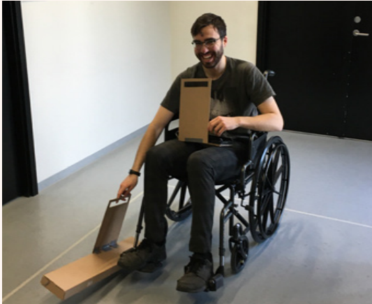
III. 2.39: Unfolding and placing the belt-driven concept on the floor (this must be done twice)
