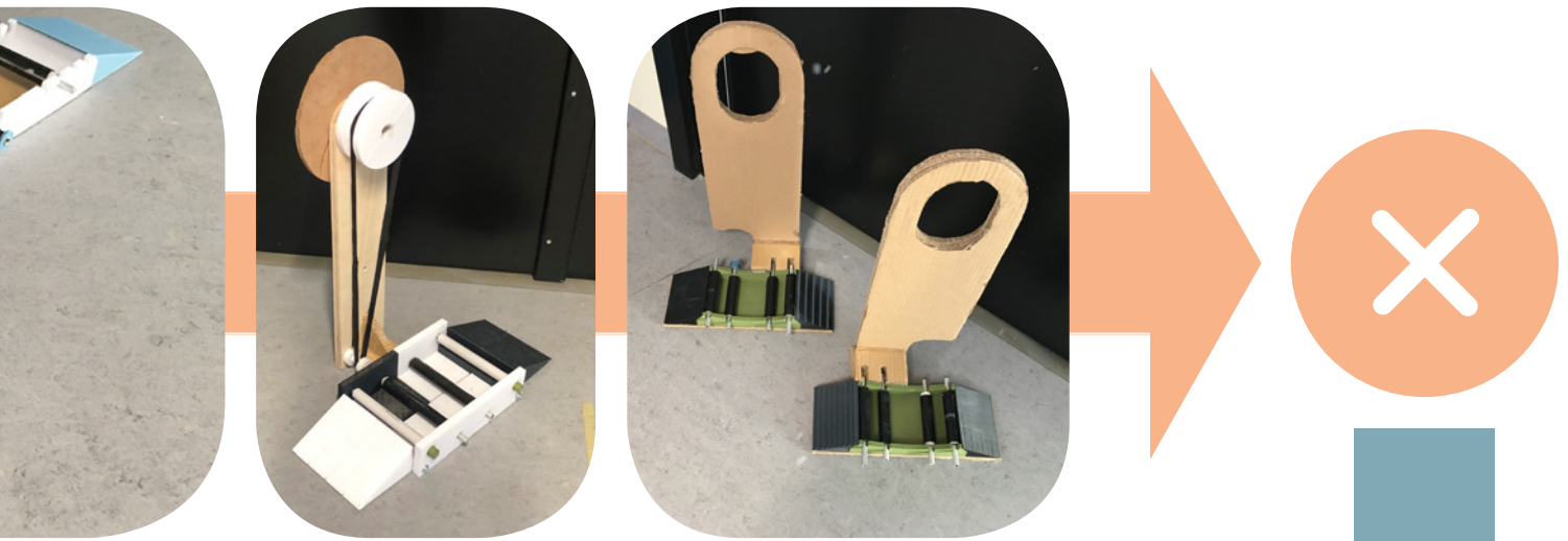
Ill. 5.3: Three transportable concept directions: belt-driven (left), push handle (middle) and motorised (right)
