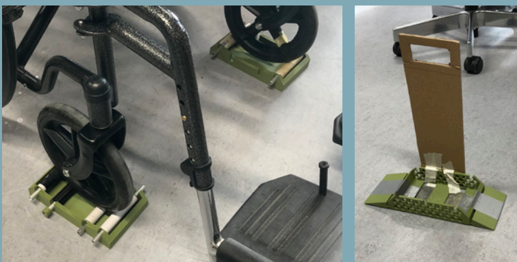
III. 2.45: Motorised concept prototypes – prototypes with rollers (left) and prototype with handle (right)
