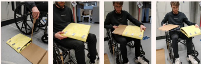
Ill. 3.27: Replacing cloth on triangle concept (4 steps)
