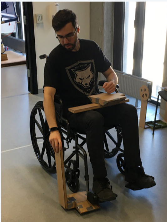
III. 2.43: Unfolding and placing the product on the floor (this must be done twice)
