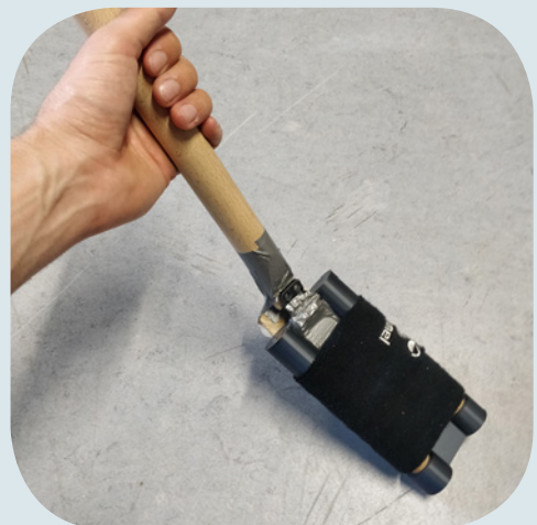
Ill. 4.25: Prototype of handheld device concept with two tubes and a sweatband
