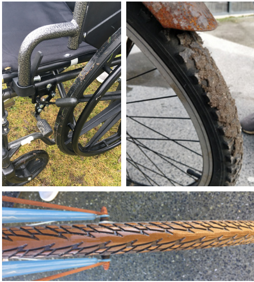
Ill. 2.20: Wheel types: flat wheelchair wheel (top left), mountain bike wheel (top right) and city bike wheel (bottom)
