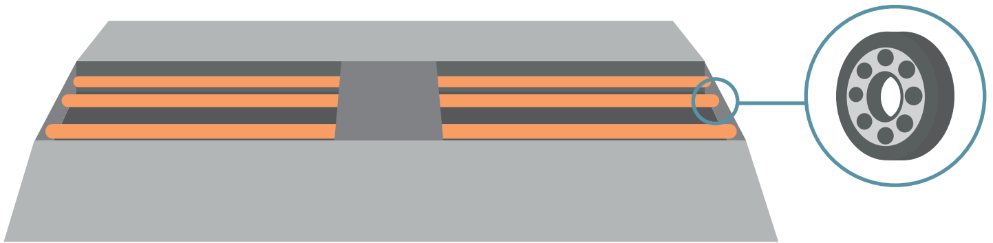
Ill. 4.7: Base with rollers (left) and ball bearing (right)
