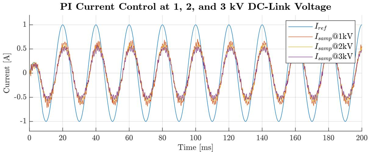
Figure 5.20: PI controller - Transient response of sampled load current at 1 A reference.
