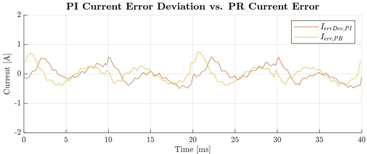
Figure 5.37: Comparison of PI and PR controller performance.
