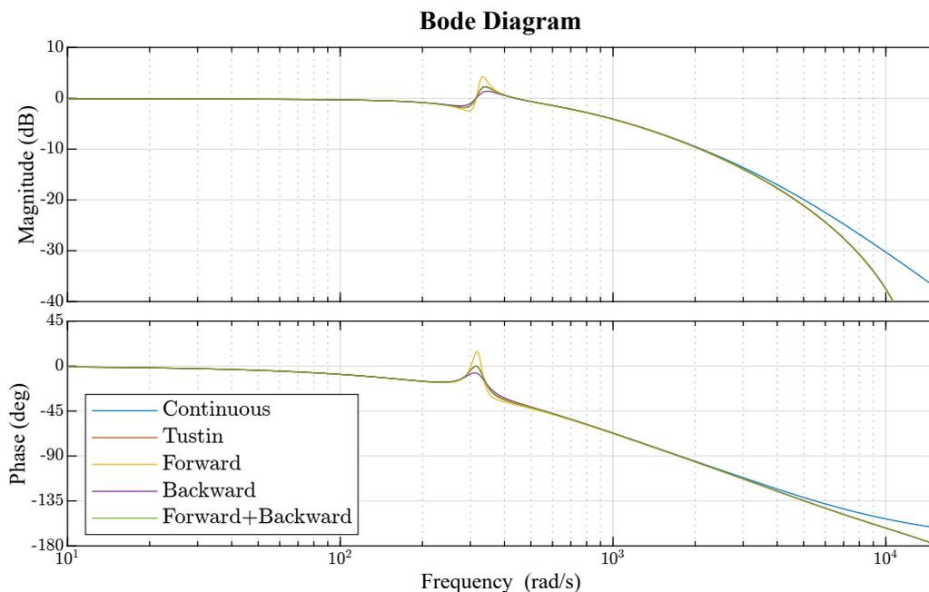
Figure A.5: Bode plot of PR controller. Comparison of discrete implementations.
