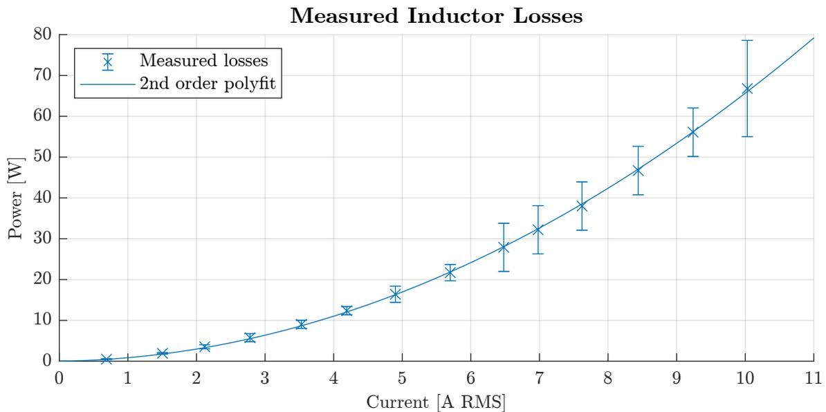
Figure 6.8: Measured power losses from inductor loss test.
