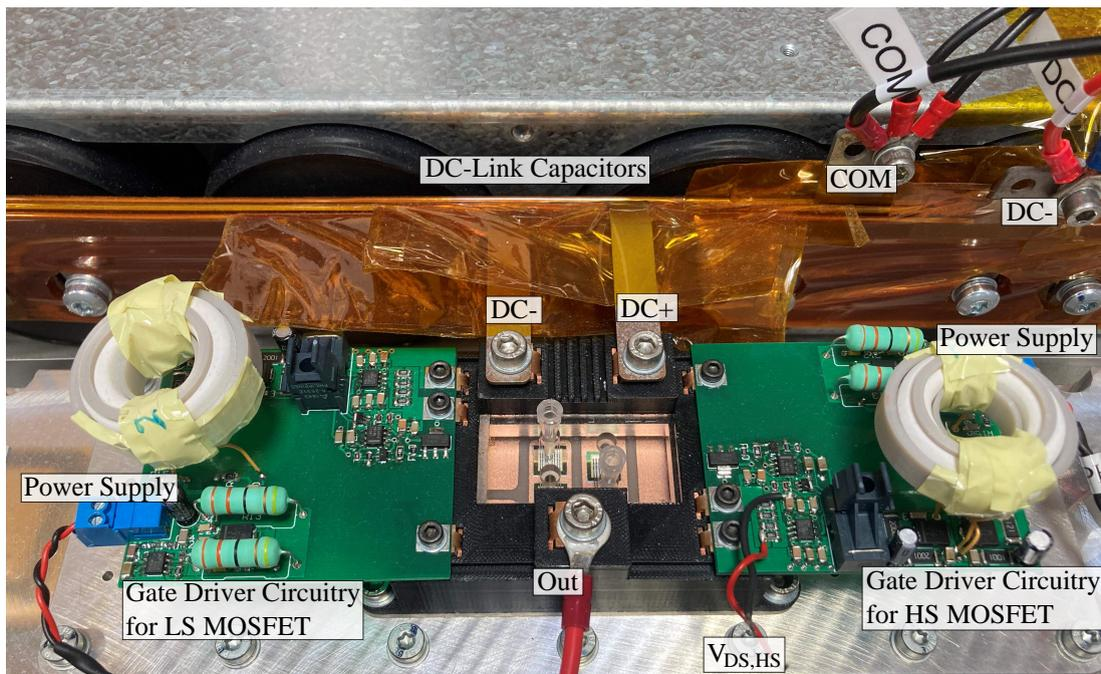
Figure 2.4: Photograph of one of the power modules and its gate drivers.
