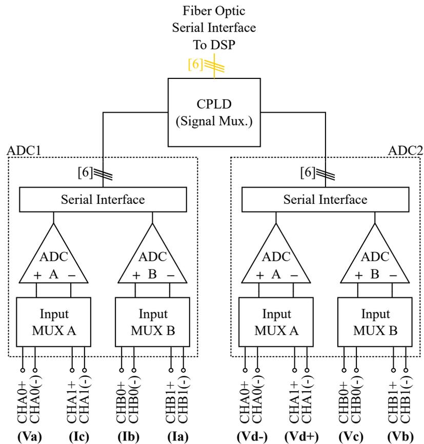
Figure 4.2: ADC configuration and interface on the PIF card.
