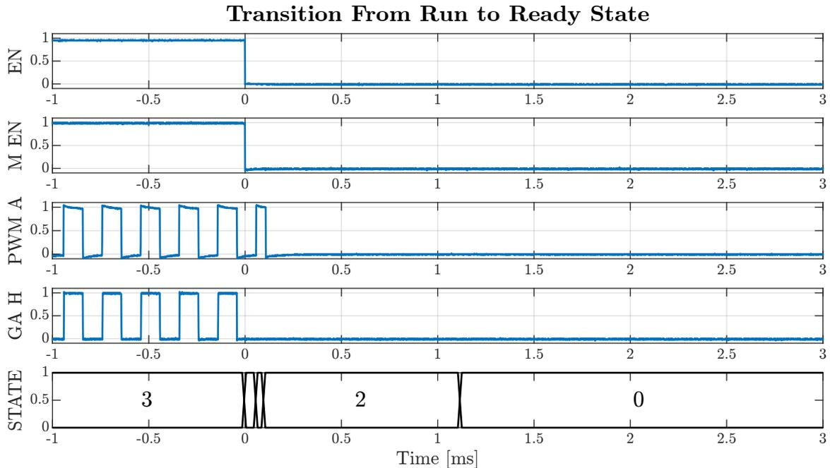
Figure 4.15: Measured transition from Run to Ready state on PIF card.
