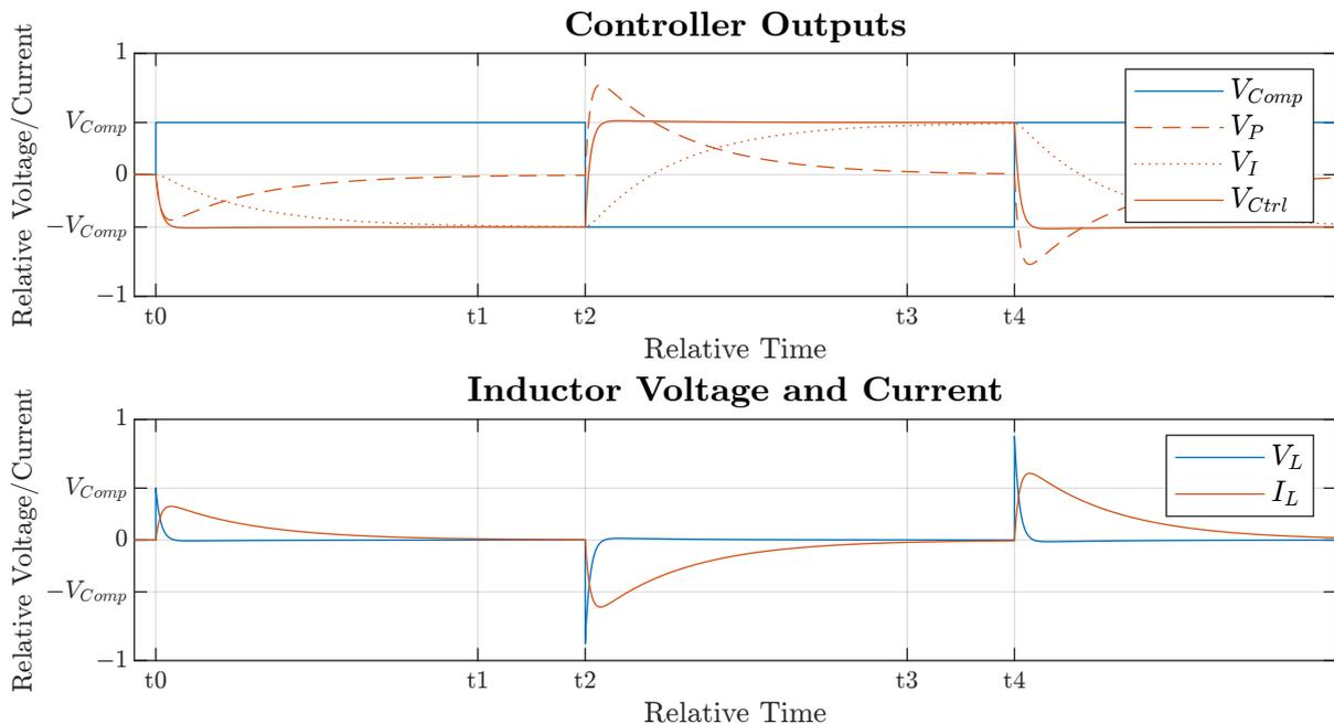
Figure 5.6: Simulation of instability issue caused by the initial dead time compensation algorithm.
