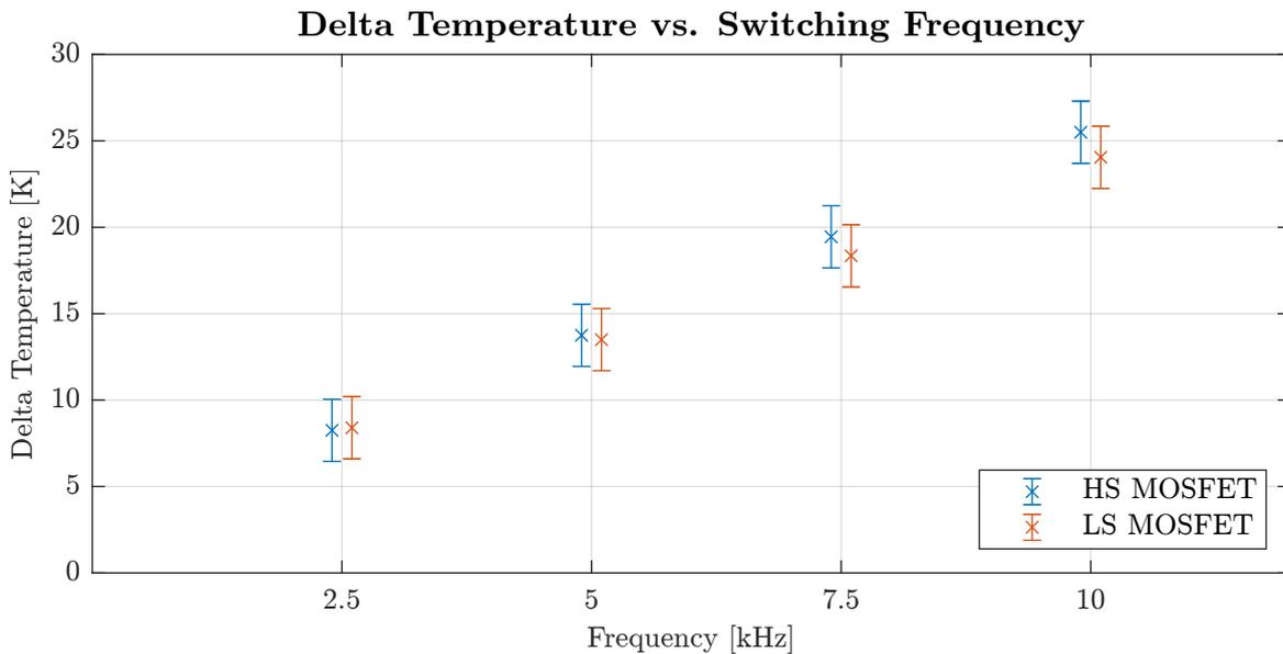
Figure 6.13: Delta die temperature at different switching frequencies.
