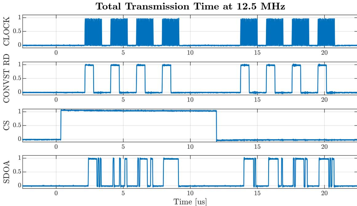
Figure 4.11: Measured total transmission time for all eight ADC channels at 12.5 MHz.
