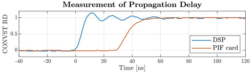
Figure 4.7: Measured propagation delay for CONVST RD from DSP to PIF card.
