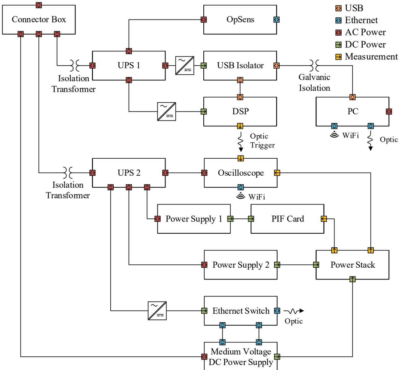
Figure 4.18: System configuration used for successful system operation at 6 kV DC-link voltage.
