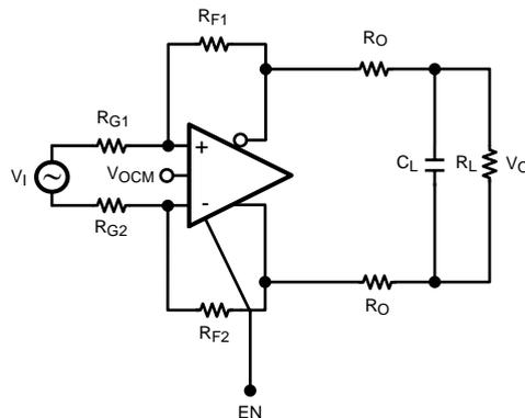
Figure B.3: Typical fully-differential coupling of the LMP8350 [55].
