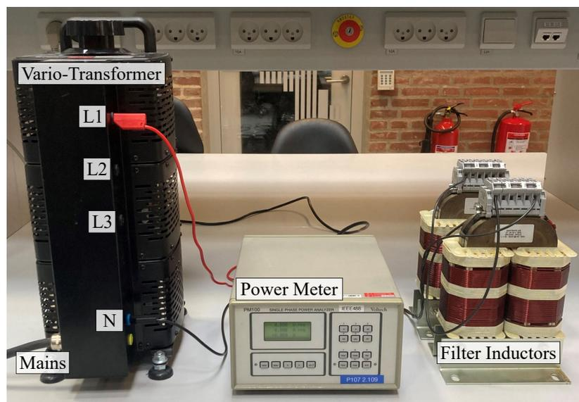
Figure 6.7: Photograph of the inductor loss test.
