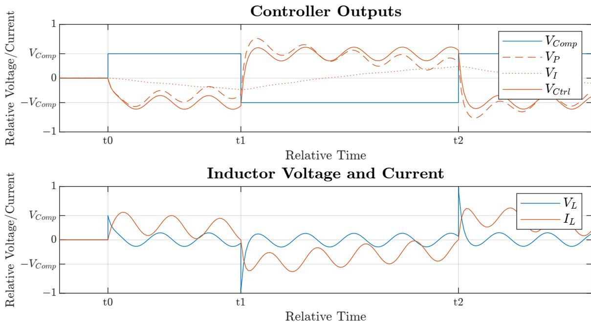
Figure 5.7: Simulation of instability issue caused by the initial dead time compensation algorithm.
