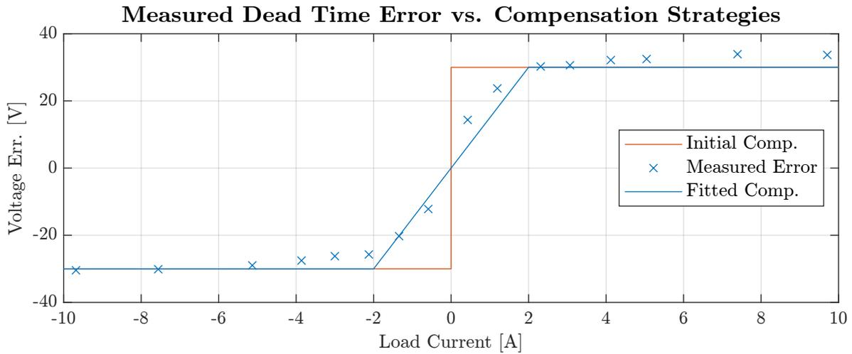
Figure 5.16: Measured dead time voltage error for varying load currents plotted along with the initial and fitted dead time compensation algorithm.
