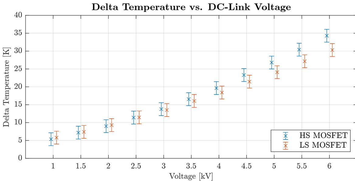
Figure 6.11: Delta die temperature at different DC-link voltages.
