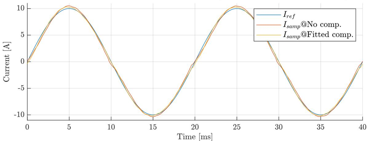
Figure 5.35: PR controller with compensation - Steady state response of sampled load current at 10 A reference.
