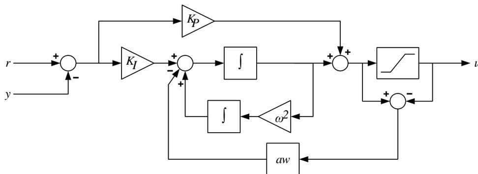
Figure 5.29: Structure of continuous PR current controller.
