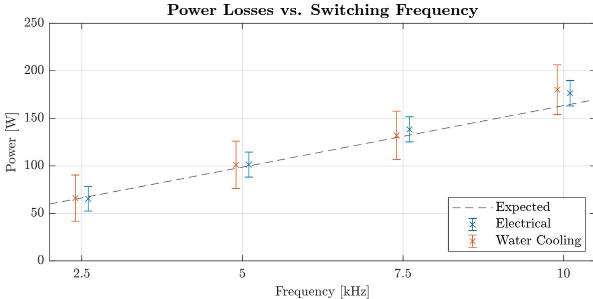
Figure 6.12: Power losses at different switching frequencies.
