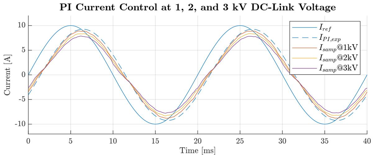
Figure 5.23: PI controller - Steady state response of sampled load current at 10 A reference.
