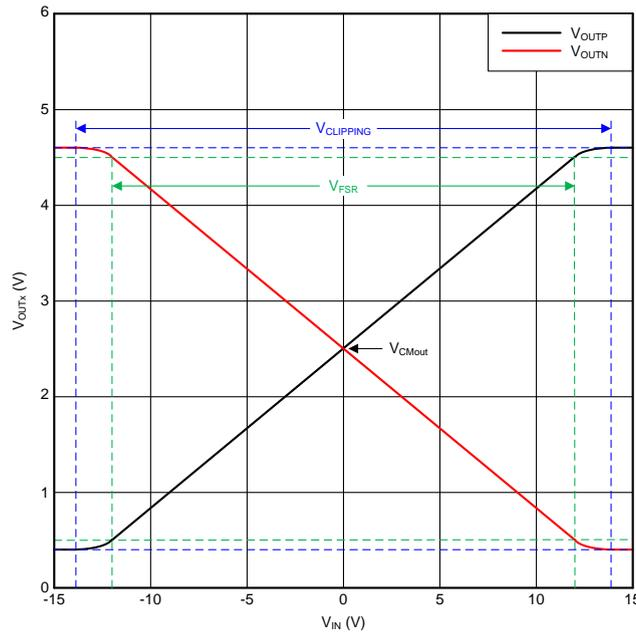
Figure B.2: Relation between input and output voltages for the ISO224 [54].
