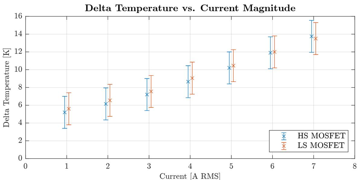
Figure 6.15: Delta die temperature at different current magnitudes.
