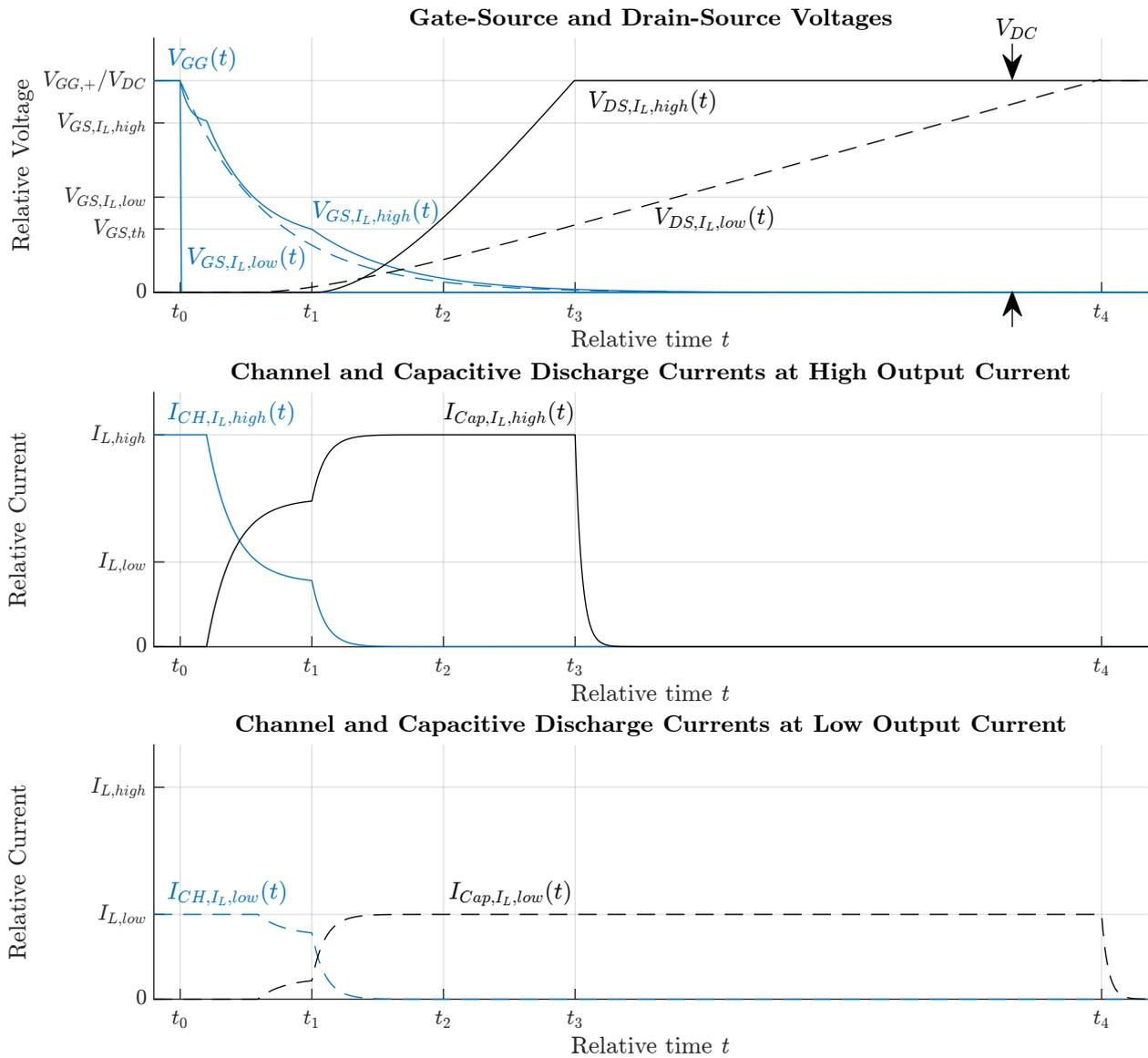
Figure 5.12: Switching transients during turn-off of HS MOSFET.
