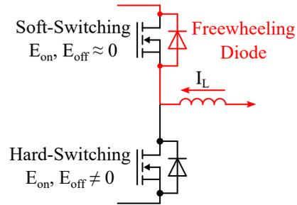
Figure 6.3: Impact of freewheeling on switching losses for negative output current.
