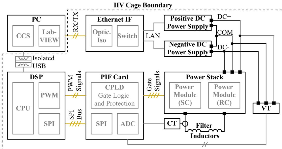
Figure 2.1: Schematic overview of the single phase setup.
