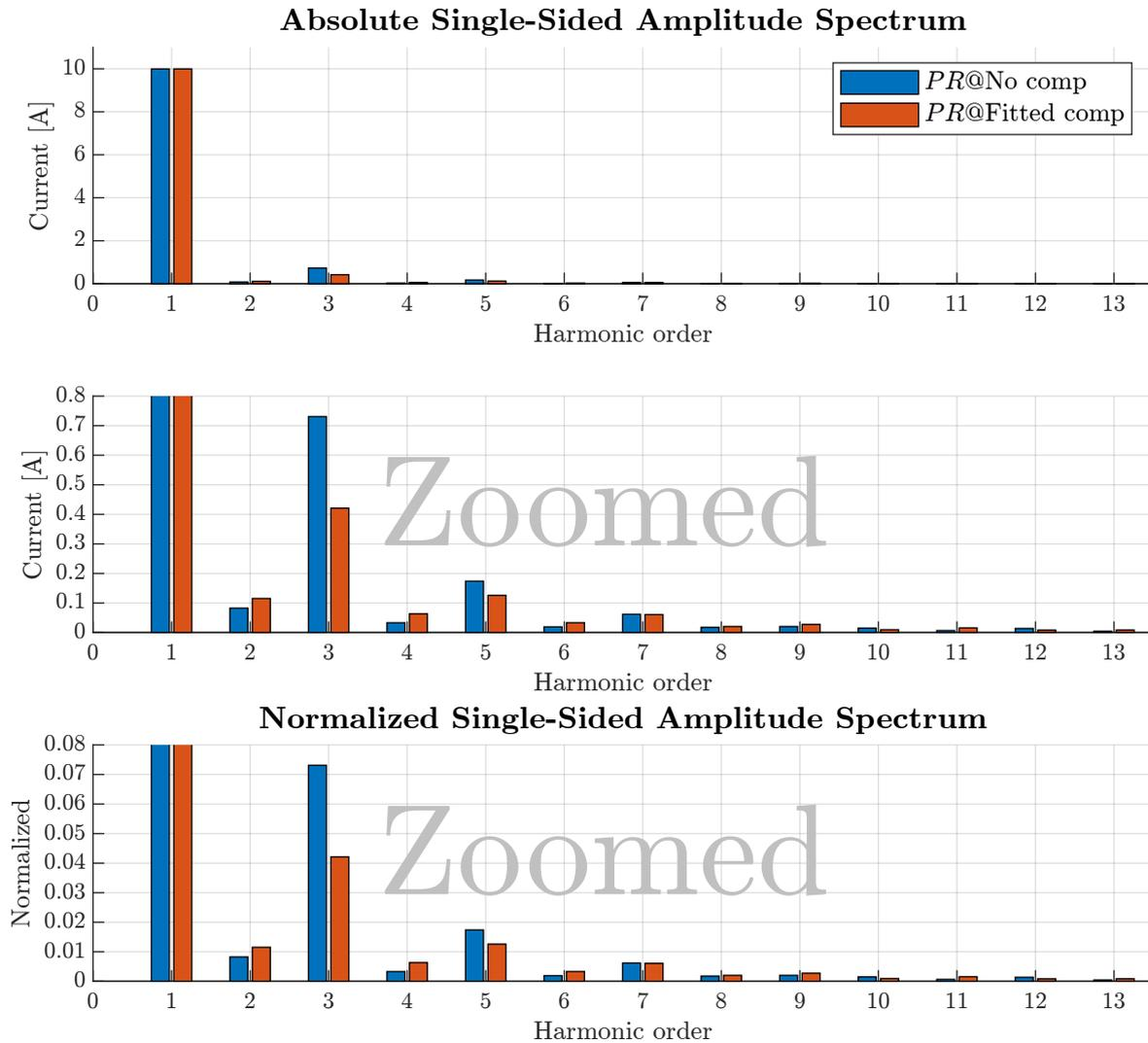
Figure 5.41: Absolute and normalized FFT analysis of PR controller performance at 6 kV.
