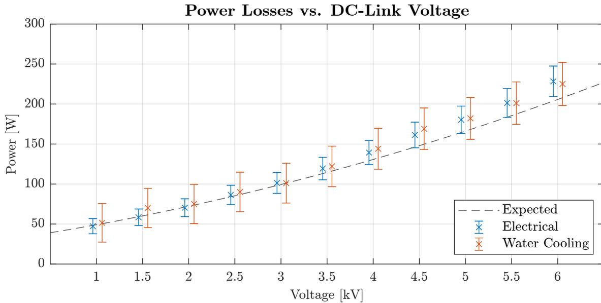
Figure 6.10: Estimated power losses at different DC-link voltages.
