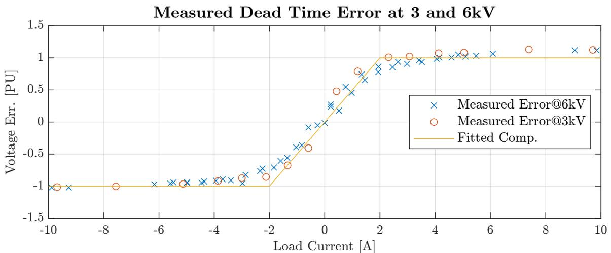
Figure 5.17: Normalized measured dead time voltage errors for 3 kV and 6 kV plotted along with the fitted compensation algorithm made at 3 kV.
