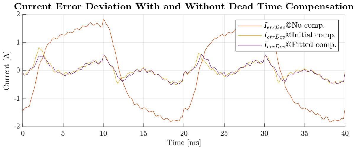
Figure 5.28: PI controller with compensation - Steady state response of sampled load current error deviation at 10 A reference.
