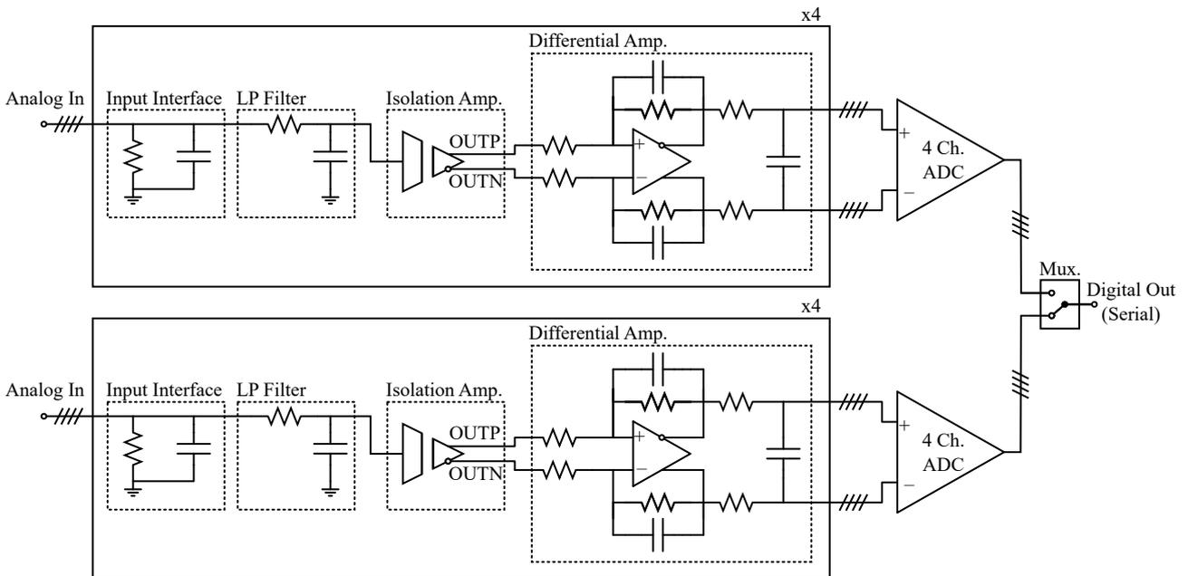
Figure B.1: Overall architecture of PIF card related to scaling and ADCs.
