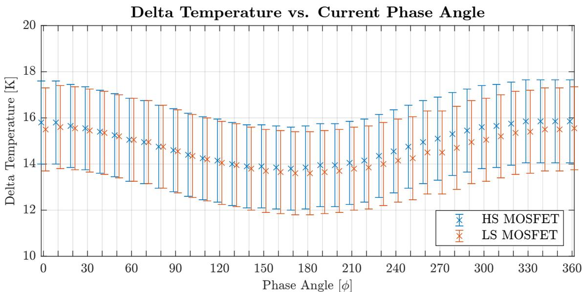
Figure 6.16: Delta die temperature for varying current phase angles.
