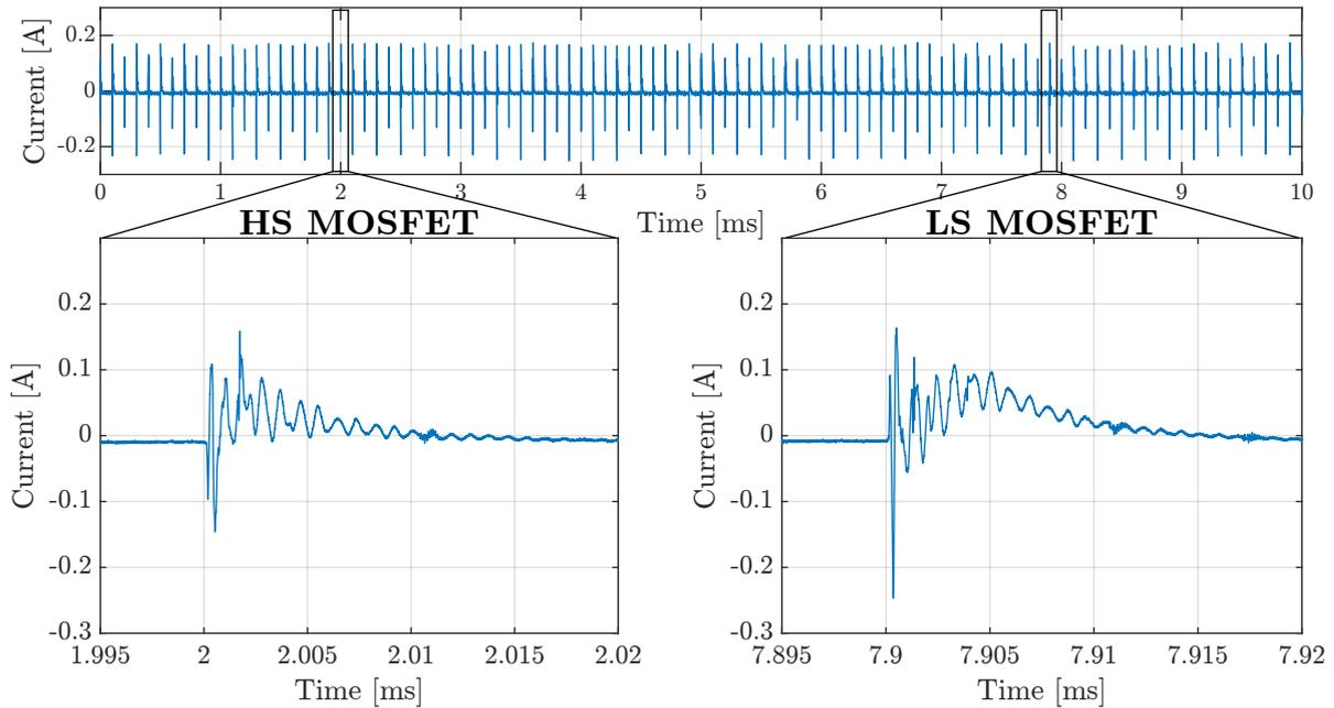
Figure 4.17: Measured common mode current in USB connection between DSP and USB isolator.
