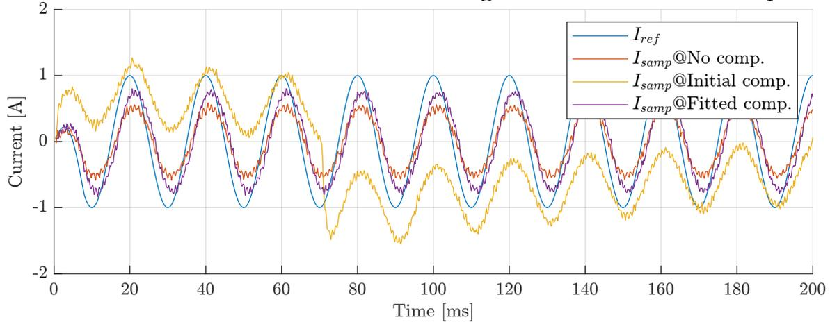
Figure 5.24: PI controller with compensation - Transient response of sampled load current at 1 A reference.
