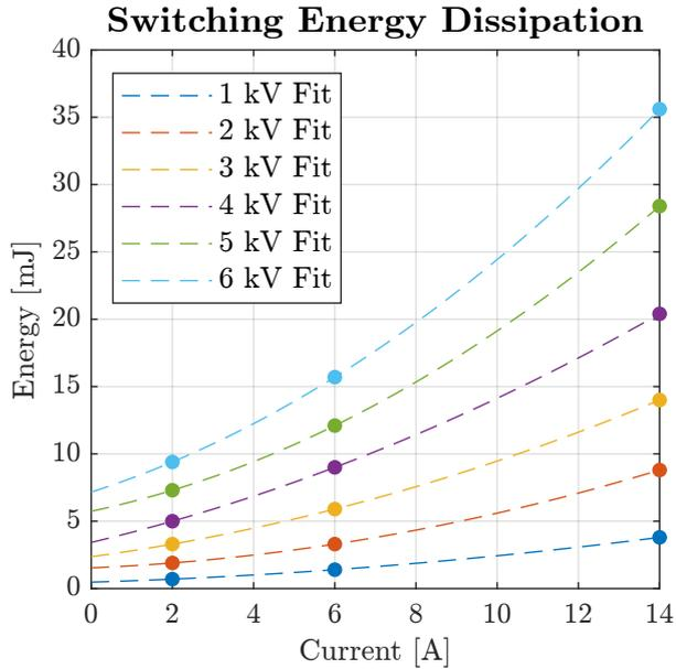
Figure 6.4: Turn-on and turn-off switching energy dissipation for varying load currents and DC-link voltages. *Source of data [3].*
