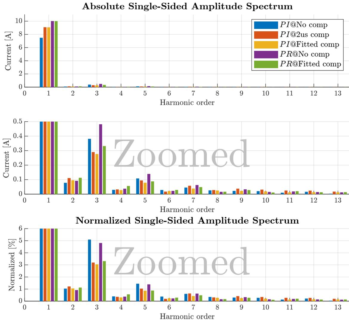
Figure 5.38: Absolute and normalized FFT analysis of PI and PR controller performance.
