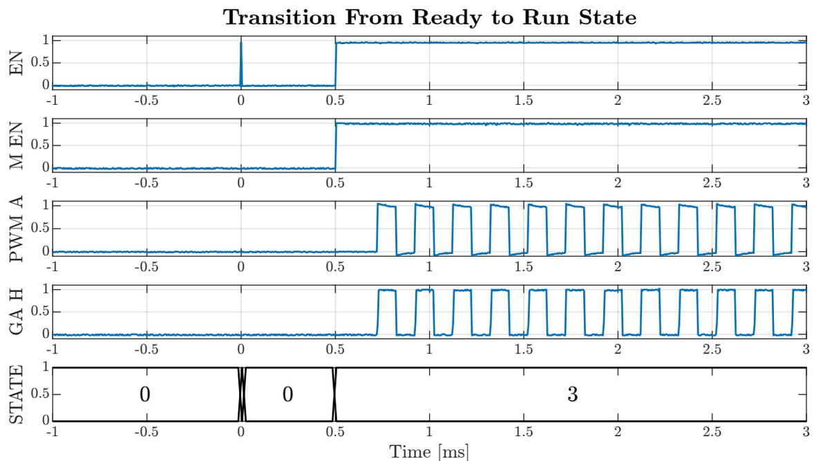
Figure 4.14: Measured transition from Ready to Run state on PIF card.
