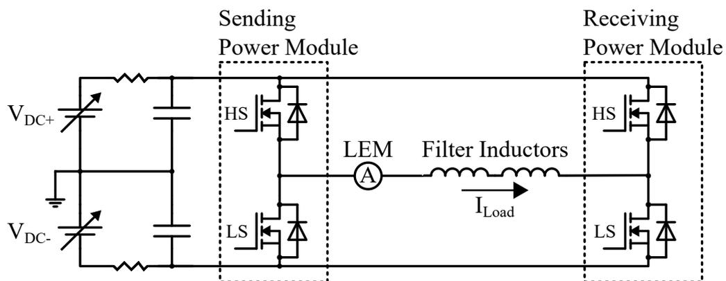
Figure 2.3: Electrical diagram of the single phase setup.
