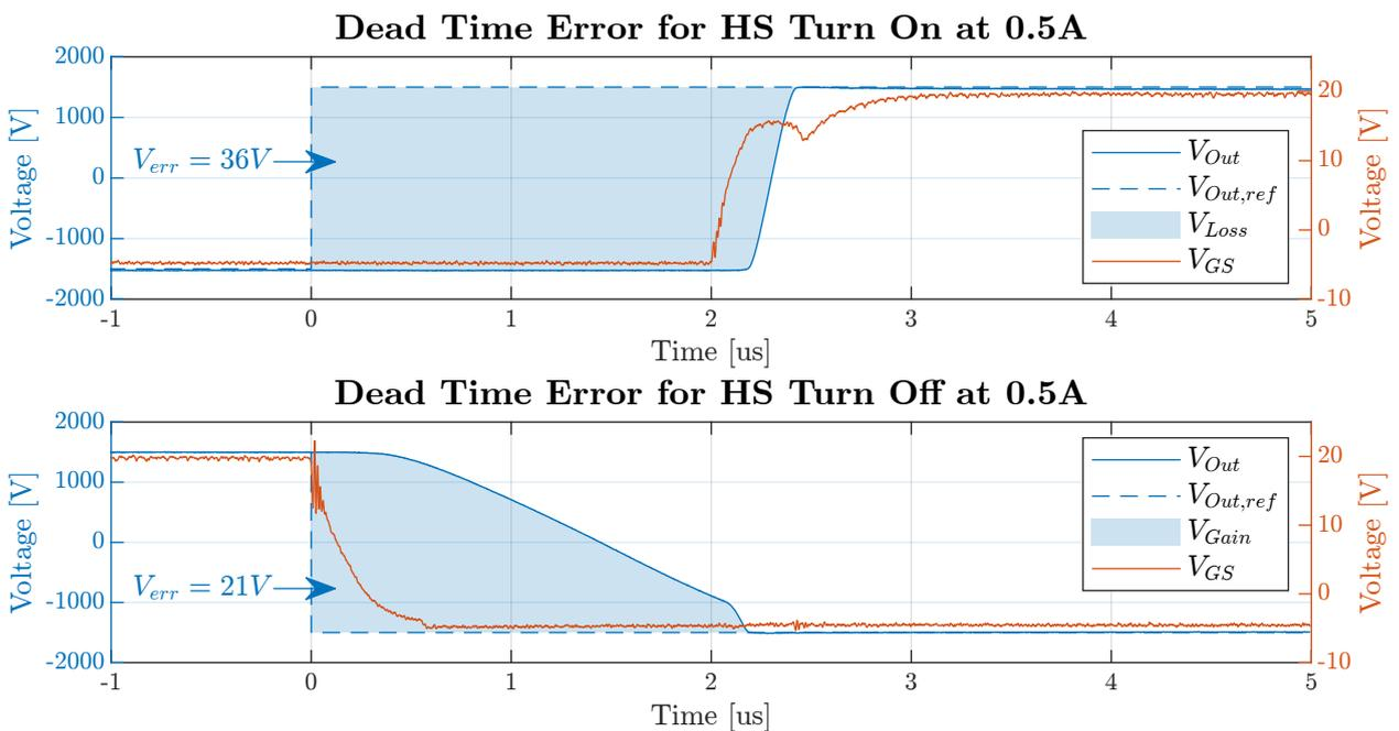
Figure 5.14: Measurement of dead time voltage error at positive 0.5 A load current.
