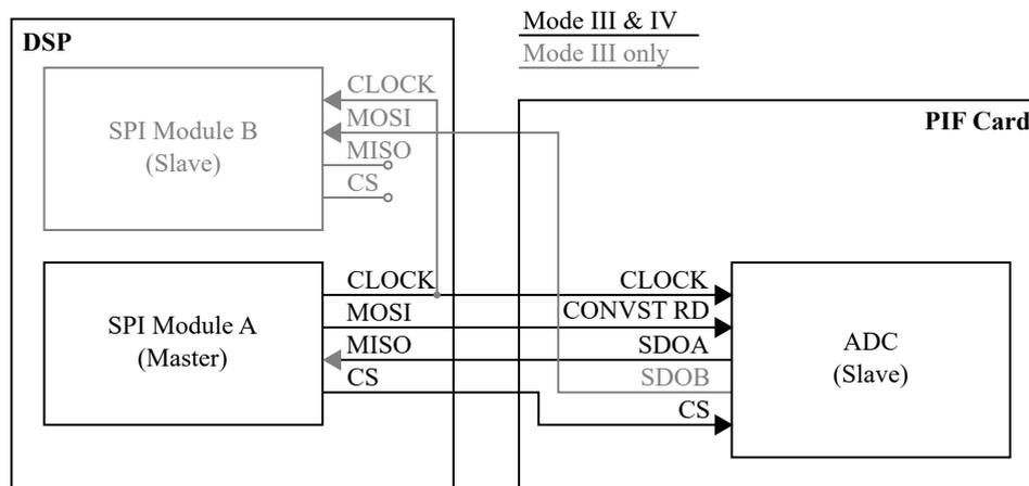
Figure 4.6: Hardware configuration to support SPI communication in mode *III* and *IV*.
