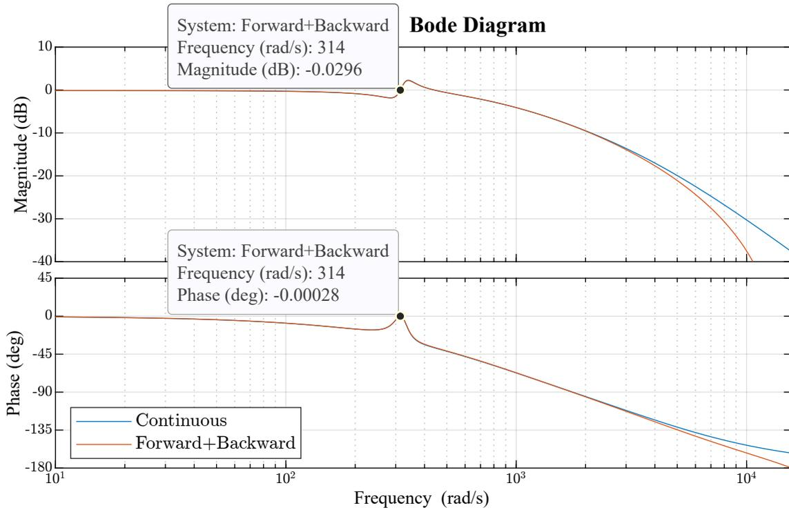
Figure 5.30: Bode plot of PR controller (314 rad/s = 50 Hz).
