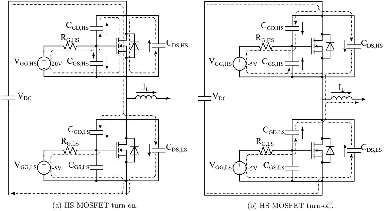
Figure 5.10: Charging and discharging of parasitic capacitances during switching transients.
