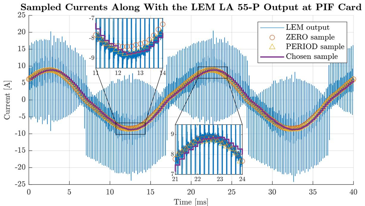
Figure 5.4: Sampled currents compared to the measurement output of LEM LA 55-P.
