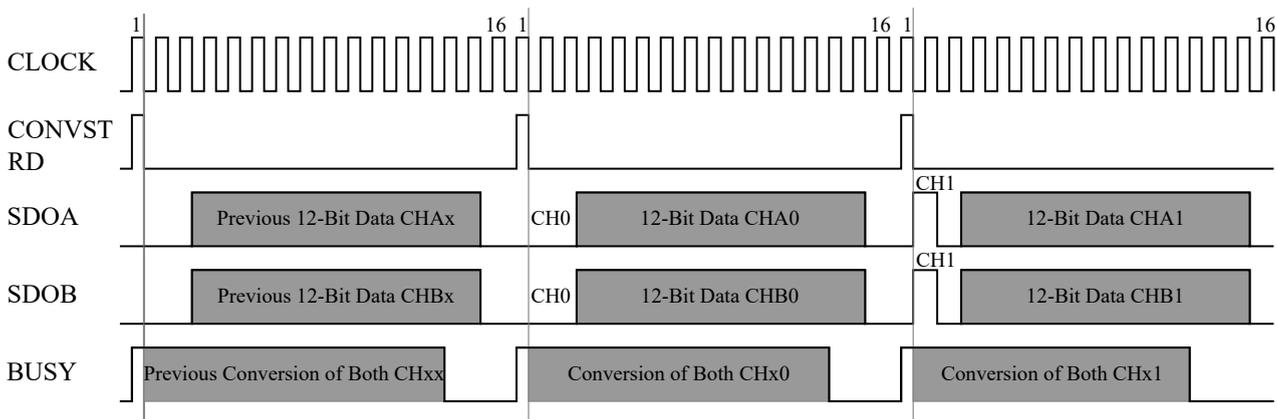
Figure 4.4: Timing diagram for mode *III*.
