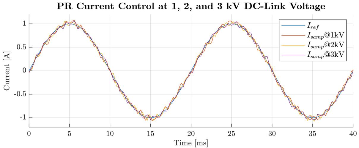
Figure 5.32: PR controller - Steady state response of sampled load current at 1 A reference.
