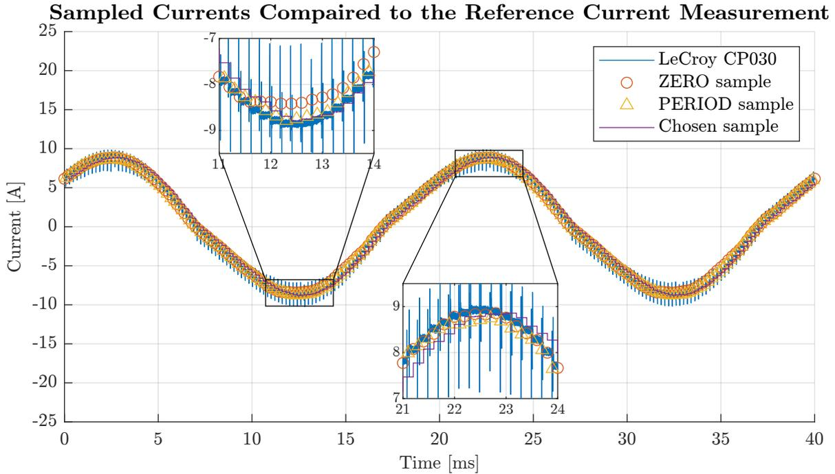
Figure 5.5: Sampled currents compared to the reference measurement made with LeCroy CP030.
