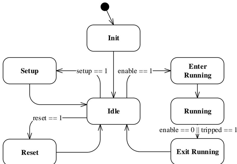
Figure A.1: Flowchart of the state machine running in *main()*.
