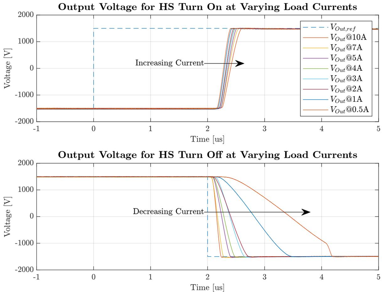
Figure 5.15: Change in output voltage transients for varying magnitudes of load current.
