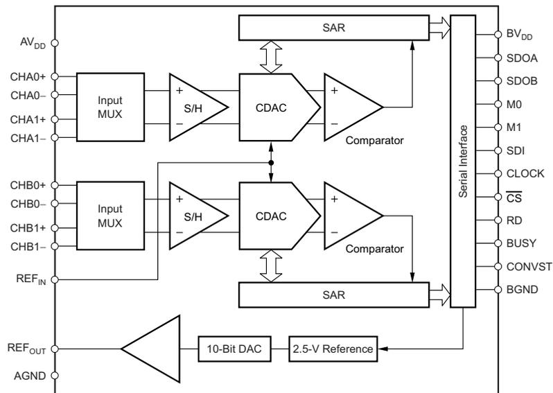
Figure 4.1: Functional diagram of the ADCs used on PIF card [39].
