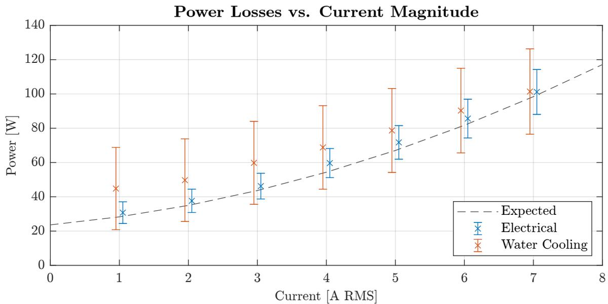
Figure 6.14: Power losses at different current magnitudes.
