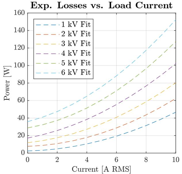
Figure 6.5: Expected power module losses (single module) for varying load currents and DC-link voltages at 5 kHz switching frequency.
