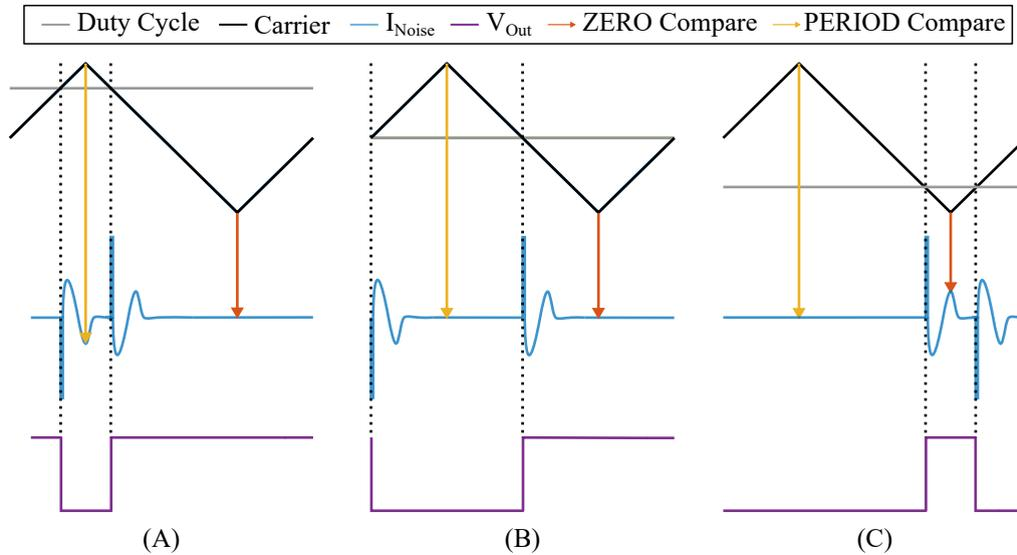
Figure 5.3: Illustration of sampling scheme at duty cycles of (A) 80%, (B) 50%, (C) 20% [1], [2].
