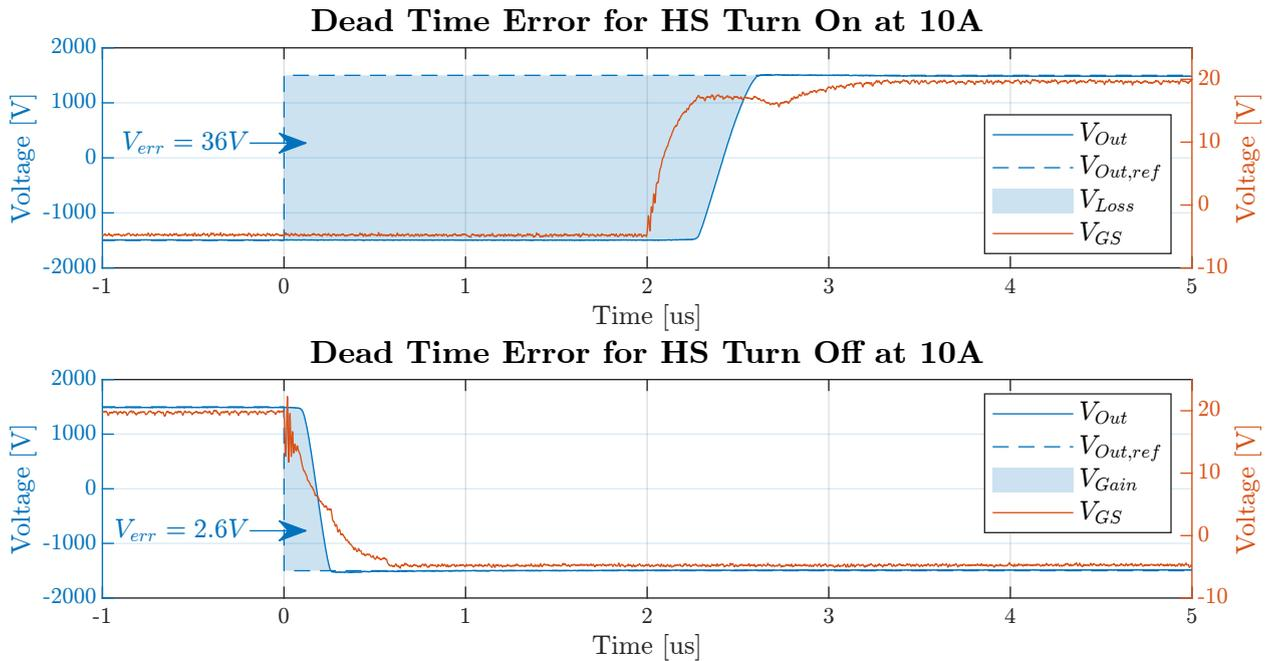
Figure 5.13: Measurement of dead time voltage error at positive 10 A load current.
