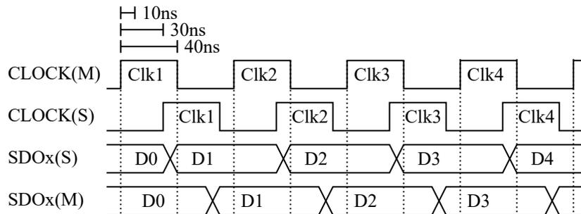
Figure 4.10: Timing diagram for SPI protocol at a bit rate of 12.5 MHz.
