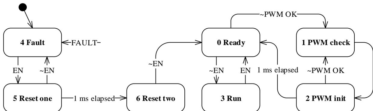
Figure 4.12: Overview of the state machine implemented on the PIF card.
