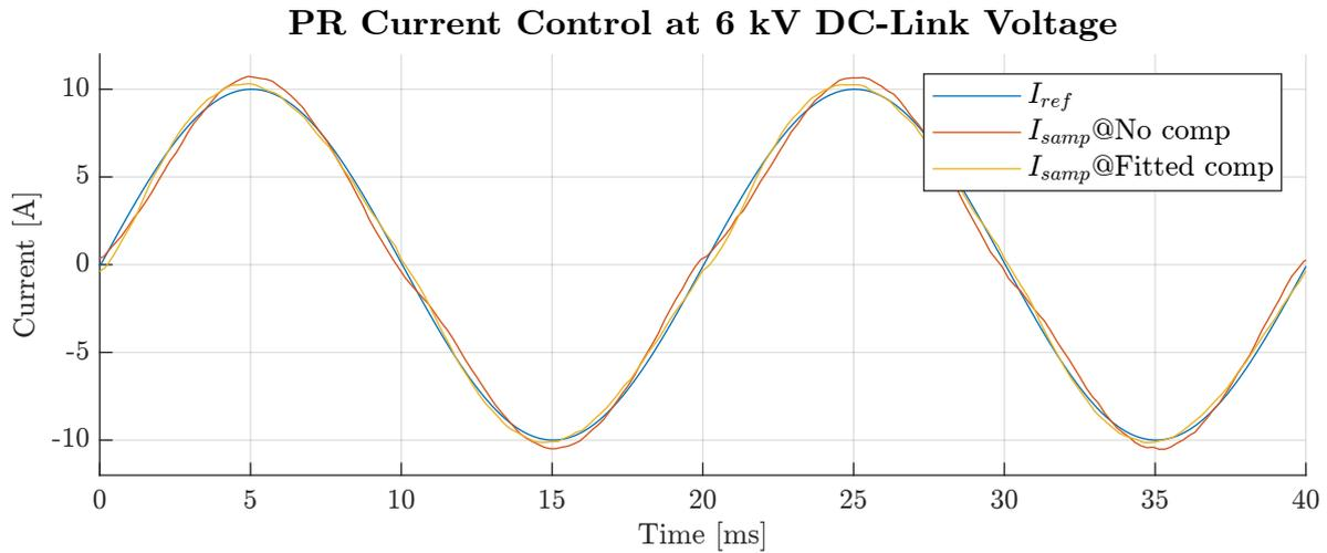
Figure 5.39: Rated operating point - Steady state response of sampled load current.
