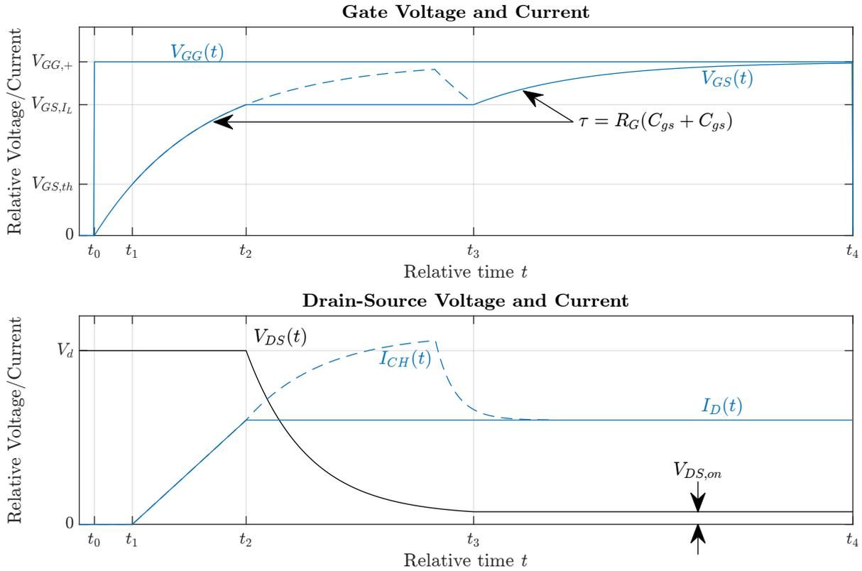
Figure 5.11: Switching transients during turn-on of HS MOSFET.
