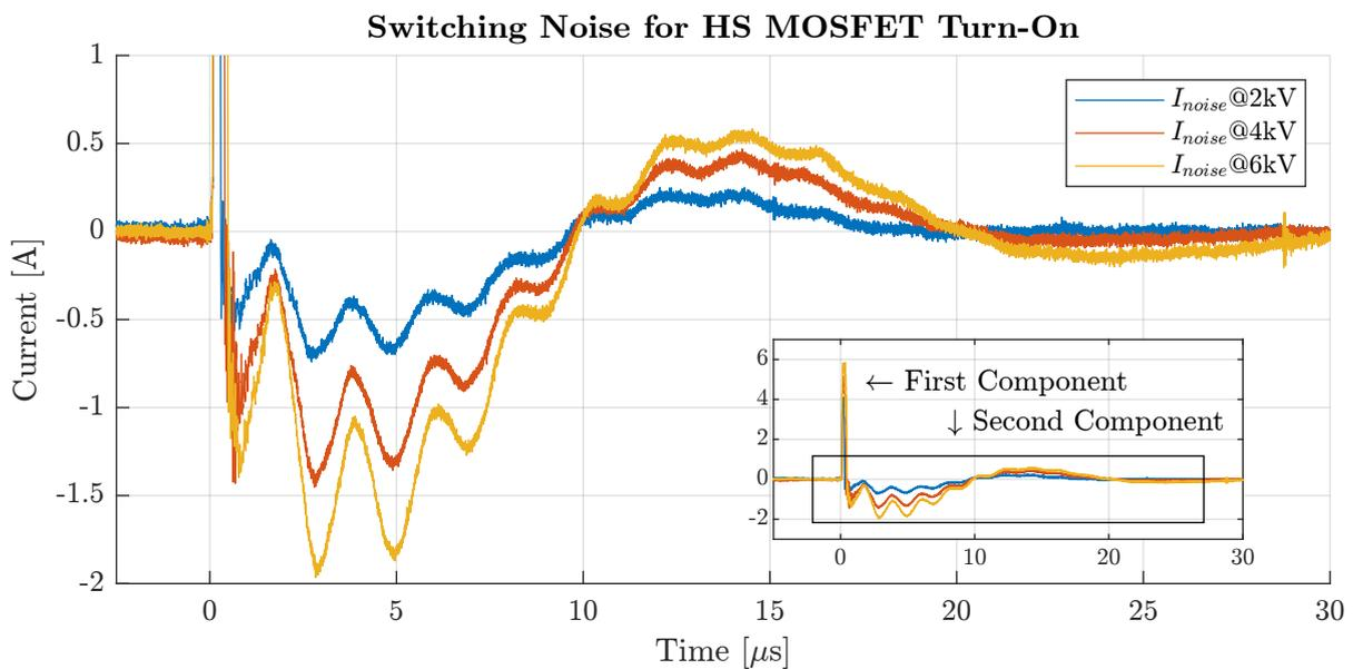
Figure 1.2: Measured switching noise currents for a turn-on switching event of the HS MOSFET [2].
