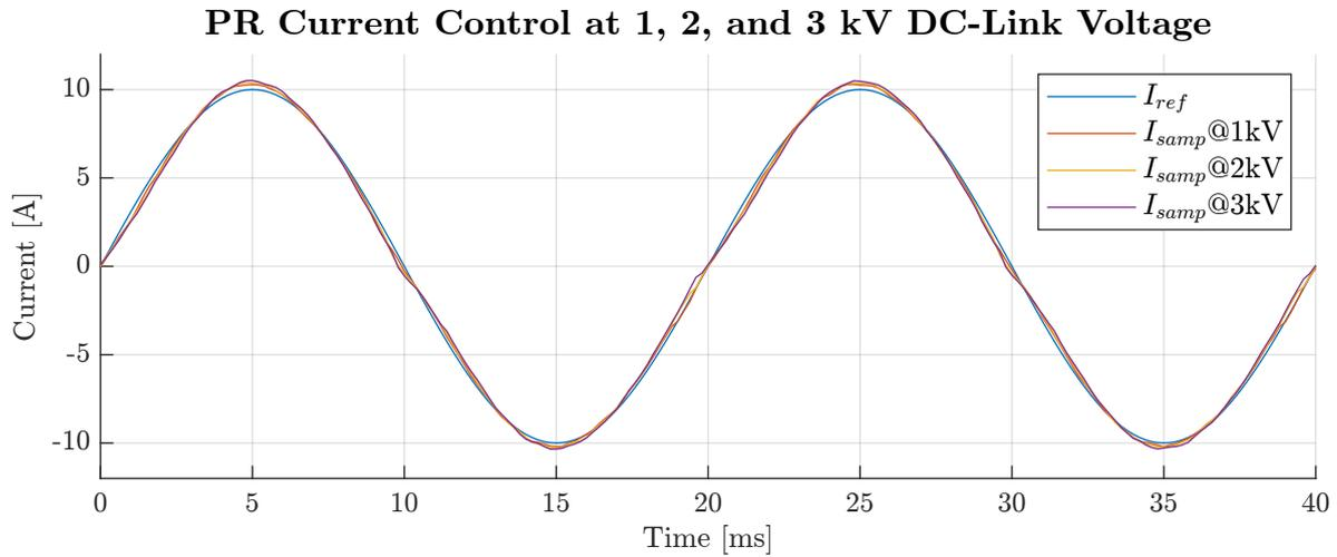
Figure 5.34: PR controller - Steady state response of sampled load current at 10 A reference.
