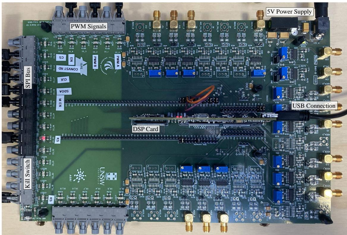
Figure 2.7: Photograph of the DSP interface board and DSP card.
