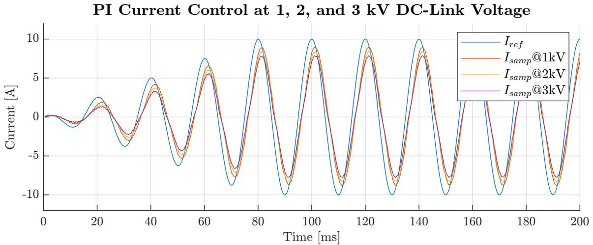
Figure 5.22: PI controller - Transient response of sampled load current at 10 A reference.
