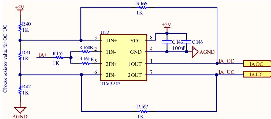
Figure B.4: Comparator circuitry for over- and undercurrent protection.
