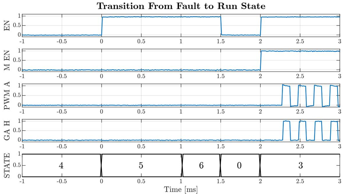
Figure 4.13: Measured transition from Fault to Run state on PIF card.
