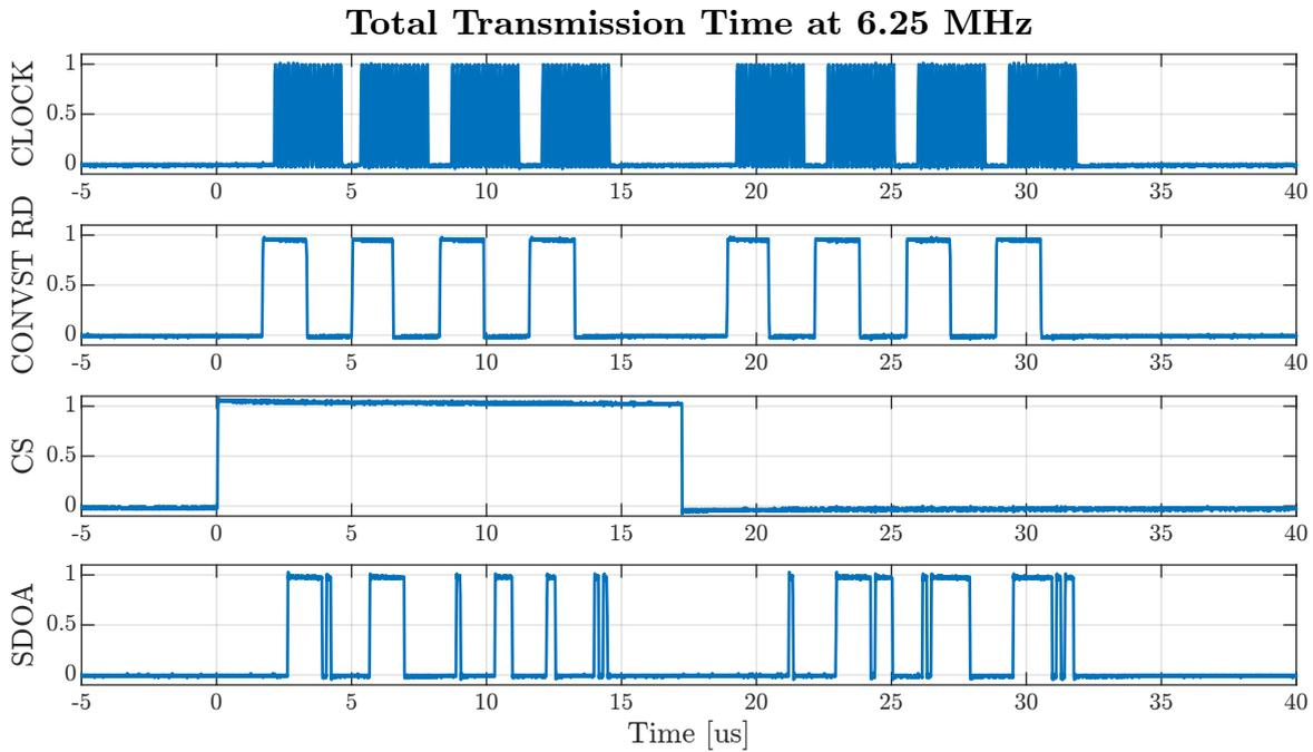
Figure 4.9: Measured total transmission time for all eight ADC channels at 6.25 MHz.
