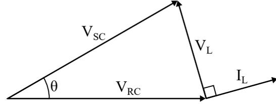
Figure 5.2: Open loop phasor diagram.
