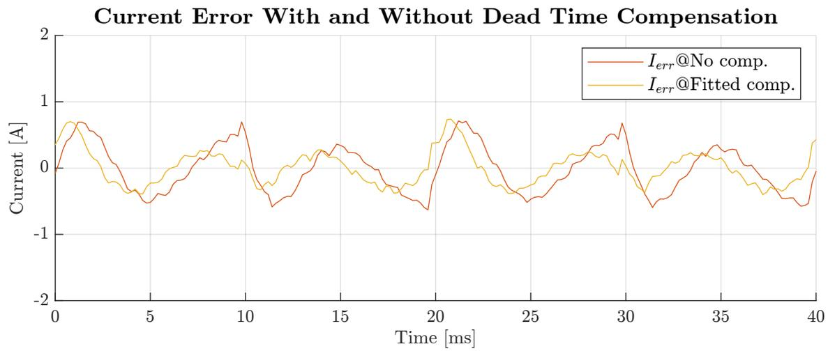
Figure 5.36: PR controller with compensation - Steady response of sampled load current error at 10 A reference.
