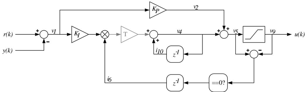
Figure A.3: Structure of the PI controller [52]. *Black: Structure from DCL, Grey: Correction.*
