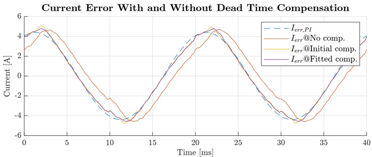
Figure 5.27: PI controller with compensation - Steady state response of sampled load current error at 10 A reference.
