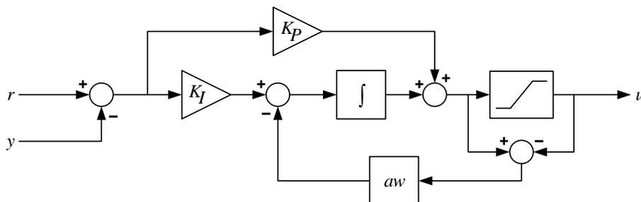
Figure 5.18: Structure of continuous PI current controller.
