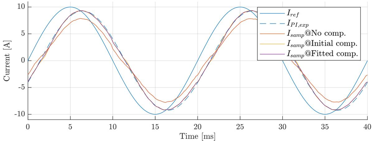
Figure 5.26: PI controller with compensation - Steady state response of sampled load current at 10 A reference.
