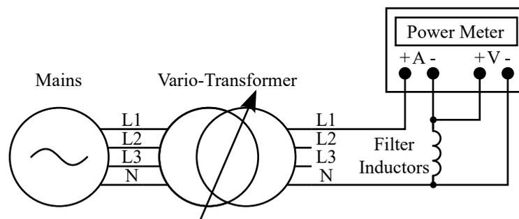
Figure 6.6: Schematic of the inductor loss test.
