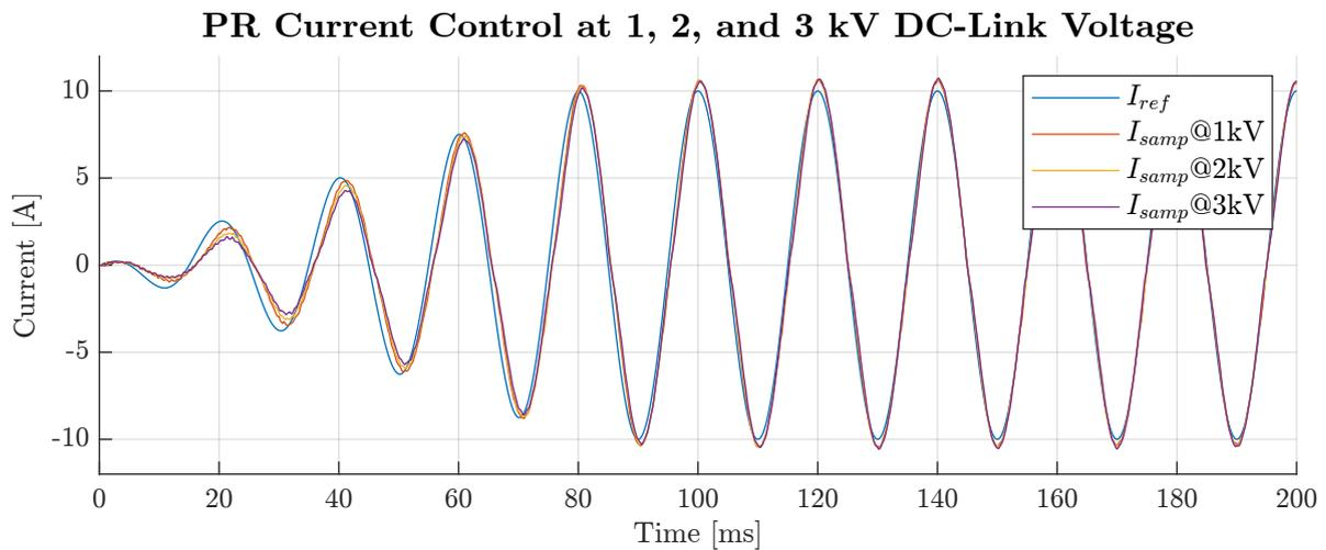
Figure 5.33: PR controller - Transient response of sampled load current at 10 A reference.
