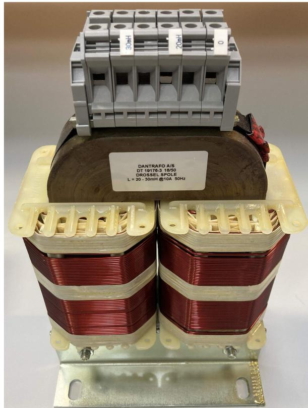
Figure 2.5: Photograph of a filter inductor.
