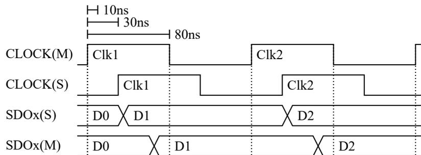
Figure 4.8: Timing diagram for SPI protocol at a bit rate of 6.25 MHz.
