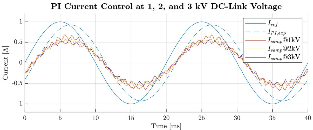
Figure 5.21: PI controller - Steady state response of sampled load current at 1 A reference.
