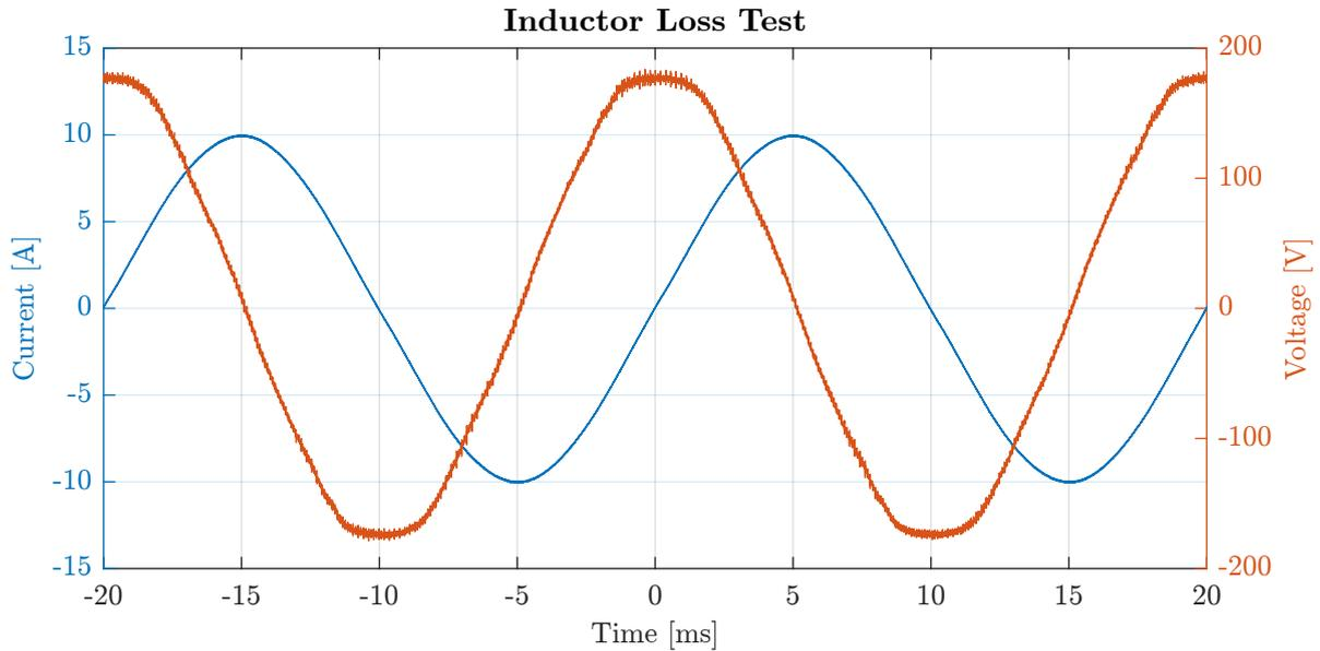
Figure 6.9: Measured current and voltage waveforms during inductor loss test.
