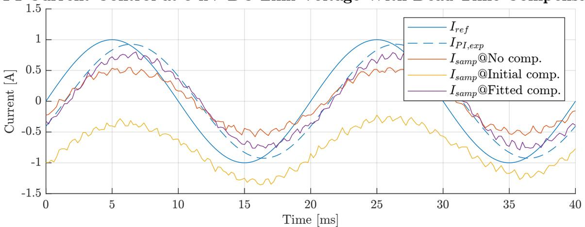
Figure 5.25: PI controller with compensation - Steady state response of sampled load current at 1 A reference.
