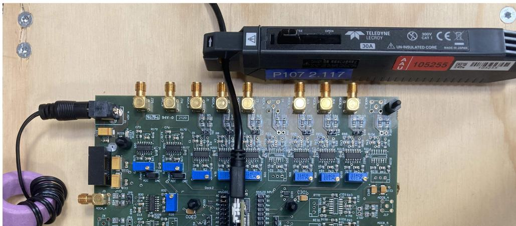
Figure 4.16: Photograph of a common mode current measurement in the USB cable.
