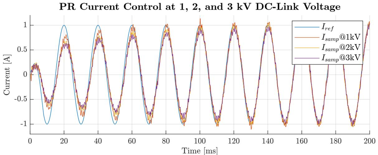
Figure 5.31: PR controller - Transient response of sampled load current at 1 A reference.
