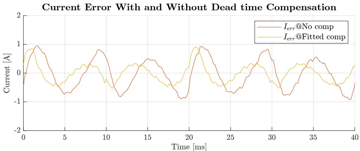
Figure 5.40: Rated operating point - Steady state response of sampled load current error.
