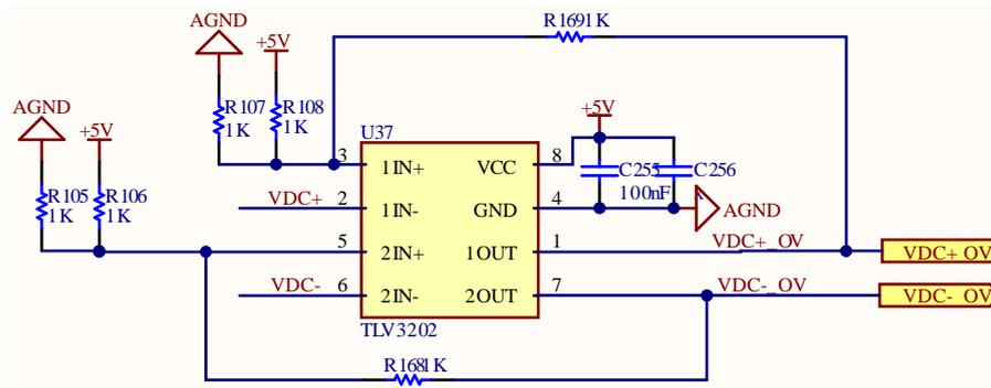
Figure B.5: Comparator circuitry for overvoltage protection.
