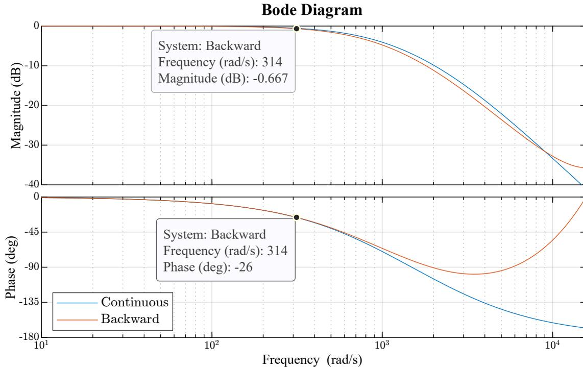
Figure 5.19: Bode plot of PI controller (314 rad/s = 50 Hz) [1].
