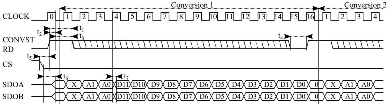
Figure 4.3: Detailed timing diagram of a conversion.
