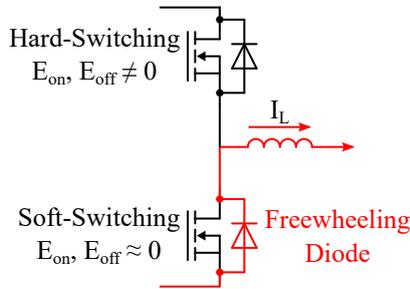
Figure 6.2: Impact of freewheeling on switching losses for positive output current.
