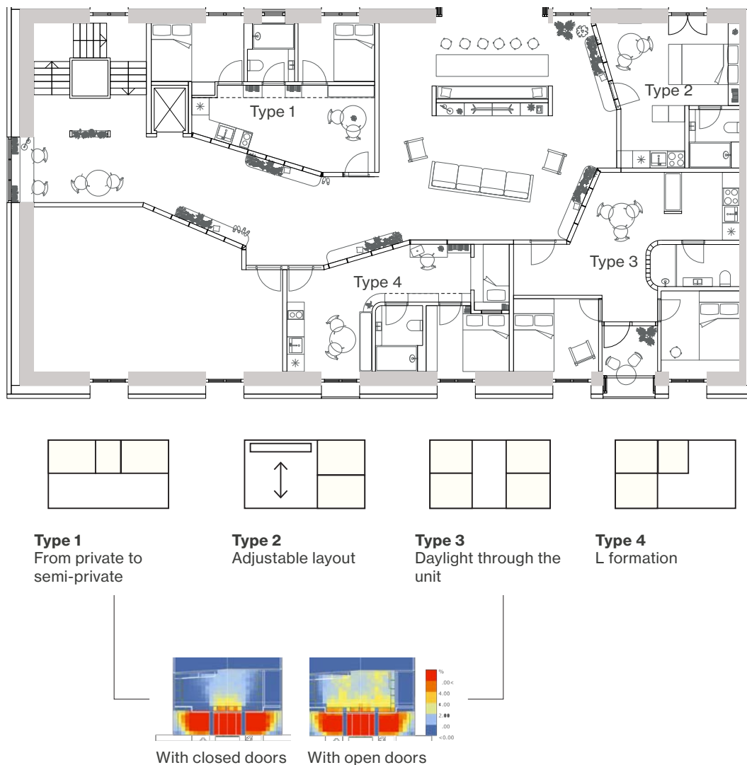
126. Types of housing unit concept, with simulated daylight
