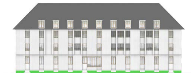
165. Exterior re-insulation using concrete on the southern and northern facades.
