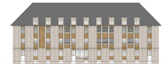
164. Exterior re-insulation using new bricks and wood on the southern and northern facades.
