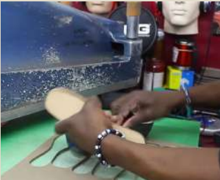
52 All soles are stamped w. A sole puncher
