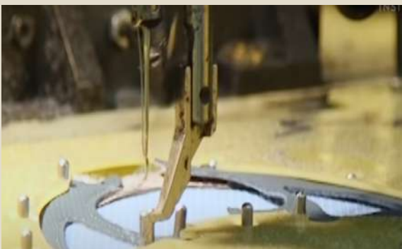
Flat stitching by machine is done on a template. Flat stitching is used because it does not create any overlapping threads and creates a durable connection.
