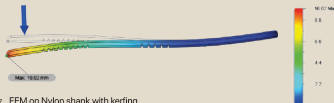
137 FEM on Nylon shank with kerfing
