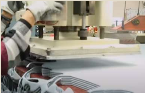
The cutting machine presses the template knife through the material, cutting out fabric and foam patterns.
