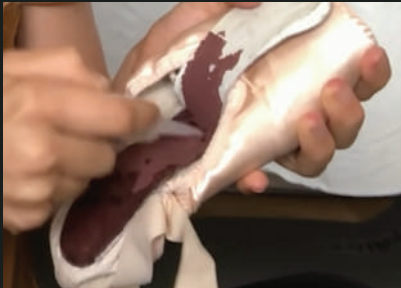
08 - glues platform, box & shank where it needs to be stiff and hard - requires glue
