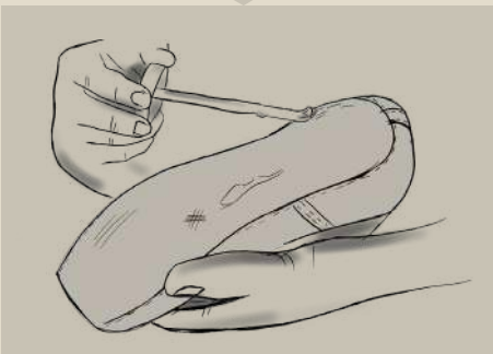
Glue is applied to the fabric lining and prepped for assembly with outer sock.
