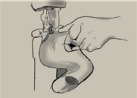
To secure all parts the final shoe is sewn together at the seam lines. Name and other details are added.
