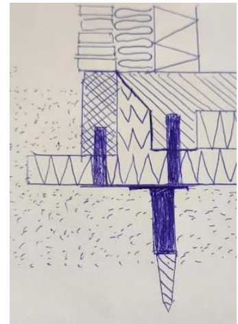
Figure 27 Screw pile foundation detail. U-plate and M24 bolts (hand-sketch)
