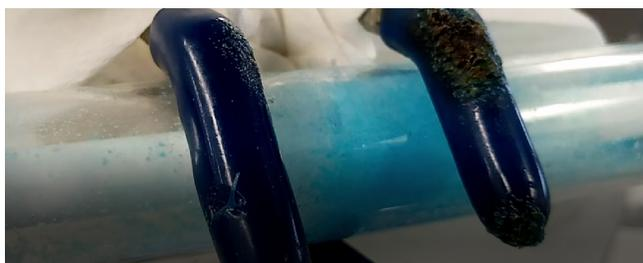
Figure 3: Percrystallisation experiment with Copper sulfate.
