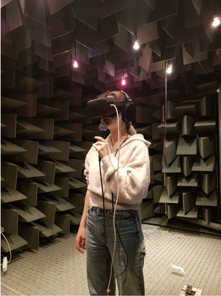
Fig. 2.6: Participant with the complete hardware setup (circum-aural open back headphones, VR HMD, microphone)
