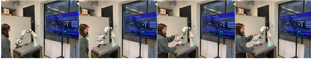
Figure 4.5: Sequence of interaction with the system. From left to right: User gives the voice command to Max; the robot starts the grasping of the top cover; user pushes the gripper; the robot releases the component.
