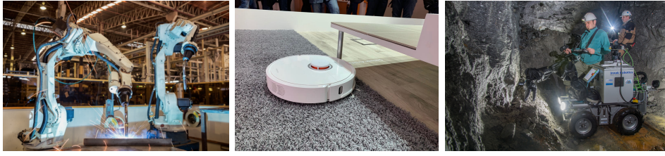
Figure 2.2: Example of a robot for each robotics category. Left: Industrial robot - Two industrial robotic arms performing soldering [Nichols, 2020]; Middle: Personal Service robot - Vacuum and moping robot [Brains, 2020]; Right: Professional Service robot - Mine robot assisting in mining [Baggaley, 2017].
