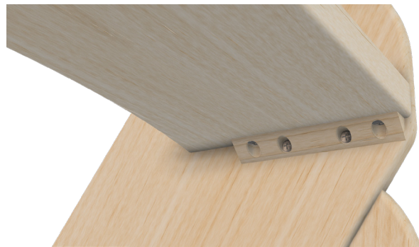
[III. 5.8]: Step connector with 4 screws
