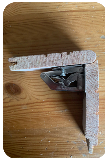
[III. 4.30]: Second spring hinge mockup in cardboard and wood
