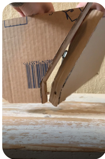
[III. 4.30]: Second spring hinge mockup in cardboard and wood
