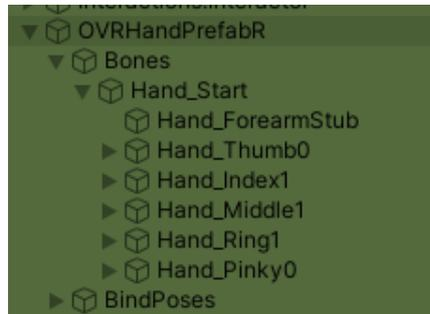
FIGURE 4.6: Hierarchy of the bones in an OVRHandPrefab for the right hand.
