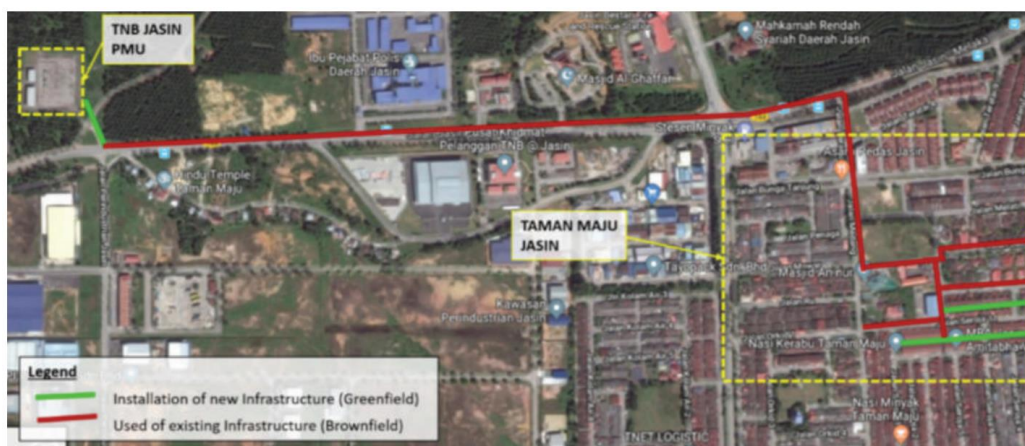
Figure 4.6: Combination of existing and new infrastructure during the pilot project (MCMC, 2018)
