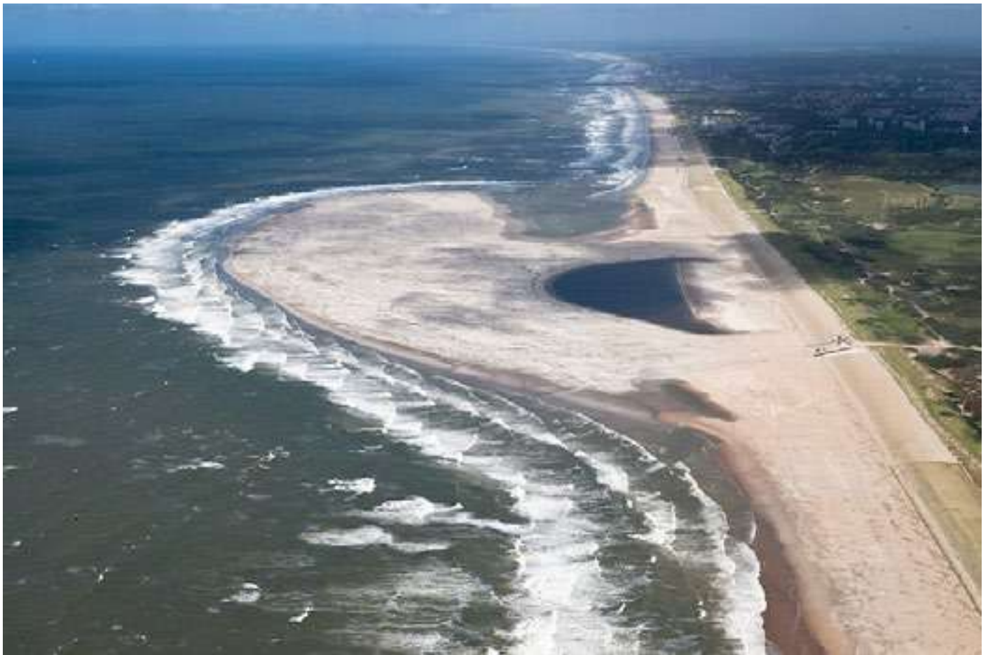
Ill. 18 The Sand Motor in Ter Heijde, Holland is an experiment to defend the coastline from flooding. Huge amounts of sand are placed at the southern part of the coast, and the nature spreads the sand along the coast, which extends the foreland and creates barrier against flooding (Resilient The Hague n.d.)
