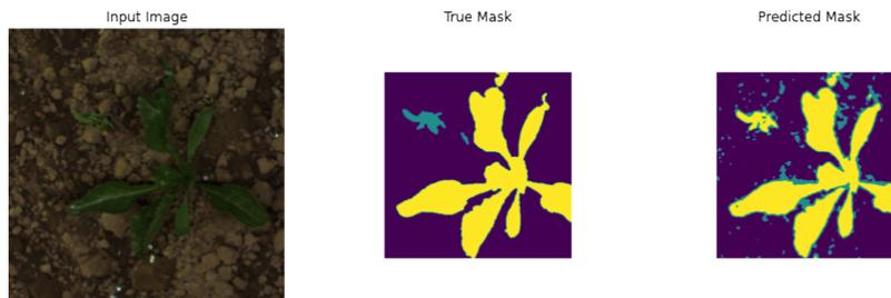
**Figure 4.5:** Prediction with model trained on mixed data-set with 10% from the real data-set
