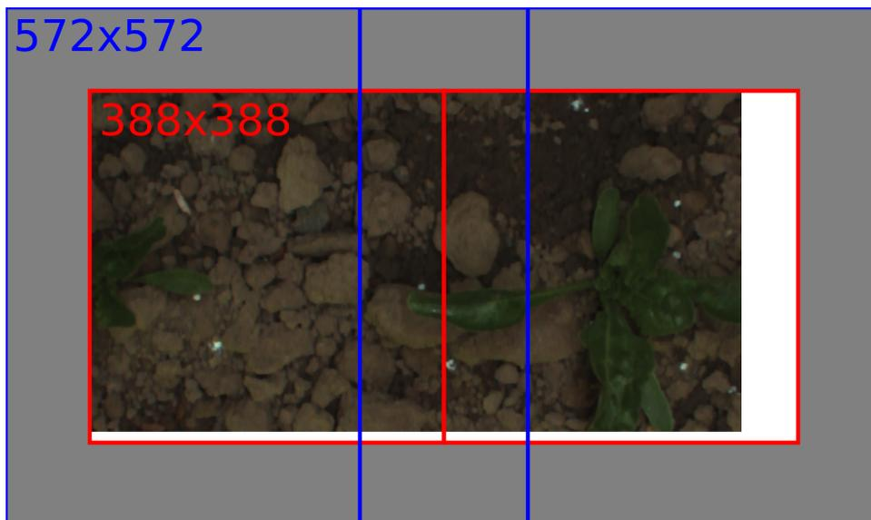
**Figure 3.24:** Example of calculating padding to tile an image. The white area is the padding required to have an integer amount of tiles. Grey area is the padding required to account for the discrepancy in input and output size. The image is tiled in step sizes of 388, producing overlapping input tiles of 572x572 (blue) and tiled output tiles of 388x388 (red)
