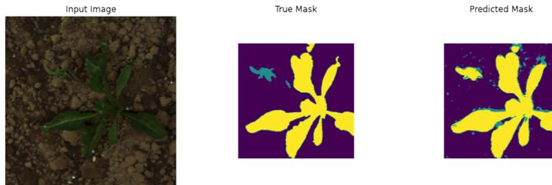
**Figure 4.4:** With just 10% of the dataset being from dataset 1 already shows poor weed prediction
