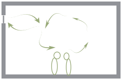
Ill 96.2 Mixing ventilation. Tempered air is supplied, mixed with the existing and exhausted. Good in low ceiling rooms with low activity.
