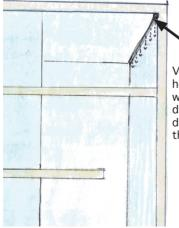
View to slim water hose at the top level, where water is running discretely and steady down the facade to the ground floor.
