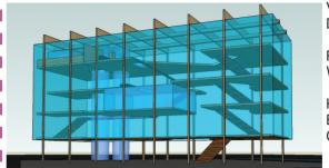
Version 4 Distance: 5m Frames: 8 Width: 185mm Height Beam: 1300mm Column: 233mm
