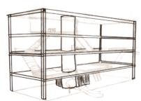
The sketch is supposed to show the core as the holding structure.
