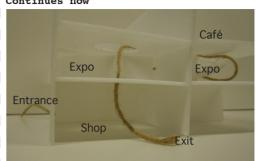
The flow in this pavilion is continues and going through the different showrooms, but in this model it is spread out on double size floor plan compared to the other strategies. A mix between this flow on a floor plan as the size of the others could be interesting to work further with.
