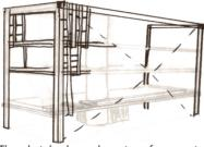
The sketch shows how two frames stabilized by diagonal cables are the holding elements. The platforms are hanging down from the frames.
