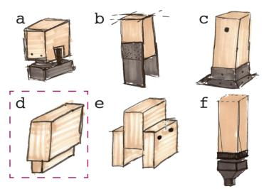
On some of the sketches the joints are done with metal and on others only wood. However, the expression of the joints must be Danish and Nordic. As mentioned earlier, it should be simple. Therefore a solution with fewer different materials will be chosen, the joints where only wood is visible, as in solution 4 of the section and plan is chosen.
