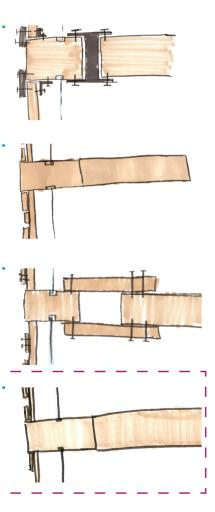
The connection to the ground. Different ideas both with metal, concrete and only wood are being sketched on. a) Connected to concrete element coming up from the ground. b) Steel fixed. c) Steel fitting. d) Connected to a concrete slab underneath. e) Wood connected directly to the ground. f) Steel fitting.
