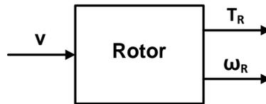
Figure 4.5 Block diagram of the rotor
