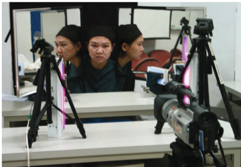
Figure 15: One camera catches three perspectives of the actor's face via the use of mirrors. Picture taken from [12].
