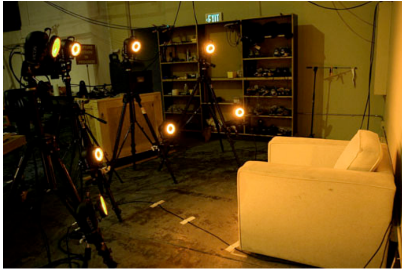
Figure 14: Multi camera optical motion capture setup. Picture taken from [33].
