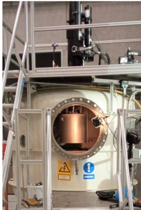
**Figure A.4:** Tank with piston installed at the top and Bucket B attached to the piston inside.
