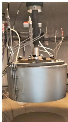
**Figure A.2:** Bucket B with PP sensors attached to the piston.
