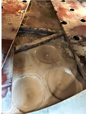
**Figure A.13:** Sand surface disturbed after second loosening approach: applying water pressure with a hose.
