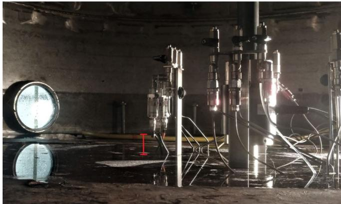
**Figure A.28:** Water raised to a secure distance before the sensor's cable connection. Distance in between sensor and water is drawn as a red line.
