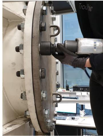
**Figure A.27:** Tightening of lid's bolts with pneumatic torque wrench to seal the tank.
