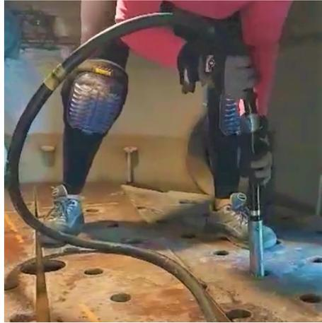
**Figure A.14:** Vibration of soil inside pressure tank.
