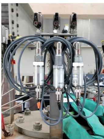
**Figure A.3:** PP sensors attached to Bucket A.
