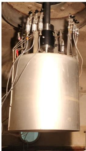
**Figure A.1:** Bucket A with PP sensors attached to the piston.
