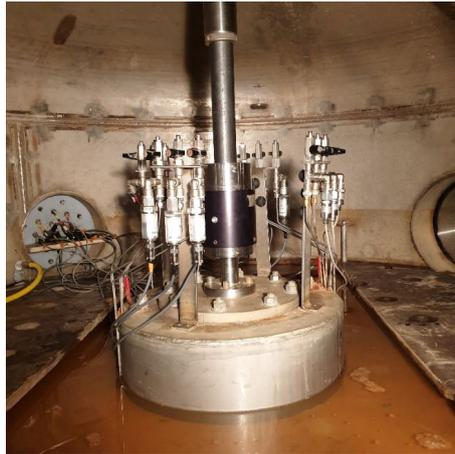
**Figure A.22:** Bucket A after first part of installation (one piston extension used).
