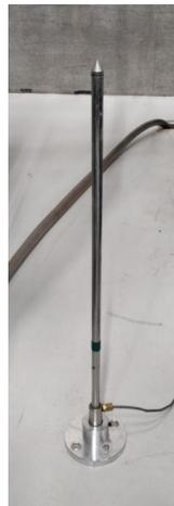
**Figure A.11:** Mini-CPT cone penetrometer.
