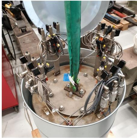
**Figure A.20:** Bucket foundation model submerged in barrel filled with water for saturation of PP sensors' system.
